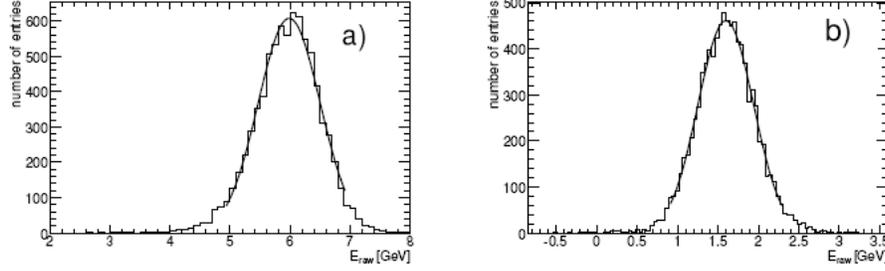
Figure 6.11: a) :  $E_{raw}$  distribution for a sample of 7 GeV electron at beam  $\eta=0.35$ . The curve corresponds to a Gaussian fit performed to determine  $E_e$  and  $\sigma_e$ . b) : Monte Carlo distribution for a sample of 1.8 GeV muons produced in the decays of beam pions at  $\eta=0.35$ .
