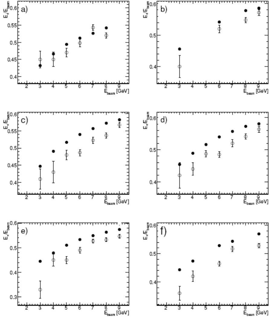
Figure 6.13: Energy response ratio measured (open points) and predicted by Monte Carlo simulation (full points) as a function of  $E_{beam}$  for different  $\eta_{beam}$  values: a) 0.20, b) 0.25, c) 0.35, d) 0.45, e) 0.55, and f) 0.65. The error includes statistical and systematic effects combined in quadrature.
