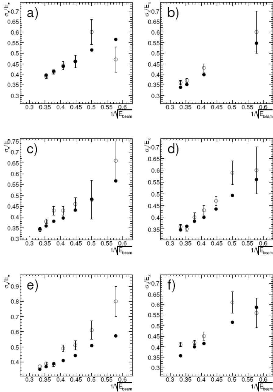
Figure 6.14: Fractional resolutions measured (open circles) and predicted by the Monte Carlo simulation (full points) as a function of  $1/\sqrt{E_{beam}}$  for different values of beam : a) 0.20, b) 0.25, c) 0.35, d) 0.45, e) 0.55, and f) 0.65. The errors include statistical and systematic effects.
