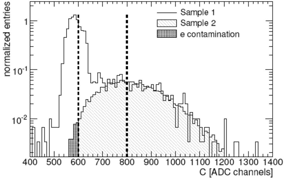
Figure 6.8: Distributions of the Cerenkov signal C for sample 1 (pions and electrons) and sample 2 (only electrons) in the case of a 9 GeV beam. The Cerenkov cuts  $C=600$  ADC (pion selection cut) and  $C=800$  ADC (electron selection cut) are indicated by the dashed lines. The dark region corresponds to the extrapolated electron contamination in the pion sample.
