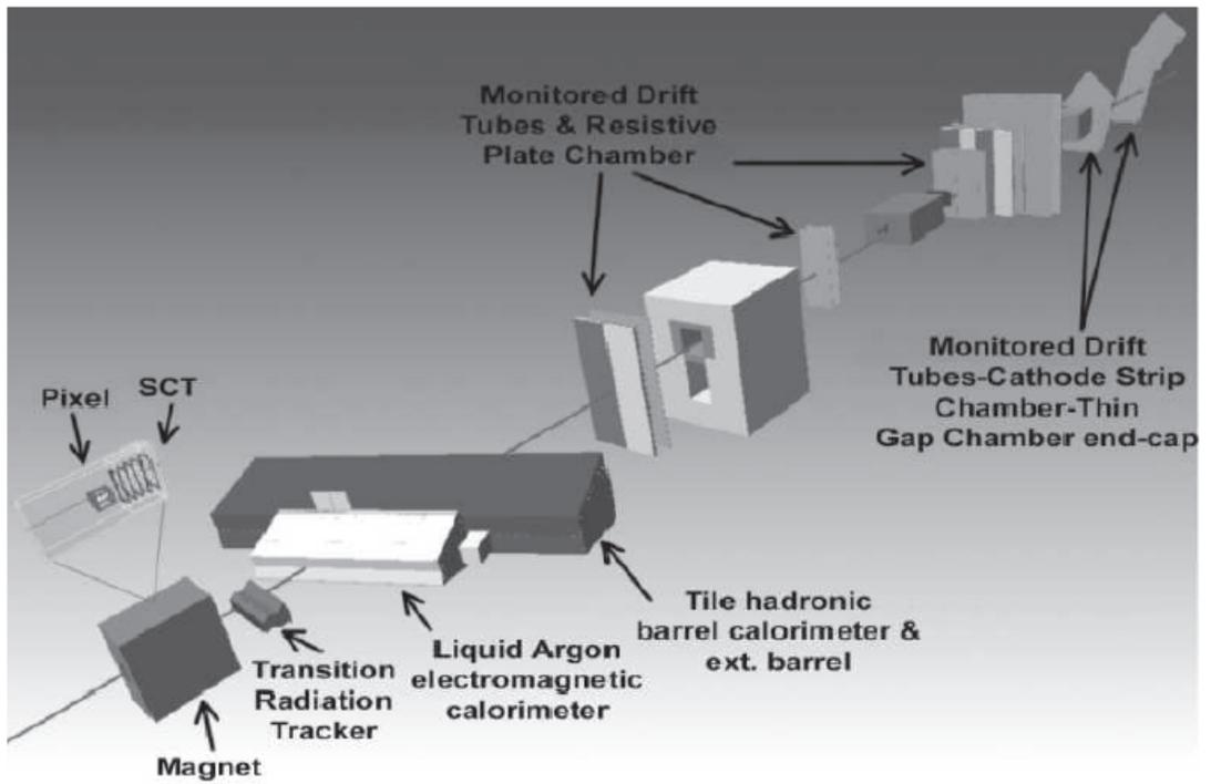
Figure 5.3: ATLAS subdetectors installed for in 2004 test beam.
