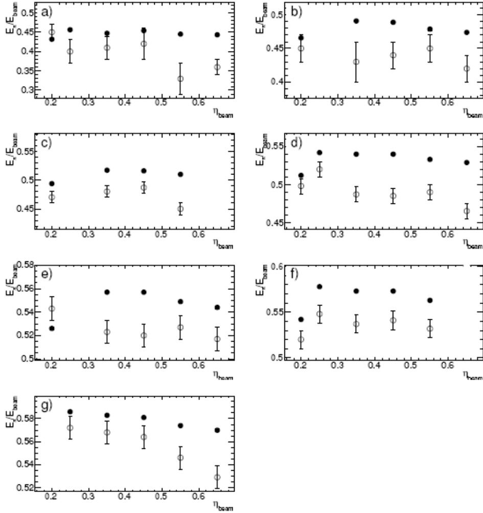
Figure 6.12: Energy response ratios measured (open points) and predicted by Monte Carlo simulation (full points) as a function of  $\eta_{beam}$  for different beam energy values: a) 3 GeV, b) 4 GeV, c) 5 GeV, d) 6 GeV, e) 7 GeV, f) 8 GeV and g) 9 GeV. The error includes statistical and systematic effects combined in quadrature.
