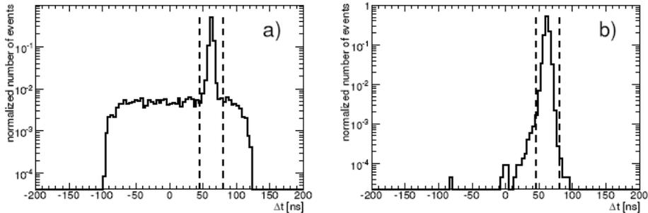
Figure 6.5: Distributions of  $\Delta t = t_{pulse} - t_{trigger}$  for TileCal cells with a signal larger than 75 MeV a) for a 9 GeV pion beam, b) for a 100 GeV pion beam where no out-of-time particles are expected. The region selected in the analysis is shown.
