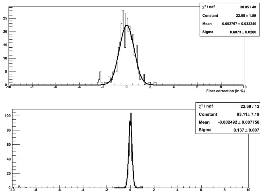
Figure 4.15: Spread of  $\Delta_{fiber}^{\frac{n}{n+1}}$ . In the top plot is shown the result of the measure before the application of the diffuser. In the bottom plot the same result but after the application of the diffuser. We can see that there is a gain of factor four from the precedent measure.
