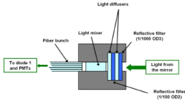
Figure 4.3: The light mixing block in the LASER box
