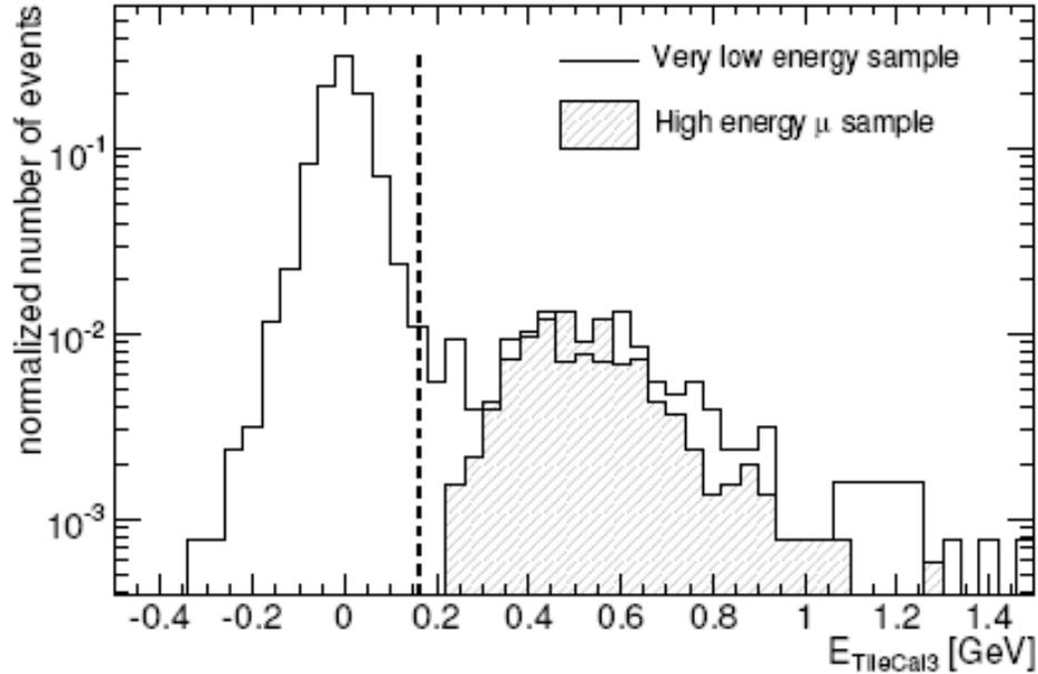
Figure 6.6: Distribution of the energy deposited in the 3rd sample of TileCal, ETileCal3. The empty distribution corresponds to a 7 GeV  $\eta_{beam}=0.2$  pion beam with high-energy muon contamination. The hatched distribution corresponds to a 20 GeV muon beam at  $\eta_{beam}=0$ . Events with ETileCal3 <160 MeV were selected in the analysis.
