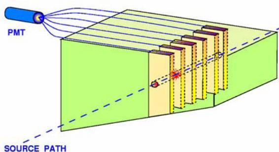
Figure 3.8: Mechanical concept of Cesium calibration system
