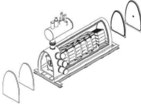
Figure 5.10: LAr view put inside the cryostat.
