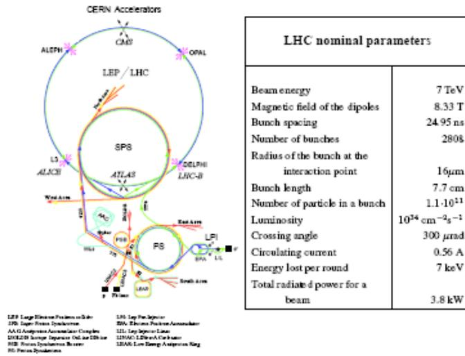
Figure 2.2: The LHC accelerator system and his nominal parameters.
