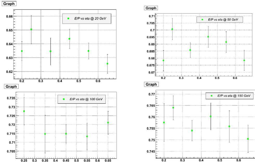
Figure 5.18: Evolution of the fractional response to hadrons as a function of eta, for different values of the beam energy.
