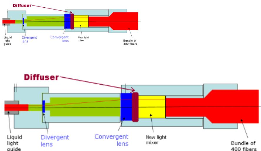
Figure 4.19: Modification in the Coimbra box. On the top before the change, on the bottom after the insertion of the diffuser.
