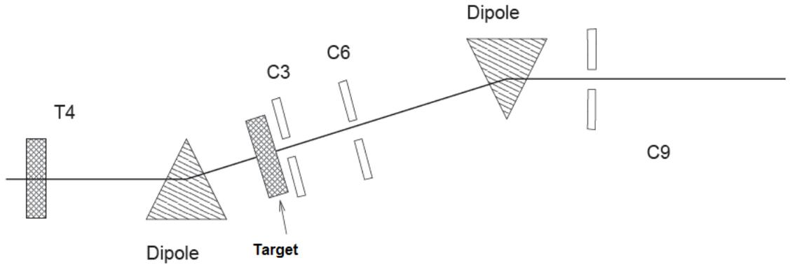
Figure 5.2: Production of a high energy tertiary beam.
