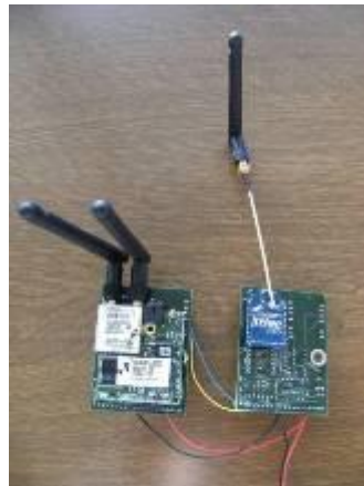
Figure IV- 4 Le multi-support WiFi-ZigBee (2 LiveNodes connectés ensemble)
