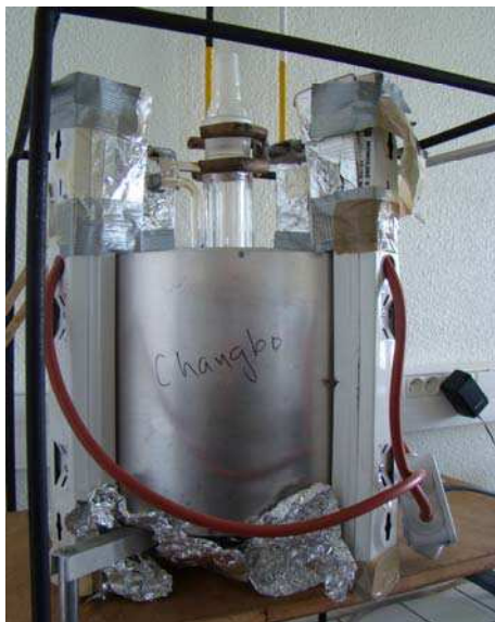
Figure III-C-3 Home-made photoreactor with four tubes (Philips TLD 15W / 05)
