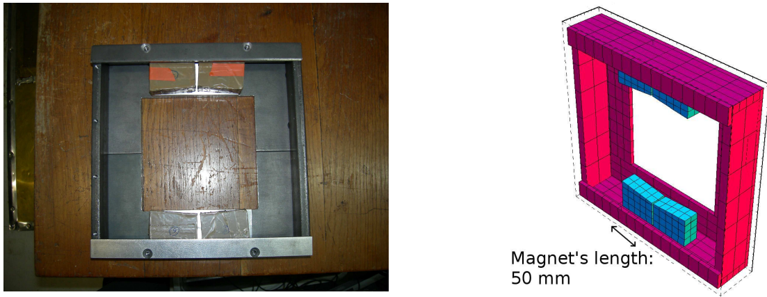
Figure 3.6: The analyzer and its RADIA model. The four magnets are in blue, the return yoke is in red). RADIA parameters were adjusted to fit with the real analyzer field (Table 3.1).
