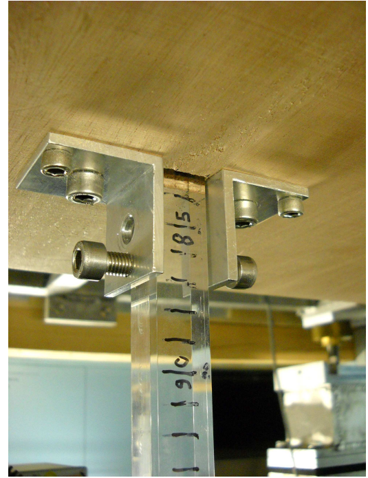
Figure 3.14: Picture of the wooden plate fixed below the magnetic shield (left side), and detail of this plate with the plexiglass stick in (right side).
