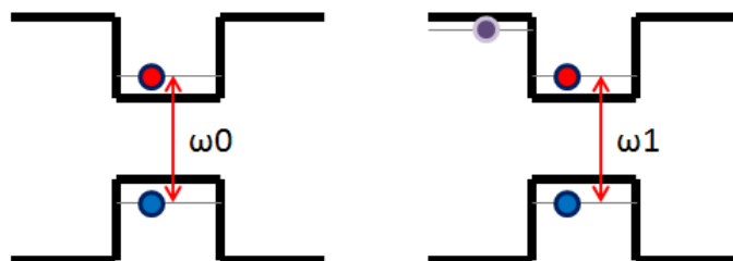
Figure 5.7: Quantum dot Stark effect modelisation. The presence of a charge in the vicinity of the quantum dot modifies the local electric field and Stark shifts the transition energy.
