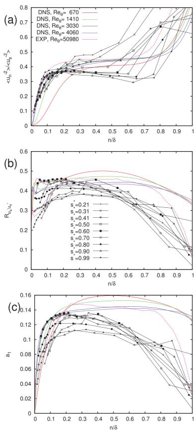
Figure 5.28: Second order correlation ratios (a)  $\overline{u_n'^2}/\overline{u_s'^2}$  (b)  $R_{u_s'u_n'}$  (c)  $a_1$ . Lines for visual aid only. Color solid lines indicate the DNS results of Schlatter & Örlü (2010). Pink dotted lines indicate the experimental results of Skåre & Krogstad (1994).
