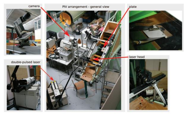
Figure 3.26: Set-up of PIV.
