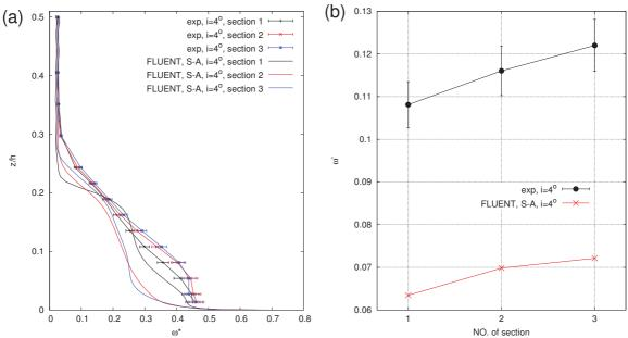
Figure 4.18: Comparisons of experimental and numerical results. Lines for visual aid only. (a) Pitchwise-mass-averaged total pressure loss coefficient  $\omega^*$ ,  $i=4^\circ$ ; (b) mass-averaged total pressure loss coefficient  $\omega'$  versus incidence,  $i=4^\circ$ .
