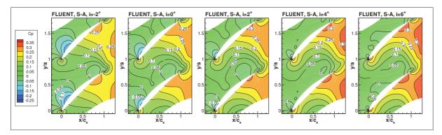
Figure 4.13: Numerical static pressure coefficients on the endwall at five incidences.
