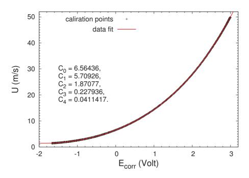
Figure 3.23: Transfer function between bridge voltage and velocity.
