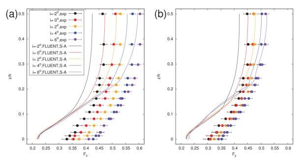
Figure 4.10: Experimental and numerical  $F_x$  and  $F_y$  at five incidences.
