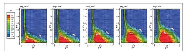
Figure 4.14: Experimental exit total pressure loss coefficient at the outlet section 1 at five incidences. Markers indicate the measurement positions.
