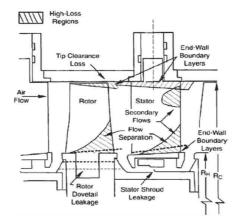
Figure 1.1: High-loss regions in compressors (Wisler, 1985).
