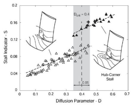
Figure 2.8: *S* and *D*, when Re, AR,  $\delta/c$  are constant (Lei *et al.*, 2008).
