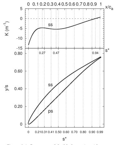
Figure 3.6: Curvature of the blade suction side.
