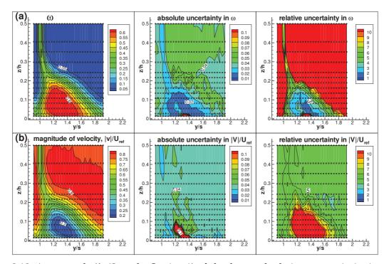
Figure 3.18: An example ( $i=4^{\circ}$ , outlet Section 1) of absolute and relative uncertainties in results measured by the five-hole pressure probe: (a) total losses coefficient; (b)magnitude of velocity. Markers indicate the measurement positions.
