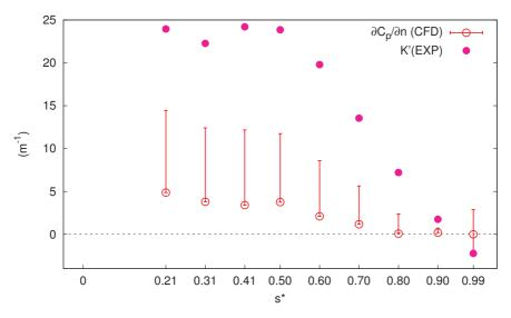
Figure 5.6: Effects of wall-normal pressure gradient and curvature at mid-span,  $i=4^{\circ}$ .
