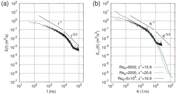
Figure 4.3: Spectra of streamwise velocity at the point where z=0.17 mm and z<sup>+</sup>=15.9, measured by HWA. (a) Frequency spectrum. (b) Spatial spectrum, green and blue lines show the experimental spectra from Metzger *et al.* (2001).
