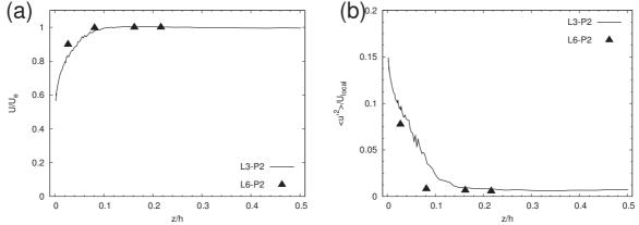
Figure 4.4: Evolution of boundary layer in streamwise direction.
