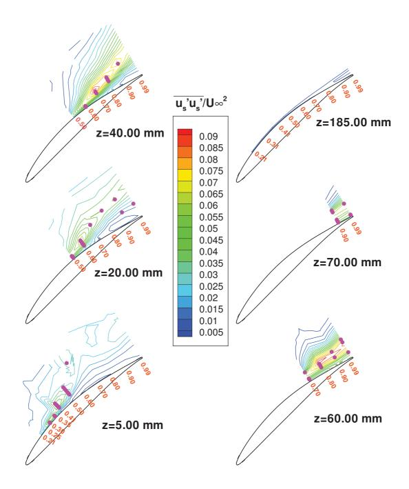
Figure 6.8: LDA experimental results of  $\overline{u_s'u_s'}/U_\infty^2$  in the cross sections in the spanwise direction. Pink points, the points with bimodal histograms.
