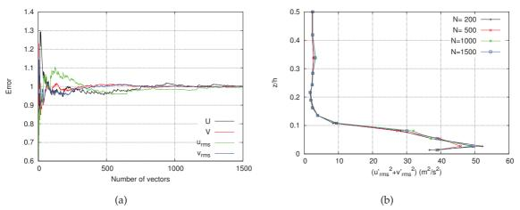
Figure 3.29: Convergence statistics at the reference points,  $x/c_a$ =0.683 and y/s=0.827. (a) Convergence statistics at z=10 mm; (b) convergence of turbulence intensity in spanwise direction.
