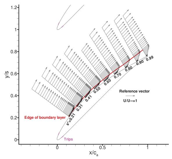
Figure 5.7: Experimental results of mean velocity vector  $\vec{U}/U_{\infty}$  at mid-span, i=4°. Red solid line, the edge of the boundary layer by connecting every point where the mean velocity is largest at its measurement station.
