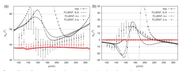
Figure D.11: Experimental and numerical results of angles at the first measurement sections,  $i=4^{\circ}$ . z/h=20.00 mm/370.00 mm=5.4%, at mid-span, black lines; z/h=185.00 mm/370.00 mm=50.0%, near the endwall, red lines.
