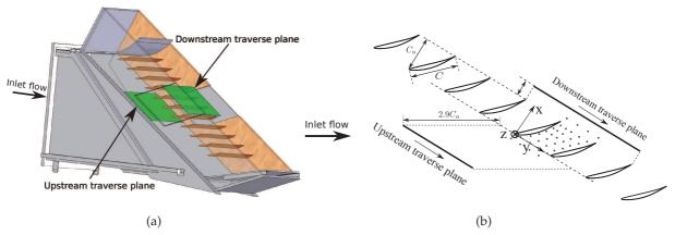
Figure 3.15: Measurement positions of the five-hole pressure probe.
