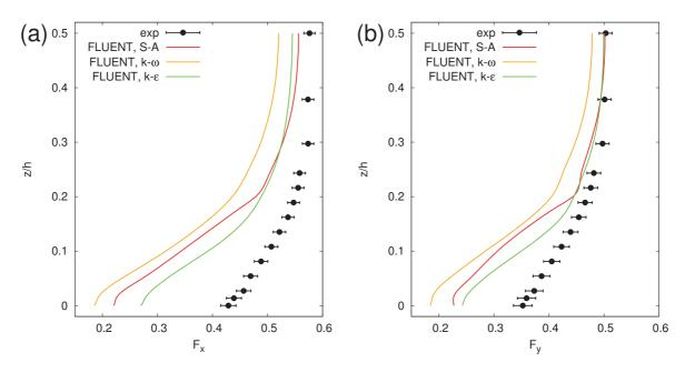
Figure D.3: Experimental and numerical  $F_x$ ,  $F_y$  at i=4 $^{\circ}$ .
