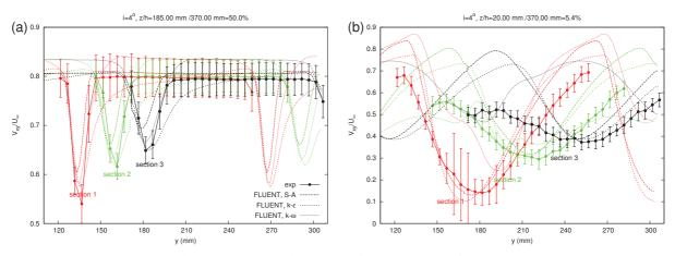
Figure D.9: Experimental and numerical results of magnitude of the vector in x-y planes, i=4 $^{\circ}$ . (a) Mid-span; (b) near the endwall.
