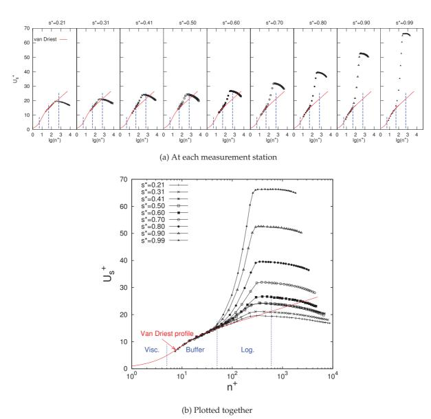
Figure 5.17: Mean velocity profiles in inner coordinate.
