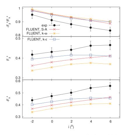
Figure D.4: Experimental and numerical  $F_x^*$ ,  $F_y^*$  and  $F_y^*/F_x^*$ .
