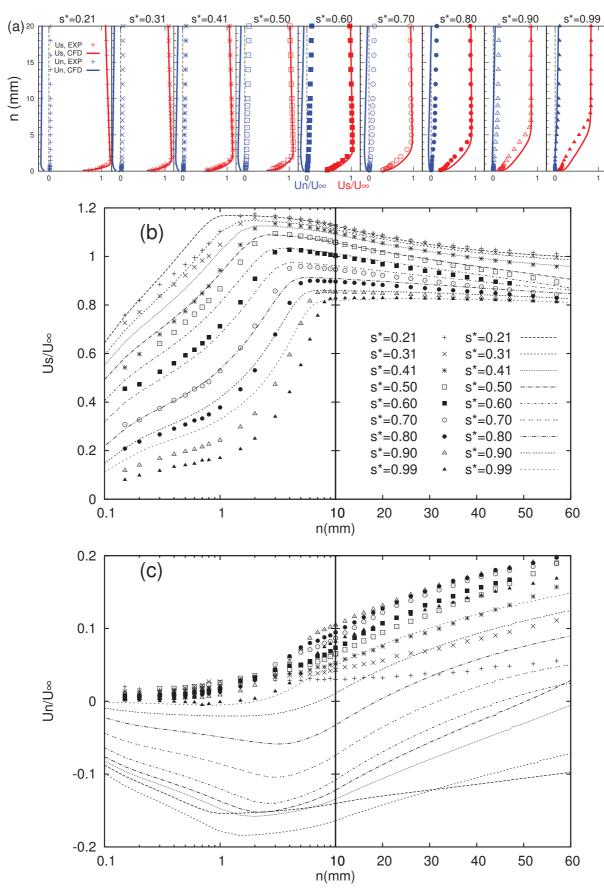
Figure 5.8: Experimental and numerical results of mean velocity at mid-span, i=4°. Numerical tool, FLUENT with the S-A turbulence model. (a)  $U_s$  with red colour,  $U_n$  with blue colour; (b)  $U_s$ ; (c)  $U_n$ .
