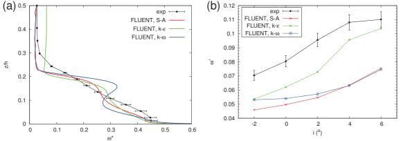
Figure D.7: (a) Experimental and numerical  $\omega^*$  at the outlet section 1 at i=4°, (b) experimental and numerical  $\omega'$  versus incidence.
