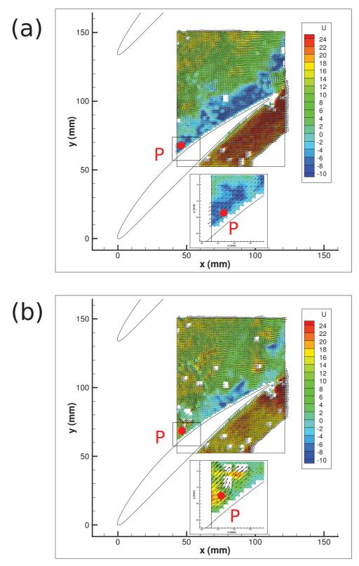
Figure 6.27: Instantaneous flow fields in the corner region, measured by PIV. Colored with axial velocity.
