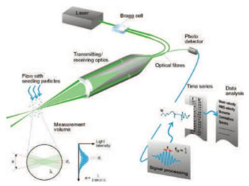
Figure 3.31: LDA principle from Dantec.
