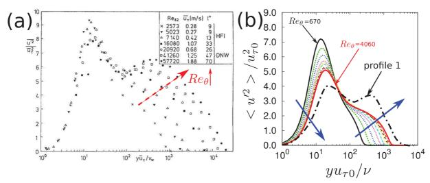
Figure 5.20: (a) Developments of Reynolds stresses  $\overline{u'^2}/u_\tau^2$  with  $Re_\theta$  in TBLs with ZPG, summarized by Fernholz & Finley (1996), also mentioned by the recent review of Marusic *et al.* (2010). (b) Effects of upstream flow on  $\overline{u'^2}$ , by adding profile 1 and profile 2 in Fig. 5.19a3. Blue arrows indicate the streamwise direction.
