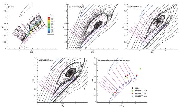
Figure D.12: Comparison of experimental and numerical results of mean velocity at z=5.00 mm, i=4°. (a) LDA experiment; (b) S-A (c) k- $\epsilon$  (d) k- $\omega$  turbulent models; (e) statistics of separation points and vortex cores.
