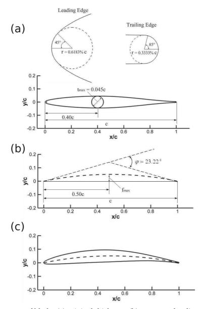
Figure 3.3: Parameters of blade: (a) original thickness; (b) mean camber line; (c) cross section, in the coordinates of blade.
