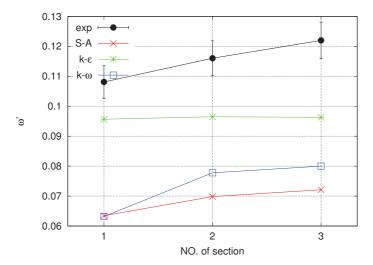
Figure D.8: Experimental and numerical developments of  $\omega'$  in the outlet sections at  $i=4^{\circ}$ . Lines for visual aid only.
