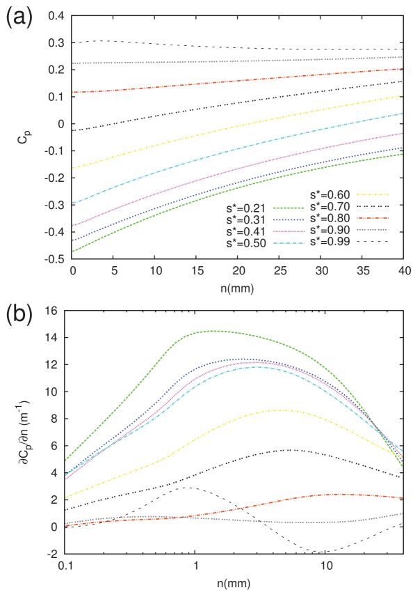
Figure 5.4: Numerical results of (a) static pressures and (b) their gradients at the measurement stations at mid-span,  $i=4^{\circ}$ . CFD tool, FLUENT with the S-A turbulence model.
