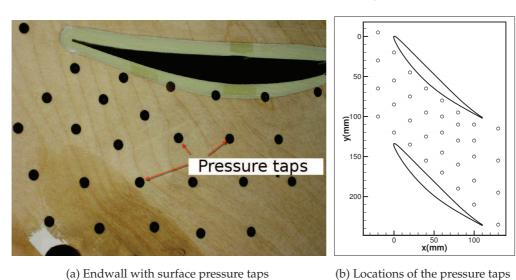
Figure 3.9: Pressure taps on the endwall.
