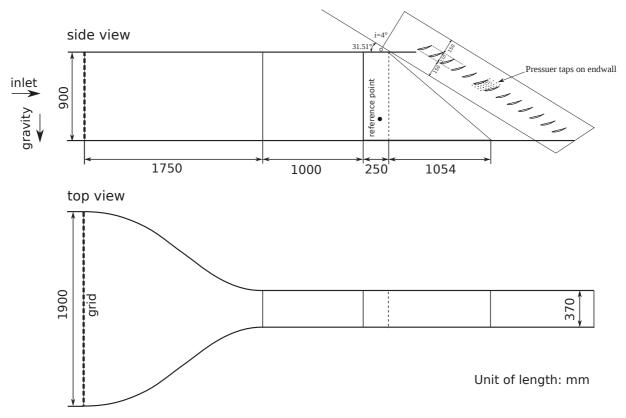
Figure 3.2: Side and top views of the cascade.
