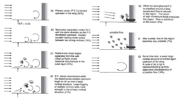
Figure 6.16: Descriptive model for the sequence of flow events in the nose region of a Rood wing-body junction, from Kim *et al.* (1991) and Simpson (2001). The percentage in parenthesis represents the approximate time proportion of the event.
