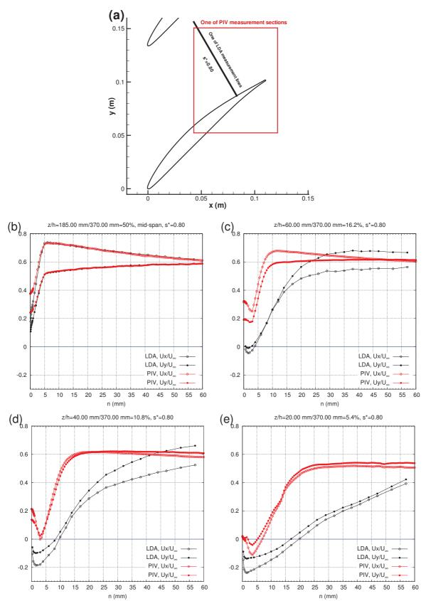
Figure 6.13: Comparison of mean velocities between LDA and PIV along the line of  $s^*$ =0.80 in x - y plane, i=4°. (a) Location of the line  $s^*$ =0.80; z= (b) 185.00 mm, mid-span, (c) 60.00 mm, (d) 40.00 mm, (e) 20.00 mm.
