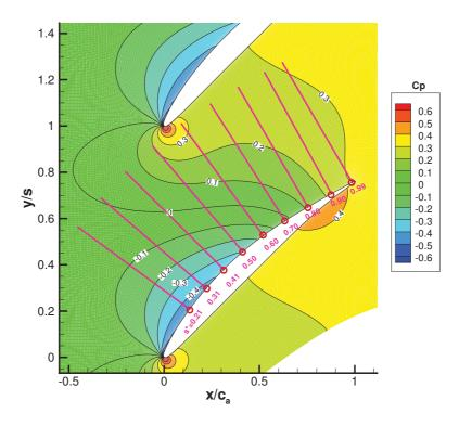
Figure 5.2: Numerical result of the contour of the static pressure at mid-span, i=4 $^{\circ}$ . CFD tool, FLUENT with the S-A turbulence model. Pink lines, LDA measurement stations. Red points, starting points on the suction side along LDA measurement stations.
