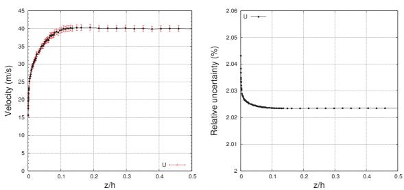
Figure 3.24: Absolute and relative errors of mean velocity measured by HWA.
