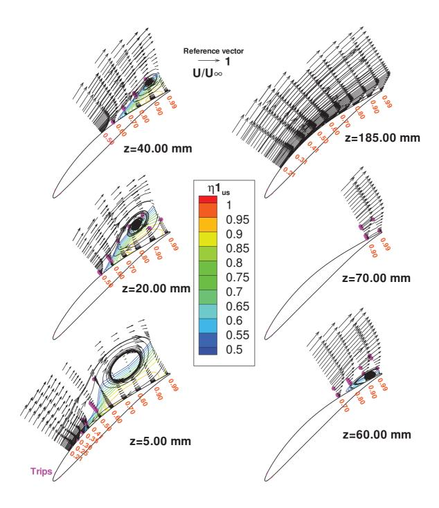
Figure 6.7: LDA experimental results of mean velocity vectors in the cross sections in the spanwise direction, colored by the first backflow coefficient  $\eta_{1_{u_s}}$ . Pink points, the points with bimodal histograms.
