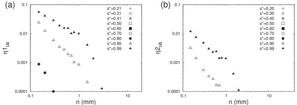
Figure 5.11: Backflow coefficients of streamwise velocity  $u_s$  at mid-span,  $i = 4^{\circ}$ . (a) The first backflow coefficient; (b) the second backflow coefficient.
