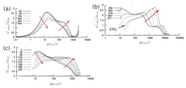
Figure 5.21: Development of  $\overline{u'^2}$  in TBLs with APG. Experimental results, summarized by Shah *et al.* (2009). Red arrows indicate the streamwise direction. (a) DNS, Re $_{\theta}$ <600, Spalart & Watmuff (1993), (b) HWA, Re $_{\theta}$ =7500 $\sim$ 32000 Bernard *et al.* (2003), (c) HWA, Re $_{\theta}$ =1767 $\sim$ 5705, Materny *et al.* (2008). Reference friction velocity  $u_{\tau 0}$  is the friction velocity at the reference measurement station at each measurement.
