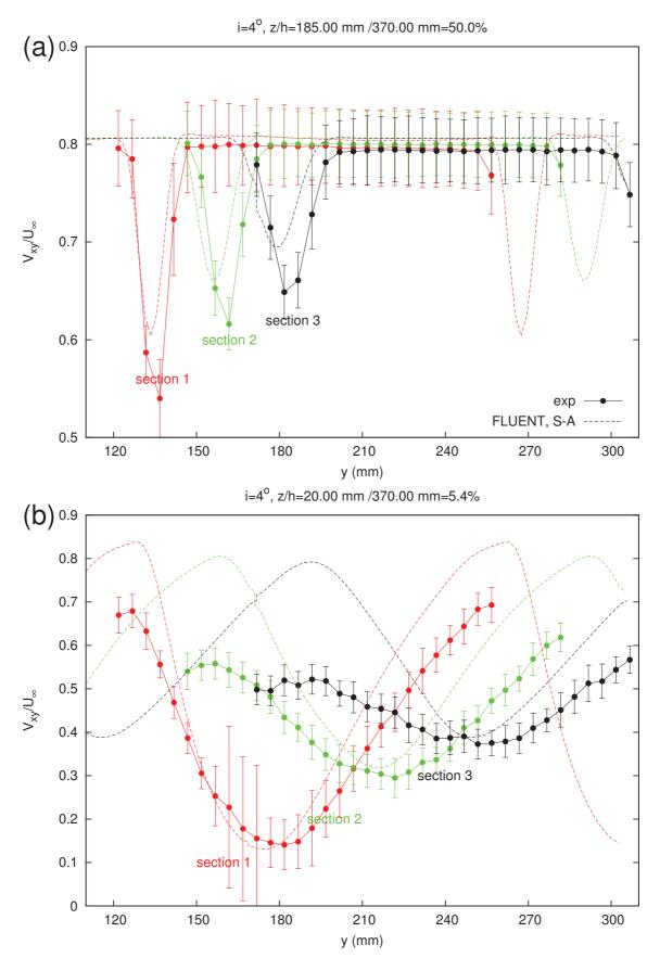
Figure 4.21: Experimental and numerical results of magnitude of the vector in x-y planes, i=4°. (a) z/h=185.00 mm/370.00 mm =50.0%, at mid-span; (b) z/h=20.00 mm/370.00 mm =5.4%, near the endwall.
