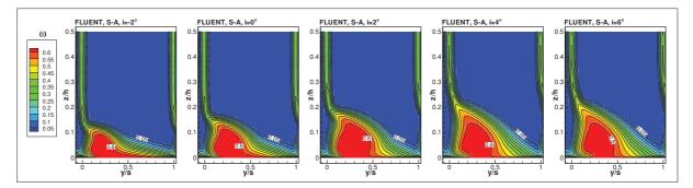
Figure 4.15: Numerical exit total pressure loss coefficient at the outlet section 1 at five incidences.
