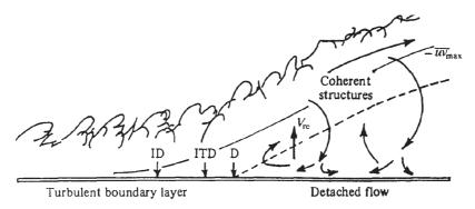
Figure 5.10: Separation process of TBLs proposed by Simpson et al. (1981a; 1981b): incipient detachment (ID),  $\eta_1$ =0.01; intermittent transitory detachment (ITD),  $\eta_1$ =0.20; transitory detachment (TD),  $\eta_1$ =0.50; detachment (D),  $\tau_w$ =0. The dashed line denotes U=0 locations, the solid line denotes maximum turbulent shear locations,  $V_{re}$  denotes the mean re-entrainment velocity along U=0.
