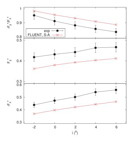
Figure 4.11: Experimental and numerical  $F_x^*$ ,  $F_y^*$  and  $F_y^*/F_x^*$ .
