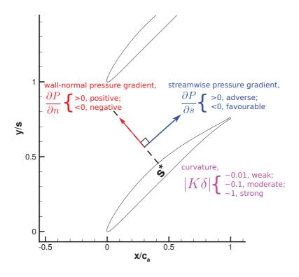
Figure 5.1: Three factors at mid-span.
