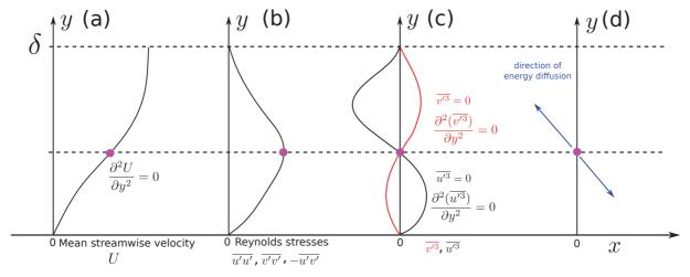
Figure 5.32: Characteristics of a special point in the TBL.
