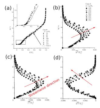
Figure 5.22: Developments of mean velocities and Reynolds stresses in a TBL with APG, from Elsberry *et al.* (2000). Red arrows indicate the streamwise direction. (a) mean velocity, (b)  $\overline{u'^2}$ , (c)  $\overline{v'^2}$ , (d)  $\overline{u'v'}$ .
