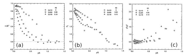
Figure 2.4: Influences of curvature on (a) Reynolds shear stress, (b) turbulent kinetic energy, (c) ratio of Reynolds normal stresses, reviewed by Patel & Sotiropoulos (1997).
