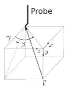
Figure 3.13: Coordinate of the five-hole pressure probe.
