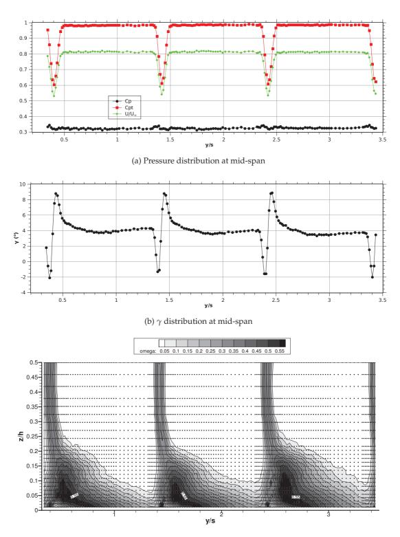
(c) Contour of total pressure loss coefficient, scatters indicate the positions of measurement points Figure 3.39: Periodicity of the test section at outlet.
