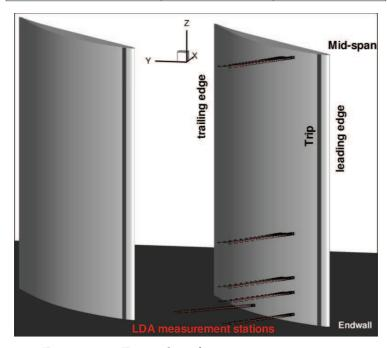
Figure 3.33: Examples of measurement stations.
