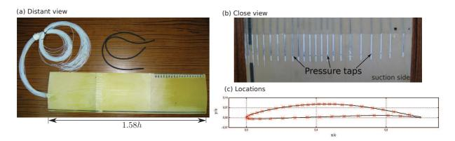
Figure 3.8: Pressure taps on the blade.
