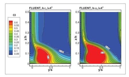
Figure D.6: Numerical results of exit total pressure loss coefficient at the outlet section 1 at i=4°, including the k- $\epsilon$  and k- $\omega$  turbulence models.
