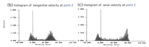
Figure 6.18: Bimodal histograms in a linear cascade, from Hobson *et al.* (1998). (a) LDA measurement stations; (b-c) the histograms of two velocity components at the point 2.
