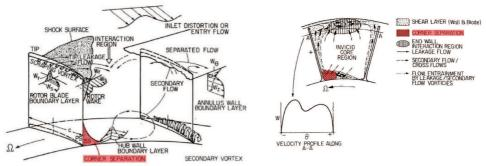
Figure 1.2: Schematic representation of the flow field in an axial flow compressor rotor passage (Lakshminarayana, 1996, left figure, pp.17; right figure, pp.508)
