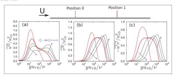
Figure 5.23: Proposed the absolute developments of Reynolds stresses under the effects of upstream flow and APG.  $u_{\tau 0}$ , reference friction velocity at reference position 0. Red dotted lines, profiles at reference position 0. Red solid lines, profiles at position 1 with ZPG. Black solid lines, profiles at position 1 with different APGs. Blue solid arrows, direction of APG increasing.
