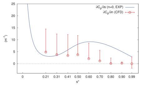
Figure 5.3: Streamwise and wall-normal pressure gradients on the blade suction side at mid-span, i=4°. Blue curve line, experimental streamwise pressure gradient. Red lines, range of variation of these numerical wall-normal pressure gradients in the measurement stations. Red points, numerical wall-normal pressure gradients on the suction side at LDA measurement stations.
