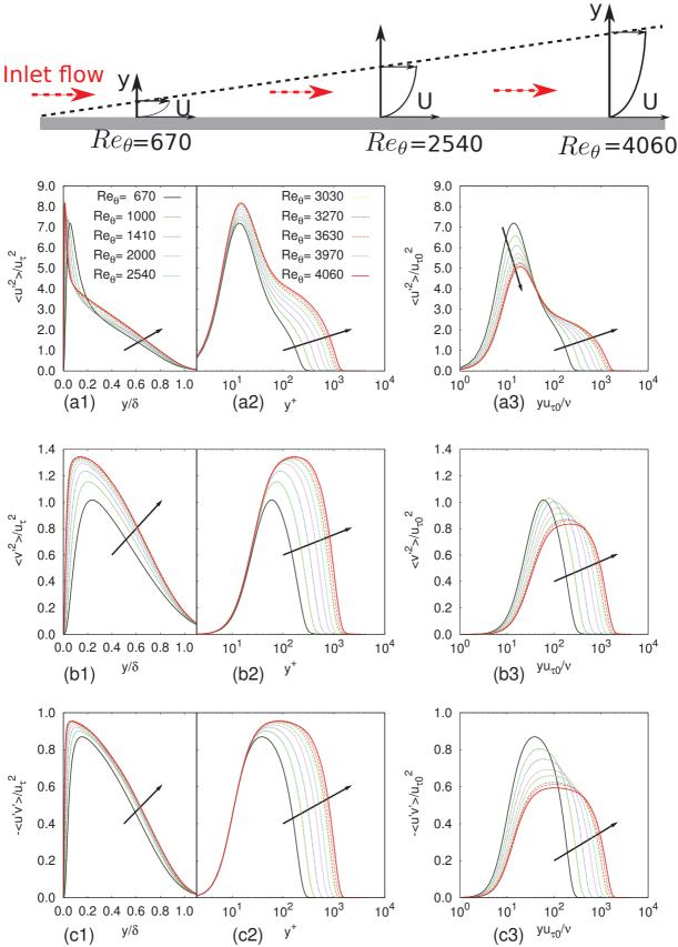
Figure 5.19: Developments of Reynolds stresses in a TBL with ZPG. DNS, from Schlatter & Örlü (2010). The arrows indicate the streamwise direction. Reference friction velocity  $u_{\tau 0}$  is the friction velocity at the first line where  $Re_{\theta}$ =670.
