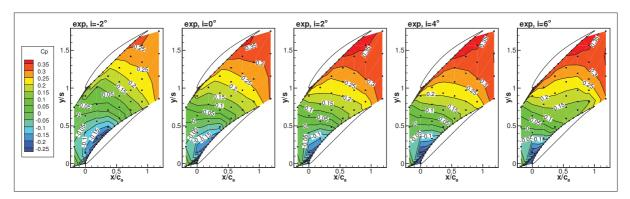
Figure 4.12: Experimental static pressure coefficients on the endwall at five incidences. Markers indicate the measurement positions.
