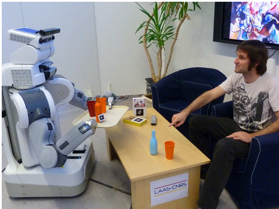
Figure 1.3: Interacting with the robot in an everyday situation: the human asks for help in vague terms, the robot takes into account the human's a priori knowledge and spatial perspective to refine its understanding of the question.
