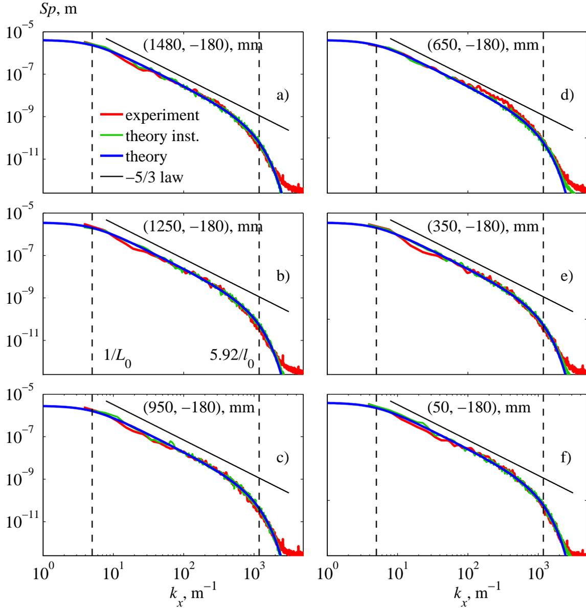
Figure C.1: Additional experimental spectra of the refraction index measured in points placed along the  $x$  axis at  $y = -180$  mm. The experimental data are shown by red line, the von Karman theoretical spectrum with parameters  $L_0 = 20$  cm and  $l_0 = 5$  mm by blue line. Green line corresponds to the spectrum obtained from an artificial realization with the same von Karman spectrum using the processing procedure (C.23). Black line denote Kolmogorov's power law  $k^{-5/3}$ .
