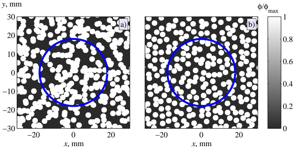
Figure 4.5: Examples of two phase layers: one of the layers is characterized by totally random positions of the circular elements (a), in the second one the elements were randomly moved from centers of a triangular grid (b). The cover ratio is equal to 0.5 for both screens, the diameter of circles  $d = 3$  mm. Blue circles show dimensions of the transducer.
