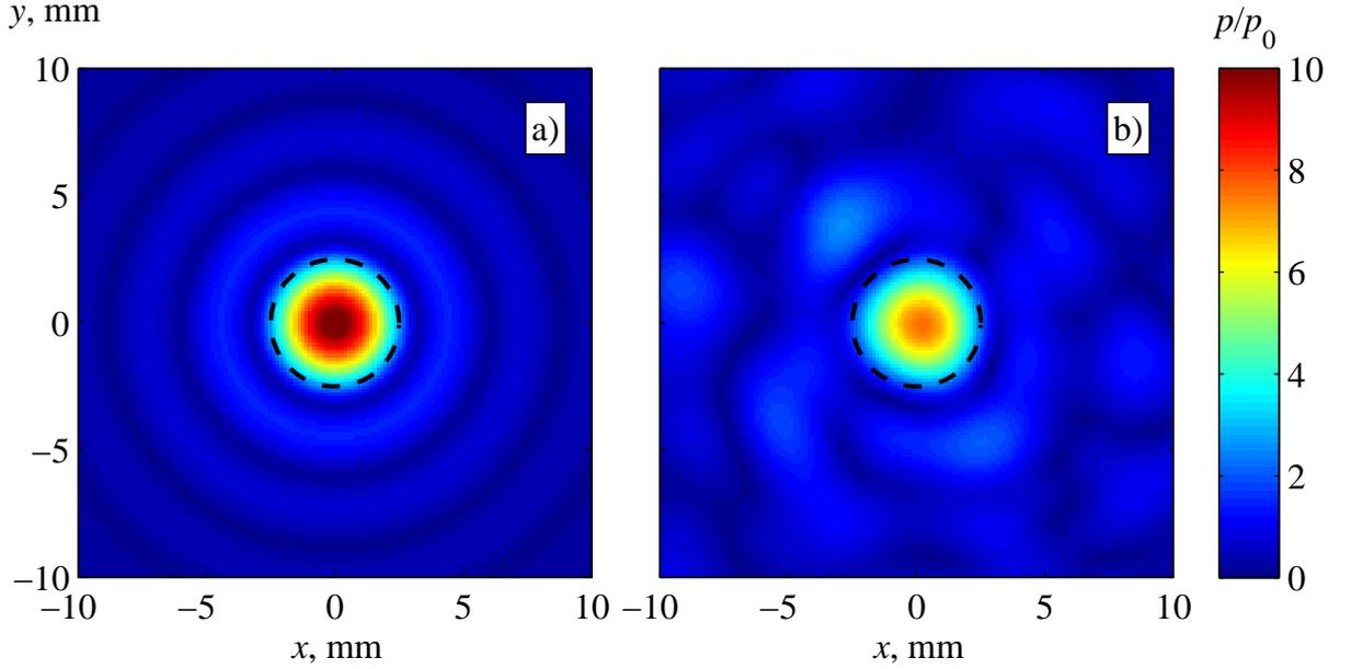
Figure 4.4: An illustration to definition of the focusing quality criterion for the first harmonic: the magnitude of the harmonic in the focal plane  $z = F$  without the phase layer in the beam path (a) and with it (b). The focal area is defined from the *undisturbed* focal distribution at the -6 dB level from its the maximum value.
