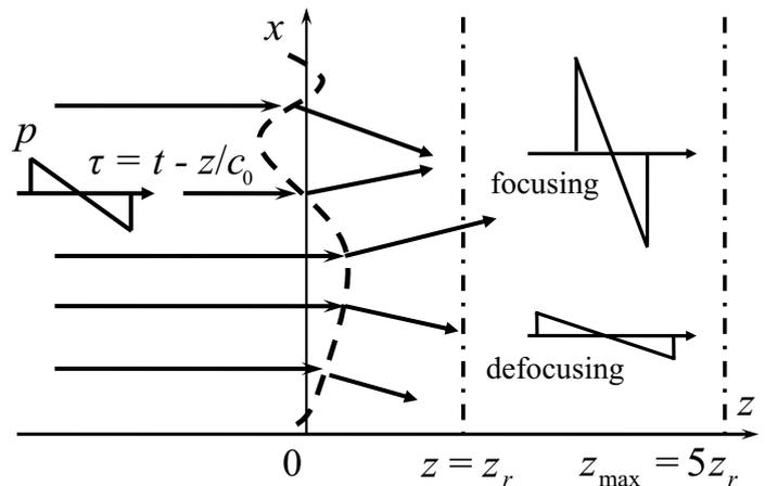
Figure 3.1: Propagation of initially plane  $N$ -wave through infinitely thin phase screen (dashed line) located at  $z = 0$ . Arrows illustrate focusing and defocusing effects behind the screen. The refractive length is denoted as  $z_r$ , maximum propagation distance in numerical simulations is  $z_{\max} = 5z_r$ .
