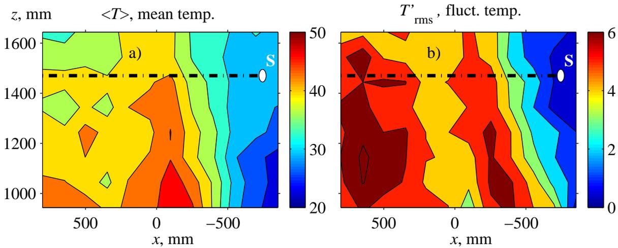
Figure 2.7: The parameters of the turbulent field in the vertical plane ( $x, y = -30 \text{ mm}, z$ ): the average temperature of  $\langle T \rangle$  (a), the rms fluctuation  $\Delta T_{rms}$  (b). Source position is shown by with a white dot next to the letter  $S$ . Propagation path of the  $N$ -wave is marked by a thick dash-dot line.
