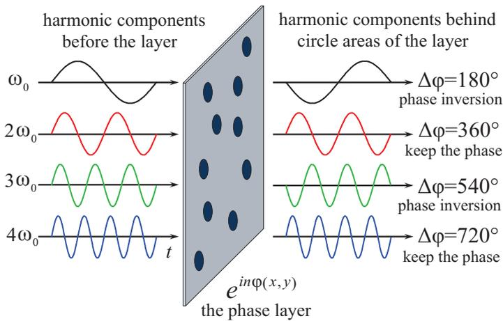
Figure 4.7: An illustration to explanation of phase distortions introduced by the 180° phase layer.
