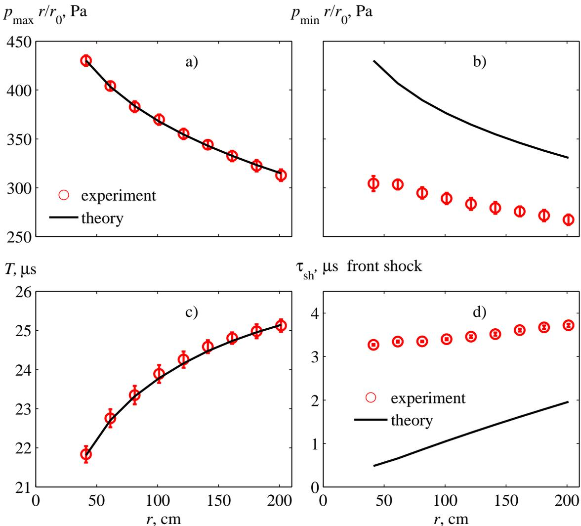
Figure 2.11: Main parameters of the  $N$ -wave, measured in a homogeneous air. The positive peak pressure (a), the negative peak pressure (b), half-duration (c), the front shock risetime (d). Black line shows the results of numerical simulation, red markers – the results of the experiment. Atmospheric conditions were the following:  $p_{\text{atm}} = 97900 \text{ Pa}$ ,  $T_{\text{atm}} = 14.5 \text{ }^\circ\text{C}$ , humidity 35%.
