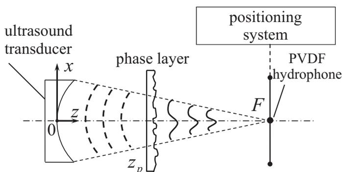
Figure 4.1: Schematic illustration of the problem and a diagram of the experimental setup.
