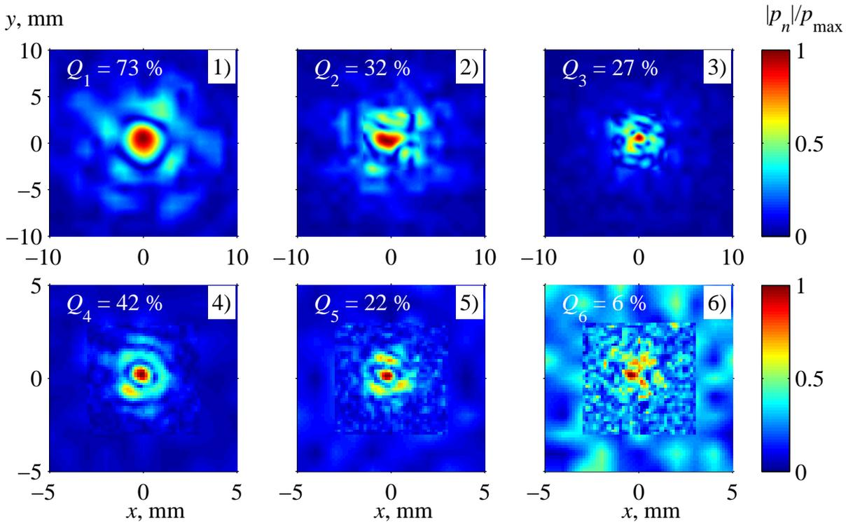
Figure 4.18: Pressure magnitudes of the first 6 harmonics in the focal plane (number in the corner), measured in a case of the  $90^\circ$  phase layer. The layer was placed at the distance from the source  $z_p = 0.71F = 51$  mm. The amplitudes are normalized on their peak values  $p_{max}$ , equal to 1260, 100, 26, 9.3, 3.6 and 1.4 kPa, respectively.
