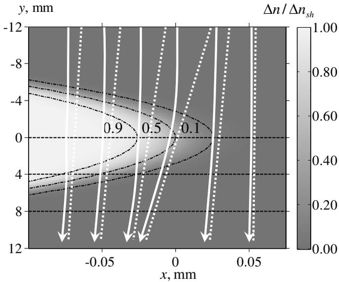
Figure 1.8: Formation of shadows. Spatial variations of refraction index caused by the acoustic shock front in the  $xOy$  plane. Contour dash-dot lines show refraction index levels corresponding to values  $0.1\Delta n_{sh}$ ,  $0.5\Delta n_{sh}$ ,  $0.9\Delta n_{sh}$ . Refraction of optic rays is schematically shown by arrows (solid lines), back propagation of rays is shown by dashed lines.
