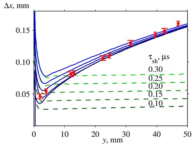
Figure 1.10: Shadow width modeled for images taken at different positions  $y$  of the camera focus. Dashed curves are obtained using the geometrical optics model and solid curves - using the parabolic equation. The change of the contrast in both sets of curves from dark to light corresponds to increasing shock rise time in the modeling. Points with vertical bars are shadow widths and corresponding standard deviations measured from experimental shadowgrams.
