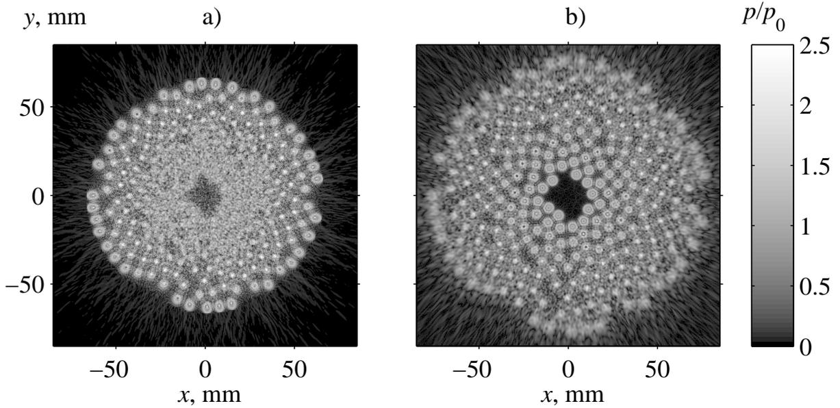
Figure 5.1: Spatial distributions of dimensionless pressure amplitude  $p/p_0$  calculated in a plane  $(x, y, z = 20 \text{ mm})$  near the edge of the radiator (a) and in a plane  $(x, y, z = 0 \text{ mm})$  – "virtual" source (b). Here,  $p_0 = \rho_0 c_0 u_0$ , where  $u_0$  is the amplitude of the vibration velocity at the surface of the array element.
