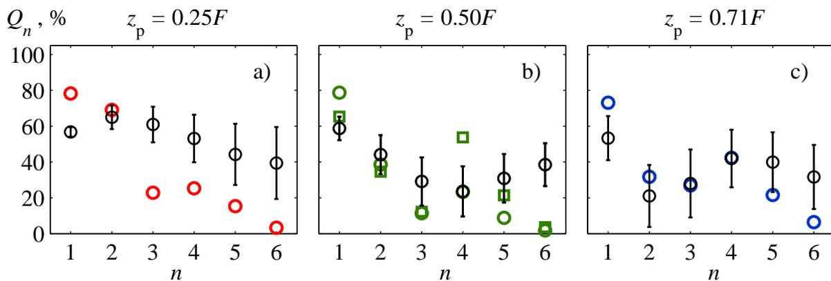
Figure 4.19: Comparison of the focusing quality criterion  $Q_n$  for the first six harmonics with the  $90^\circ$  phase layer placed at the distances  $z_p = 0.25F = 18$  mm (a),  $z_p = 0.50F = 36$  mm (b) and  $z_p = 0.71F = 51$  mm (c): experimental data (color markers) and simulations results (black markers). Different type of the color markers correspond to different realizations of the phase layer obtained by moving it parallel in its own plane.
