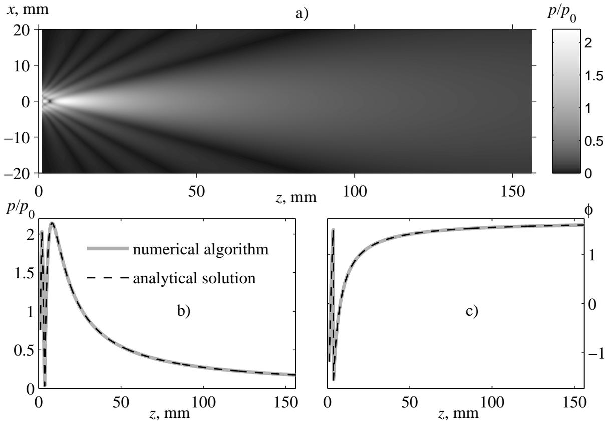
Figure 5.5: Pressure amplitude distribution  $p/p_0$  for a single array element, calculated numerically in a linear approximation in the axial plane of the element (a). Results of linear numerical calculations (solid gray curves) for the pressure amplitude (b) and phase (c) along the element axis in comparison to an analytic solution (thin dashed curves).
