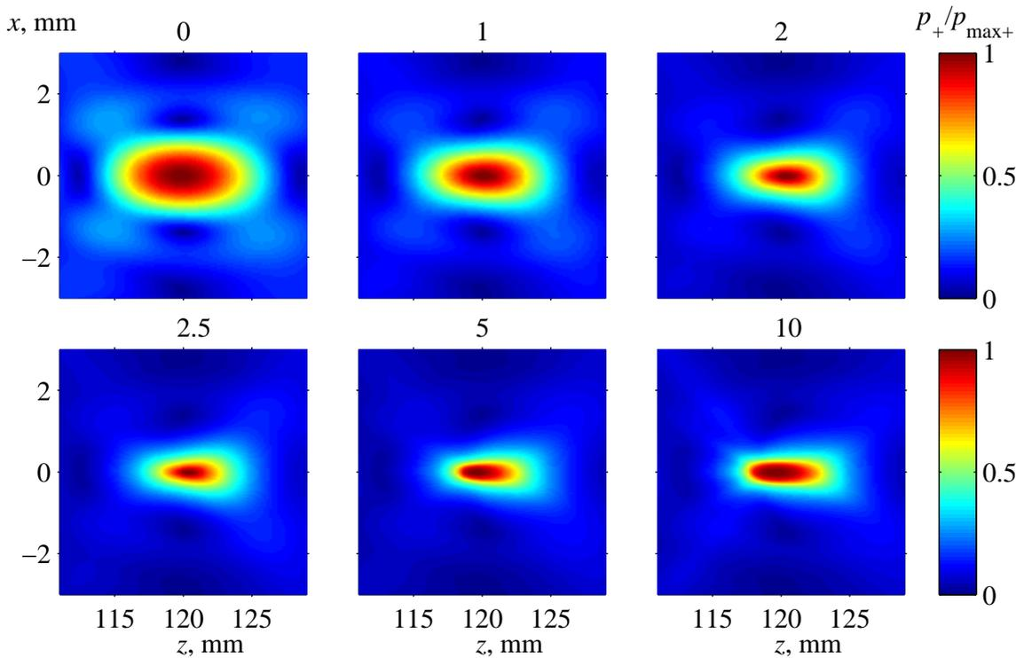
Figure 5.10: Normalized at their maximum distributions of peak positive pressures  $p_+/p_{\max+}$  in a plane  $(x, z)$  near the focus for different initial intensities at the elements 1, 2, 2.5, 5 and 10 W/cm<sup>2</sup>. Scale of the  $x$  axis is stretched 3 times in comparison to the  $z$  axis.
