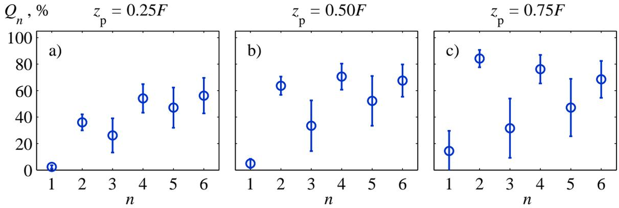
Figure 4.9: Mean values of the focusing quality  $Q_n$  for the first 6 harmonics in a case of the 180° phase layer placed at distances  $z_p = 0.25F$  (a),  $z_p = 0.50F$  (b), and  $z_p = 0.75F$  (c) from the source. Averaging was done using 10 realizations, error bars correspond to standard deviations.
