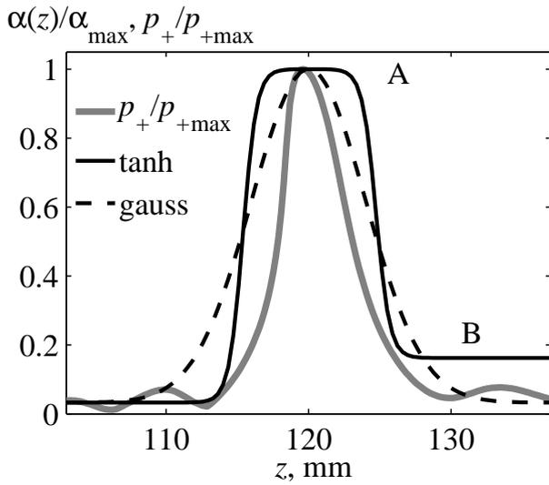
Figure 5.4: An example of the artificial absorption  $\alpha(z)$ , given by the Eq. 5.6 along the  $z$  axis (black solid line), peak positive pressure – gray solid line, and a possible gaussian dependence of the artificial absorption – dashed line. The simulation case corresponds to  $I_0 = 5 \text{ W/cm}^2$  (see sec. 5.4.3). All curves are normalized here to their maximal values.
