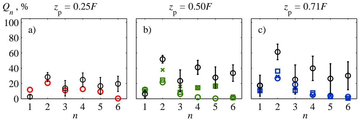
Figure 4.17: Comparison of the focusing quality criterion  $Q_n$  for the first six harmonics with the  $180^\circ$  phase layer placed at the distances  $z_p = 0.25F = 18$  mm (a),  $z_p = 0.50F = 36$  mm (b) and  $z_p = 0.71F = 51$  mm (c): experimental data (color markers) and simulations results (black markers). Different type of the color markers corresponds to different realizations of the phase layer obtained by moving it parallel in the  $(x, y)$  plane.
