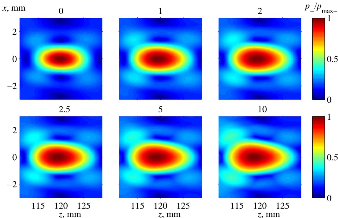
Figure 5.11: Normalized at their maximum distributions of peak negative pressures  $p_-/p_{\max-}$  in a plane  $(x, z)$  near the focus for different initial intensities at the elements 1, 2, 2.5, 5 and 10 W/cm<sup>2</sup>. Scale of the  $x$  axis is stretched 3 times in comparison to the  $z$  axis.
