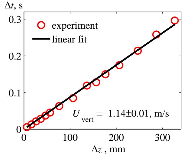
Figure 2.8: Determination of the average lifting speed of the turbulent structures  $U_{\text{vert}}$  using dependence of the time shifting interval between the two signals of the probes, at which the maximum correlation is reached, from the distance between them. Measurements were made at the point (175, -30, 1644) mm. The experiment – red circular markers, linear approximation  $\Delta z = U_{\text{vert}}\Delta t$  – black line.
