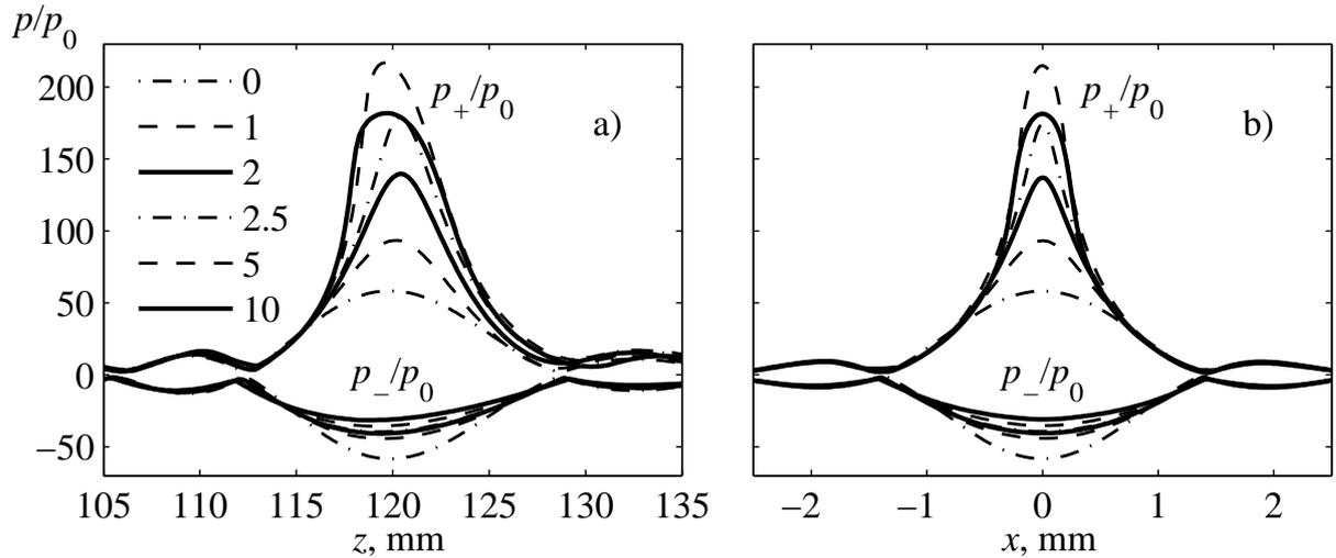
Figure 5.9: Distributions of dimensionless positive  $p_+/p_0$  and negative  $p_-/p_0$  peak pressures along the axis of the array (a) and in the focal plane along the  $x$  axis (b) at various initial intensities: 0 – linear focusing (dotted line); the remaining numerals next to the curves correspond to intensities on the array elements, measured in  $\text{W}/\text{cm}^2$ .
