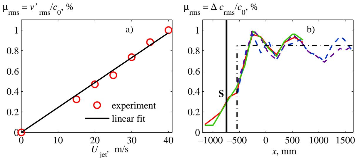
Figure 2.24: The rms fluctuations of the refraction index measured in the experiment with the jet (Fig. 2.23a,  $U_{\text{jet}}$  is flow velocity at the exit of the jet) and along the  $N$ -wave propagation path in the experiment with heating grid (Fig. 2.23b).
