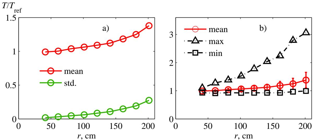
Figure 2.18: Average characteristics of the  $N$ -wave duration derived from temporal moments (Eq. 2.13) and normalized to values in a homogeneous medium  $T/T_{ref}$ . The graph shows the mean value (red line) and the standard deviation (green line) (a), as well as maximum (triangle markers) and minimum (square markers) values observed in the sample (b).
