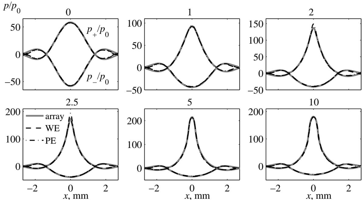
Figure 5.16: Comparison of the peak pressures in the focal plane along the  $x$  axis, obtained in modeling of the field of the array (solid gray line) and the fields of equivalent sources. Notations are the same as in Fig. 5.14.
