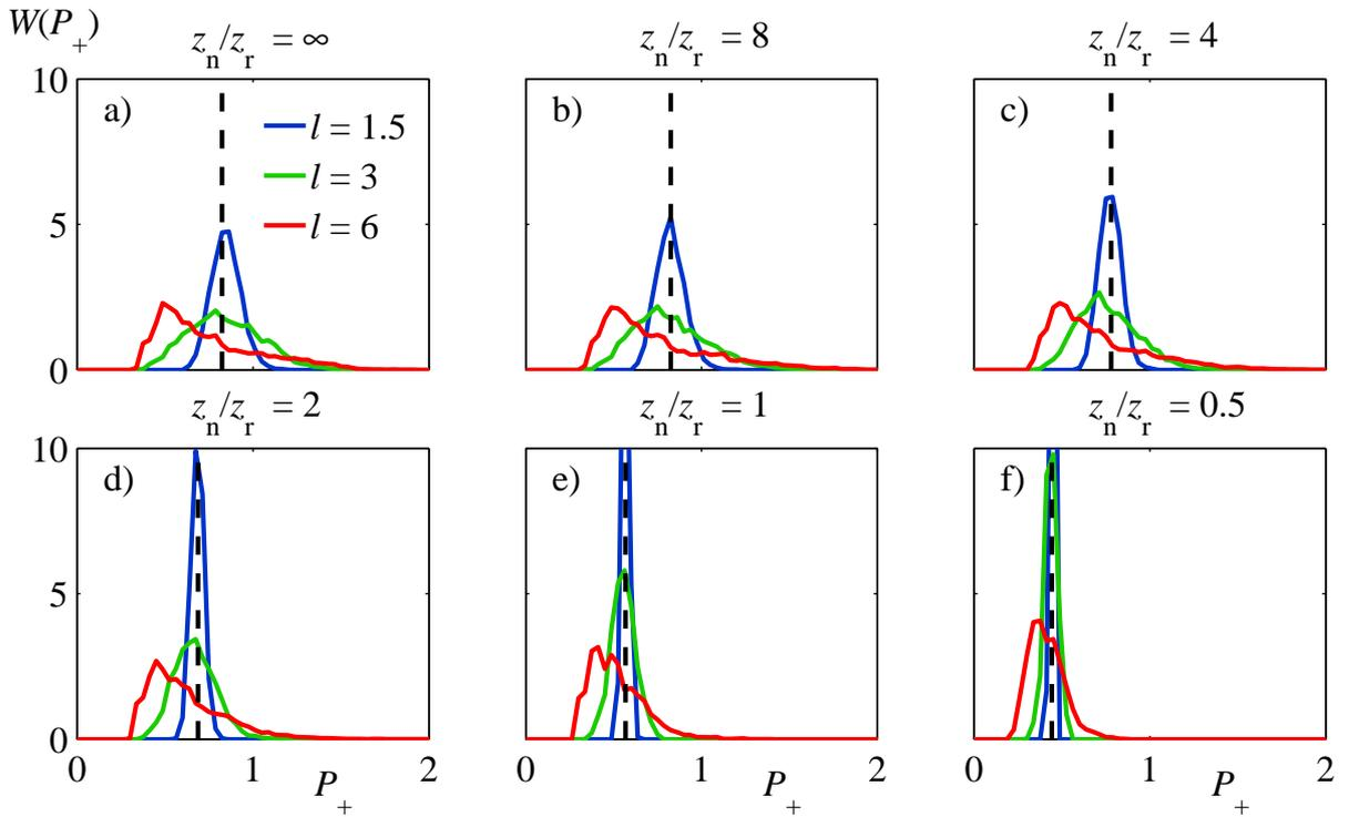
Figure 3.7: Comparison between probability distribution functions of the  $N$ -wave peak positive pressure obtained at the distance  $z = 2z_r$  for various nonlinear lengths  $z_n$ : linear (a),  $z_n = 8z_r$  (b),  $z_n = 4z_r$  (c),  $z_n = 2z_r$  (d),  $z_n = z_r$  (e) and  $z_n = 0.5z_r$  (f). Correlation lengths of the screens are:  $l = 6$  (red curve),  $l = 3$  (green curve),  $l = 1.5$  (blue curve).
