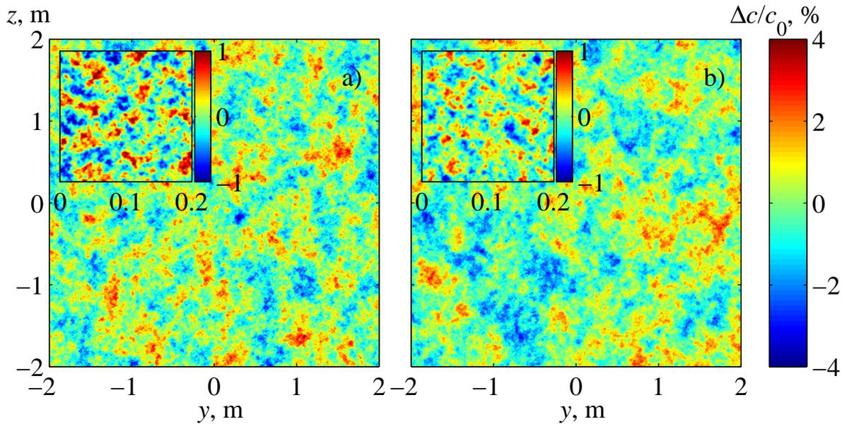
Figure 2.2: Realizations of the turbulent fields, constructed on the basis of the von Karman spectrum of vector (a) and scalar (b) types. In the tabs, given the increased 10-fold with filtered low-frequency field components.
