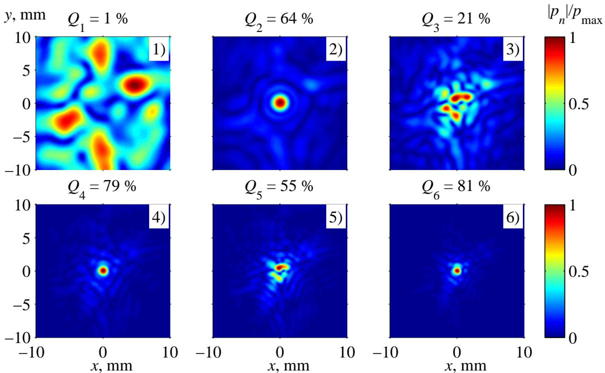
Figure 4.8: Spatial distributions of the pressure magnitude of the first 6 harmonics (number in the corner) in case of the 180° phase layer ( $d = 3$  mm) placed at  $z_p = 0.5F = 35$  mm distance from the source. The focusing quality  $Q_n$  is given at the top of each image. The characteristic feature of the example is low focusing quality of the odd harmonics and high quality of even harmonics.
