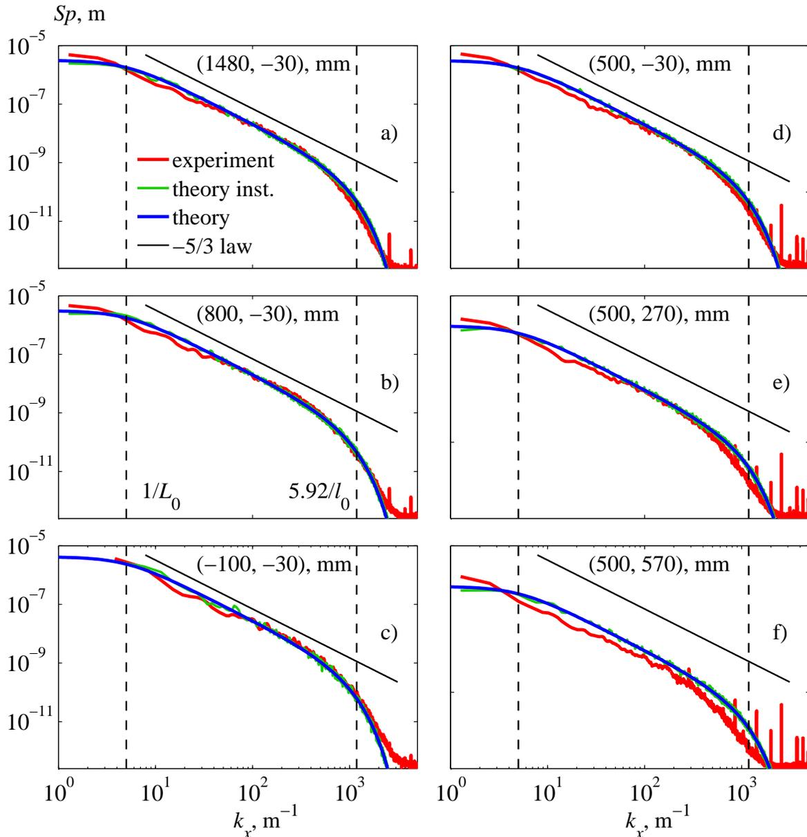
Figure 2.10: One-dimensional spectra of fluctuations of the refractive index obtained experimentally (red line) and by the von Karman model spectrum with the parameters of  $L_0 = 20$  cm,  $l_0 = 5$  mm (blue line). The green line shows a spectrum obtained by processing the artificial realization with the von Kármán spectrum using the same methodology (see Appenix. C), as in the processing of experimental spectra. Black line corresponds to the law  $k^{-5/3}$ .
