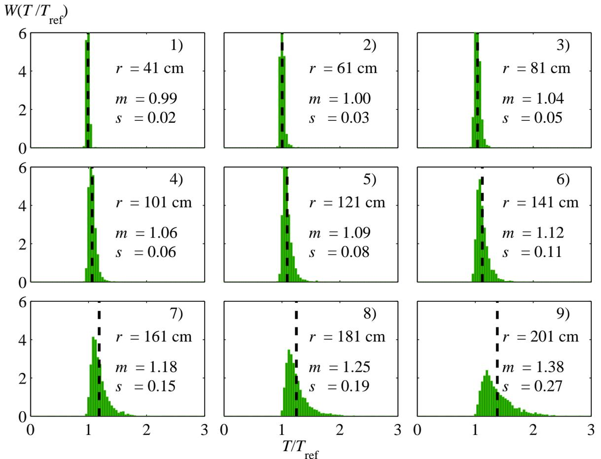
Figure 2.17: Histograms of the statistical distributions of the  $N$ -wave duration derived from temporal moments (Eq. 2.13) and normalized to the corresponding values in a homogeneous medium,  $T/T_{\text{ref}}$ . Black dashed line shows the average value of each distribution. Values for the source-microphones distance  $r$ , the mean  $m$  and standard deviation  $s$  are given on the graphs. Class size is 0.04.
