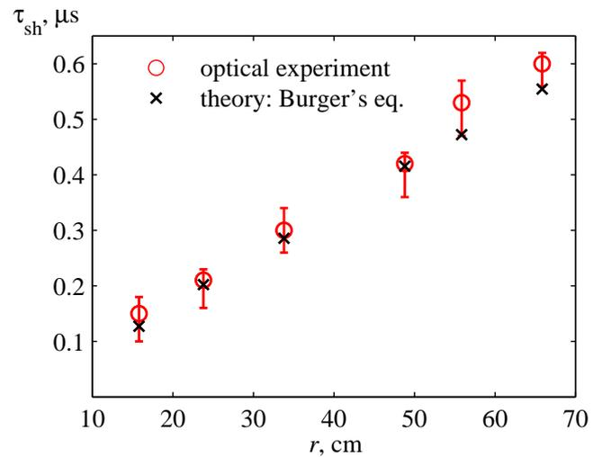
Figure 1.12: Comparison between the optically measured rise time (circles) and the rise time predicted by using the acoustic wave propagation (crosses, Eq. 1.1) at different distances from the spark source.
