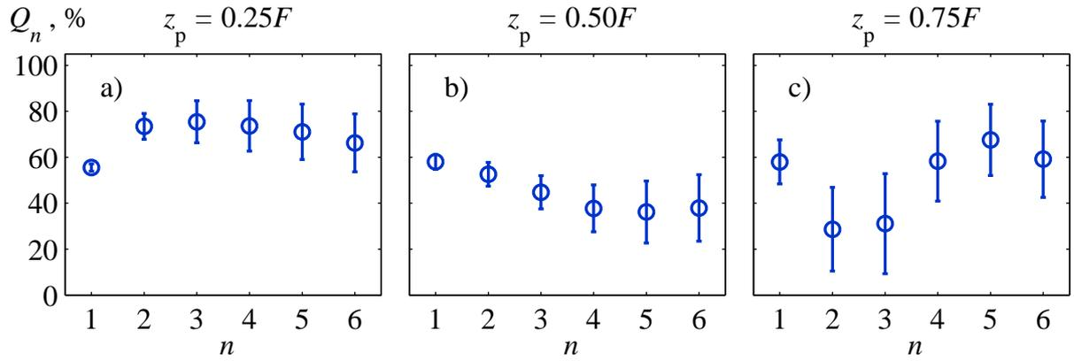
Figure 4.11: Mean values of the focusing quality  $Q_n$  for the first 6 harmonics in a case of the 90° phase layer placed at distances  $z_p = 0.25F$  (a),  $z_p = 0.50F$  (b), and  $z_p = 0.75F$  (c) from the source. Averaging was done using 10 realizations, error bars correspond to standard deviations.
