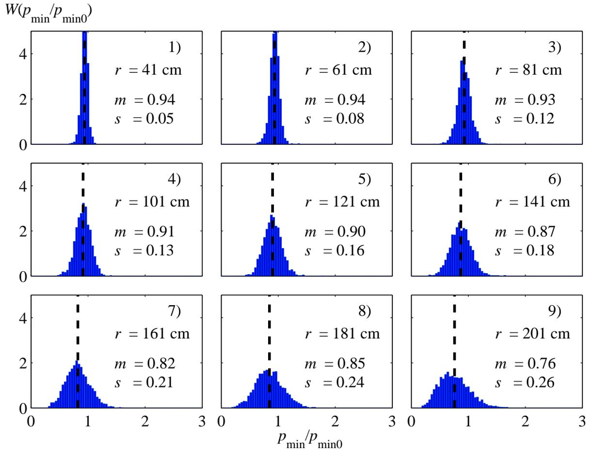
Figure 2.15: Histograms of the statistical distributions of the peak negative pressure, normalized to the corresponding values in a homogeneous medium,  $p_{\min}/p_{\min 0}$ . Black dashed line shows the average value of each distribution. Values for the source-microphones distance  $r$ , the mean  $m$  and standard deviation  $s$  are given on the graphs. Class size is 0.04.
