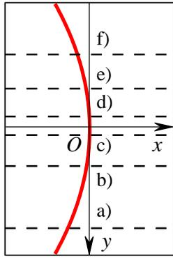
Figure 1.5: Positions of the camera observation plane along the  $y$  axis that correspond to the shadowgrams given in Fig. 1.6: 32 mm (a), 12 mm (b), 2 mm (c), -4 mm (d), -13 mm (e), and -24 mm (f). Shock wavefront is plotted schematically as a red solid curve.
