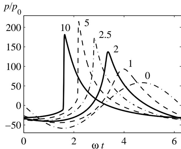
Figure 5.8: Dimensionless pressure waveforms in the geometric focus of the array ( $x = 0, y = 0, z = F$ ), calculated at different initial intensity levels on array elements: 1, 2, 2.5, 5, and 10 W/cm<sup>2</sup> (numbers next to the curves); 0 – linear focusing of the field.
