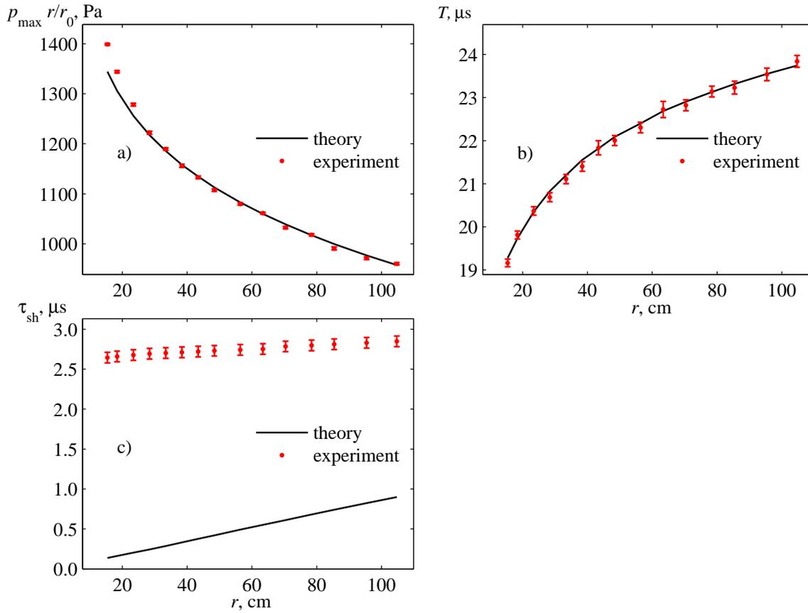
Figure 1.4: Theoretical (solid line) and experimental (markers with error bars) data for peak positive pressure (a), half duration (b), and rise time (c) of the wave.
