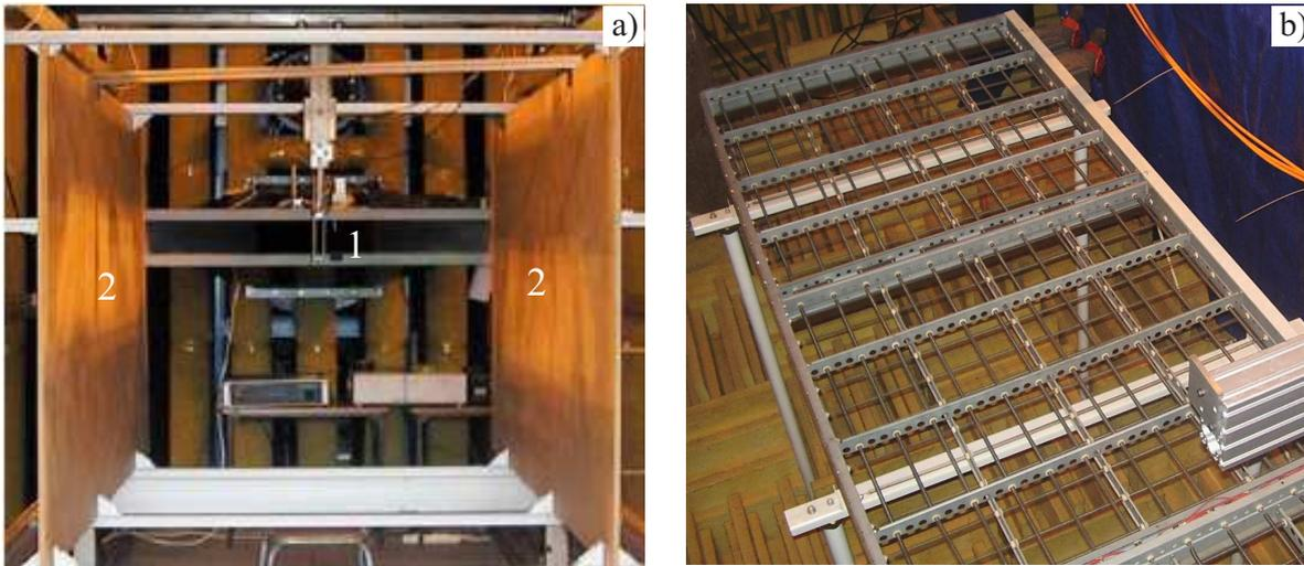
Figure 2.23: Two experiments on  $N$ -wave propagation through turbulent media: experiment with jet flow (1) expanded between two wooden baffles (2) – kinematic turbulence case, (a), and experiment with heating grid – scalar turbulence case, (b).
