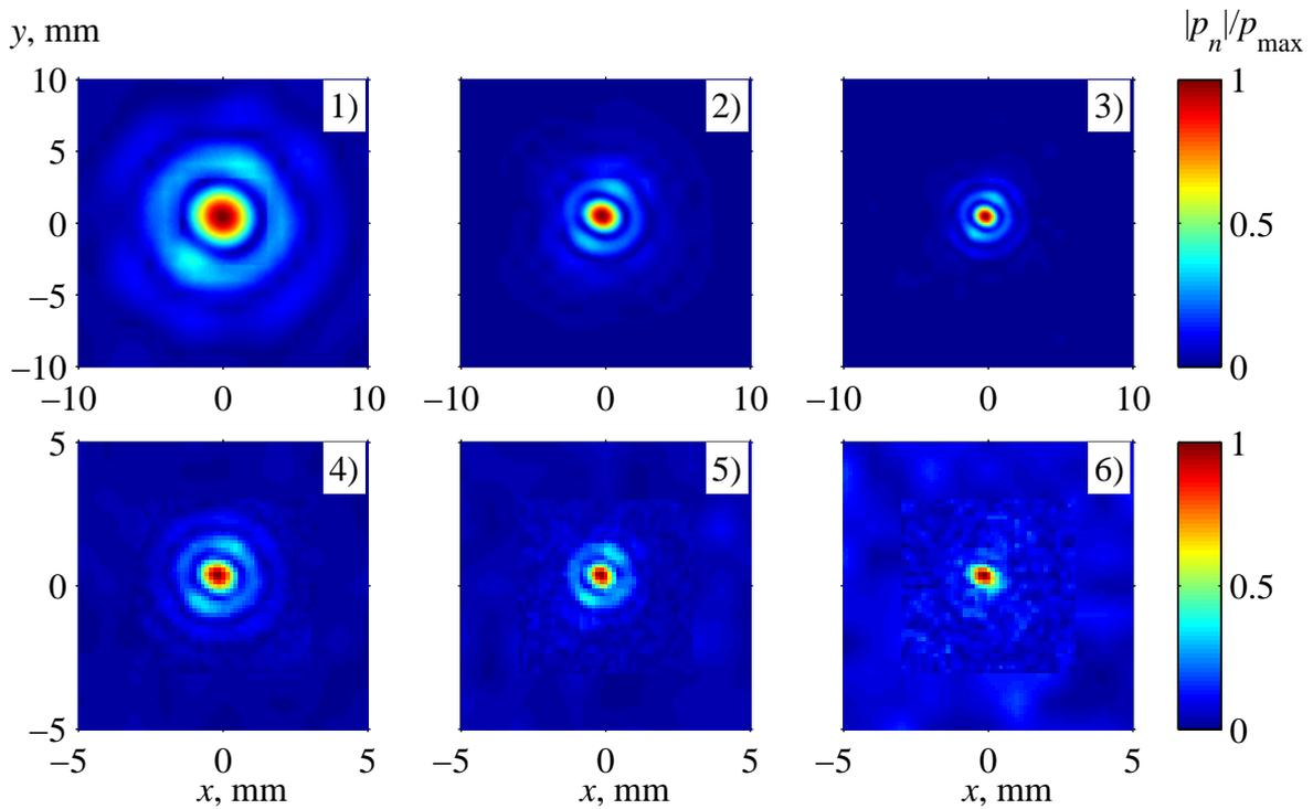
Figure 4.15: Pressure magnitudes of the first 6 harmonics in the focal plane (the number is in the corner), measured without the phase layer. The amplitudes are normalized on their peak values  $p_{\max}$ , equal to 2000, 420, 150, 55, 28 and 14 kPa, respectively.
