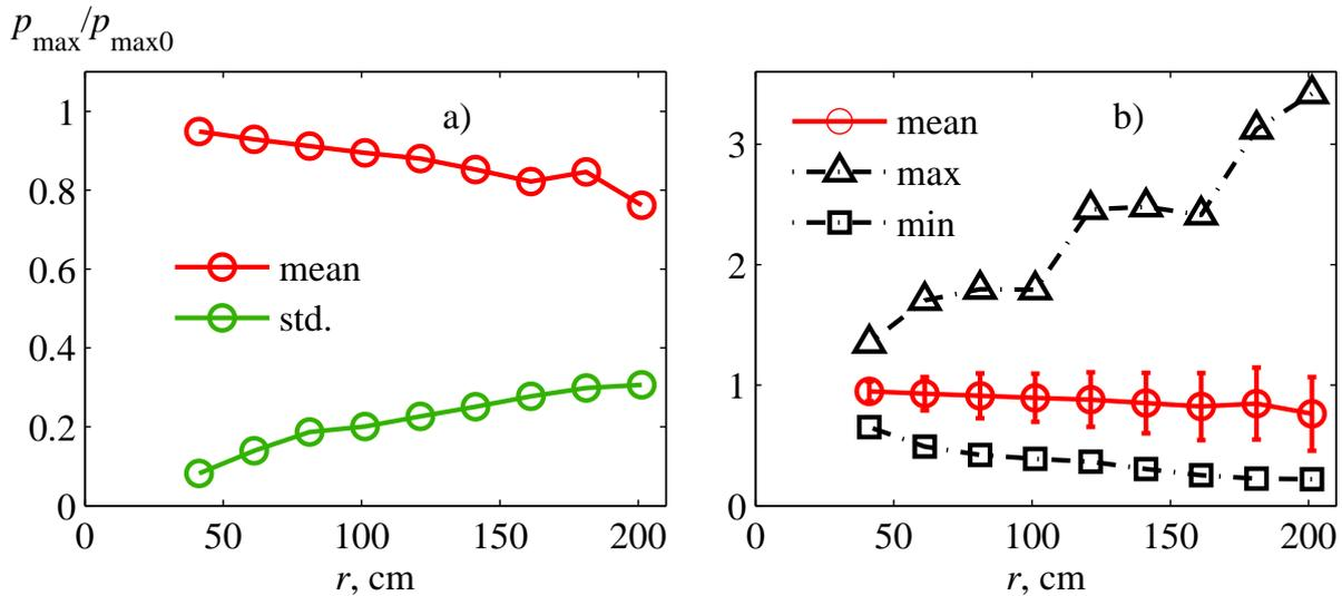
Figure 2.14: Average characteristics of the peak positive pressure, normalized to values in a homogeneous medium  $p_{\max}/p_{\max0}$ . The graph shows the mean value (red line) and the standard deviation (green line) (a), as well as maximum (triangle markers) and minimum (square markers) values observed in the sample (b).
