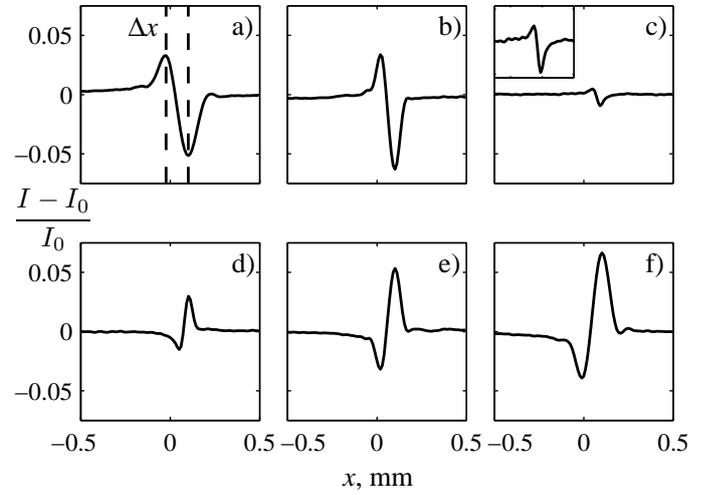
Figure 1.7: Normalized intensity distributions  $(I-I_0)/I_0$  along the  $x$ -axis obtained from shadowgrams given in Fig. 1.6.  $I_0$  is the background intensity. In the subplot (c) a zoom is plotted.
