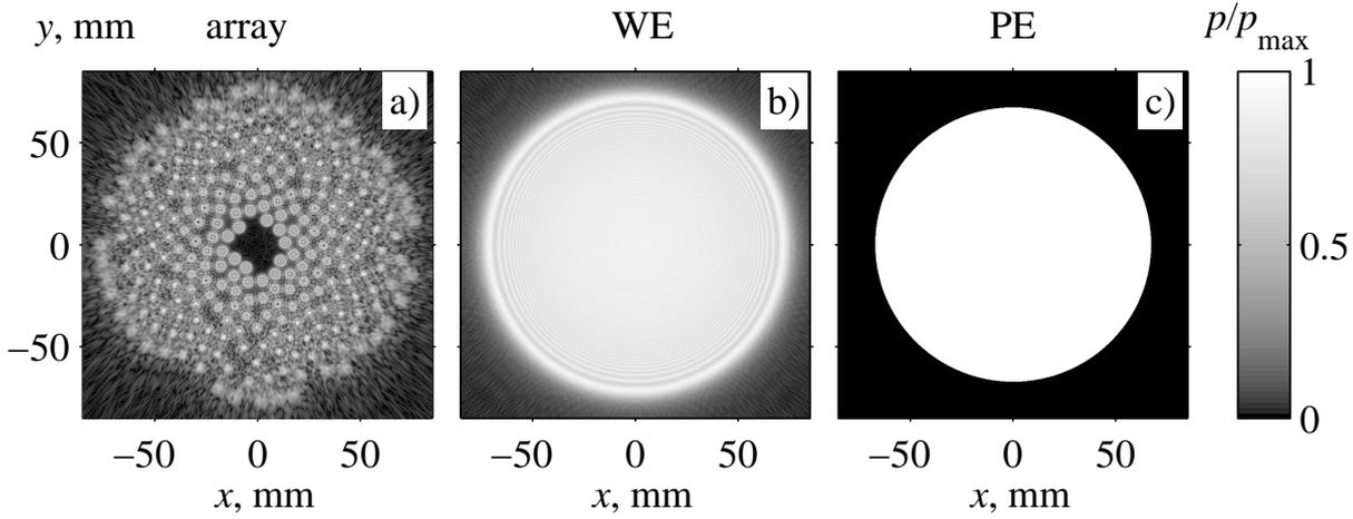
Figure 5.12: Initial pressure magnitude distributions of the array (a) and of two equivalent sources (b and c) in a plane  $z = 0$ , normalized at the maximum of the each distribution. Abbreviates explain diffraction models corresponding to the boundary conditions: WE – the Westervelt equation (b), PE – parabolic equation (c). Dimensionless pressure  $p_{\max}/p_0$  for three cases are equal to 2.34, 1.13 and 1.00, respectively.
