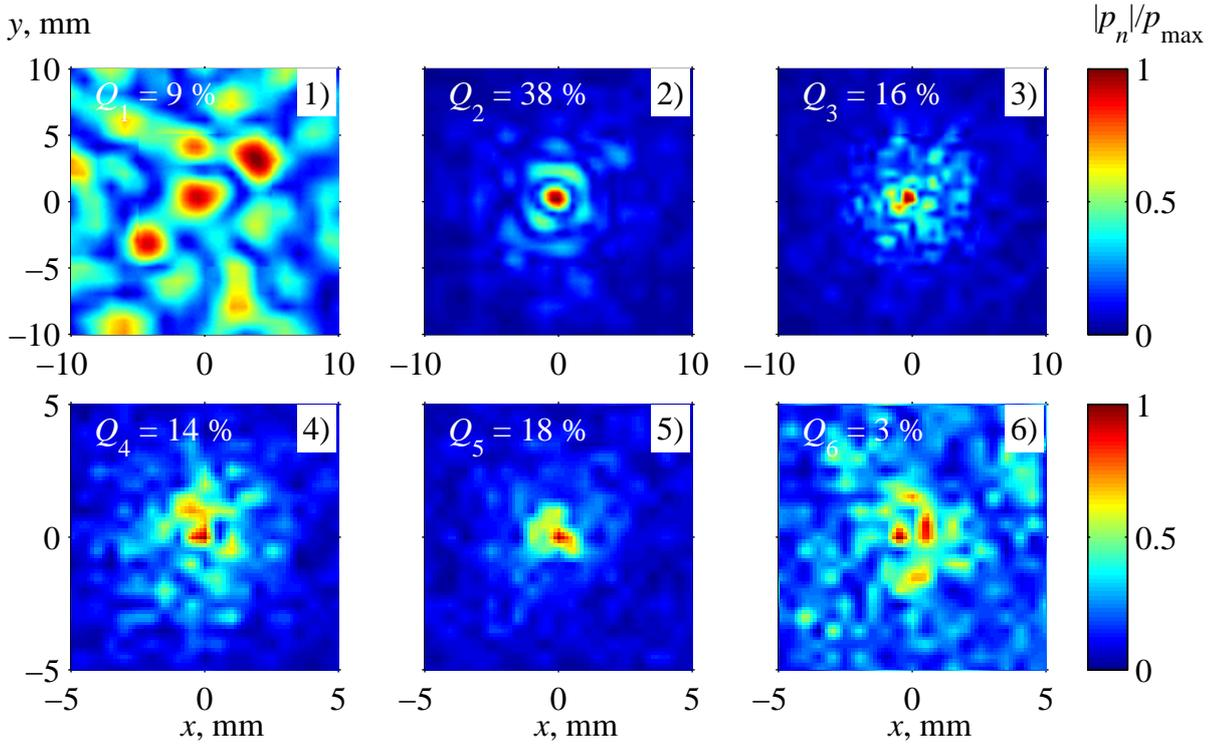
Figure 4.16: Pressure magnitudes of the first 6 harmonics measured in the focal plane (number in the corner). The  $180^\circ$  phase layer was placed at the distance from the source  $z_p = 0.5F = 36$  mm. The amplitudes are normalized on their peak values  $p_{\max}$ , equal to 450, 76, 16, 3.0, 2.5 and 0.6 kPa, respectively.
