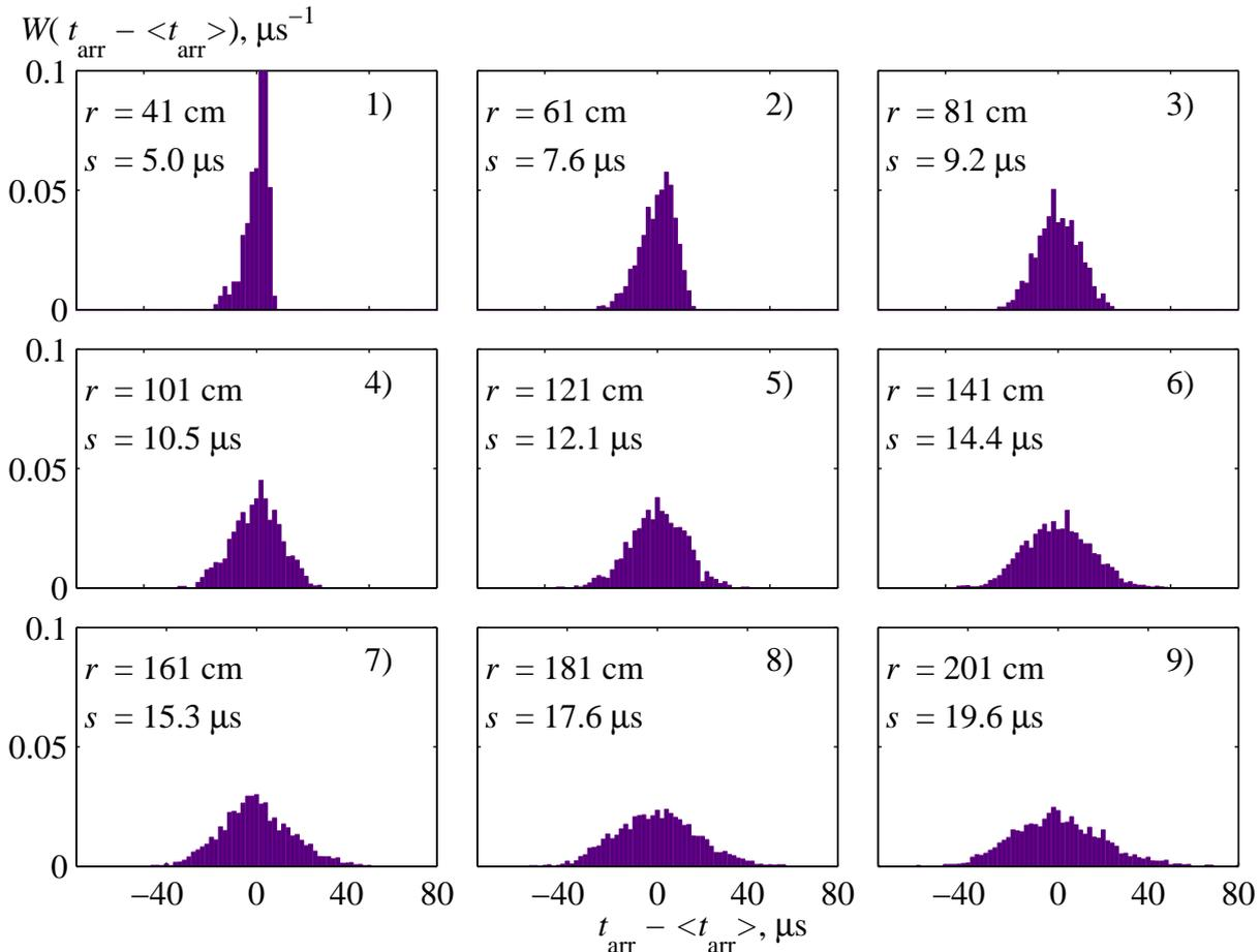
Figure 2.21: Histograms of the statistical distributions of the pulse arrival time with subtracted mean value. The data are given in microseconds. Values for the source-microphones distance  $r$  and standard deviation  $s$  are given on the graphs. Class size is  $2 \mu s$ .
