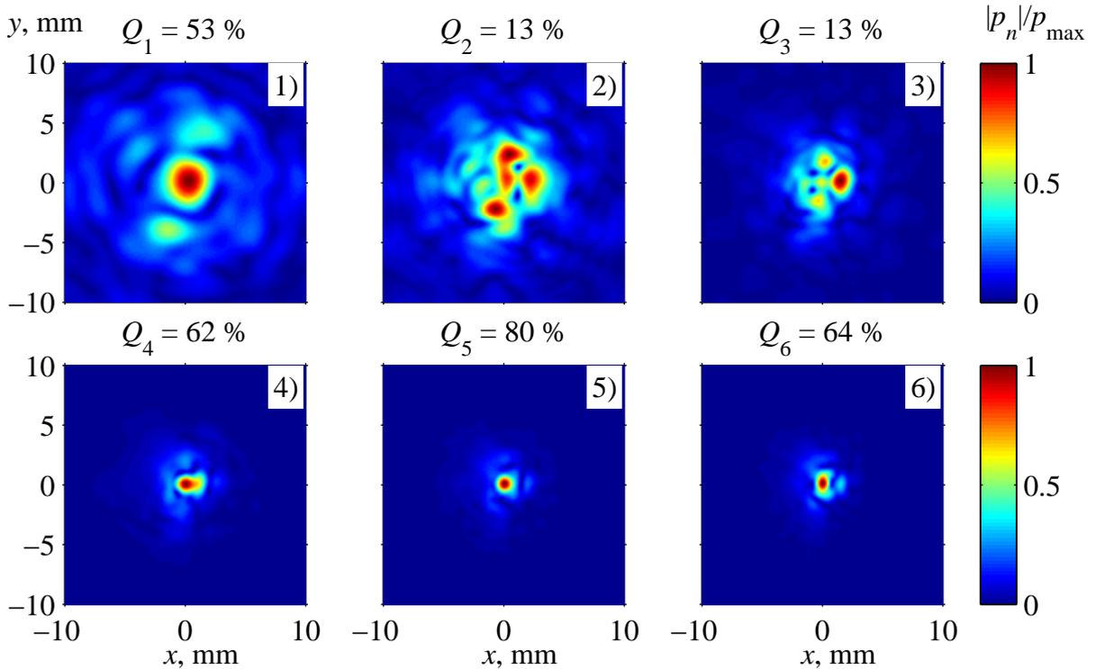
Figure 4.12: Spatial distributions of the pressure magnitude in the focal plane for the first 6 harmonics (number is given in the corner) in a case of the 90° phase layer ( $d = 3$  mm) placed at  $z_p = 0.75F = 52.5$  mm distance from the source. The focusing quality  $Q_n$  is given at the top of each image.
