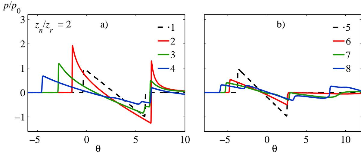
Figure 3.5:  $N$ -waveforms in the same points as shown in Fig. 3.4, but using stronger nonlinearity in calculations:  $z_n/z_r = 2$ . Nonlinear absorption and nonlinear lengthening effects are clearly seen. Fusion of two shocks into the one shock is also observed.
