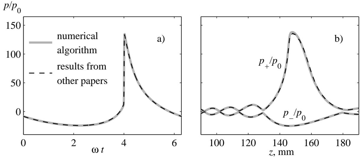
Figure 5.6: Comparison of the modeling results for nonlinear field of an axially symmetric radiator. The results were obtained in the parabolic approximation using the new algorithm (solid gray curves) and calculations performed with other algorithms (thin dashed curves): pressure waveforms at the geometric focus (a); positive  $p_+/p_0$  and  $p_-/p_0$  negative peak pressures along the beam axis (b). Nonlinear parameter  $N = 0.25$ , linear focusing gain  $G = 40$ .
