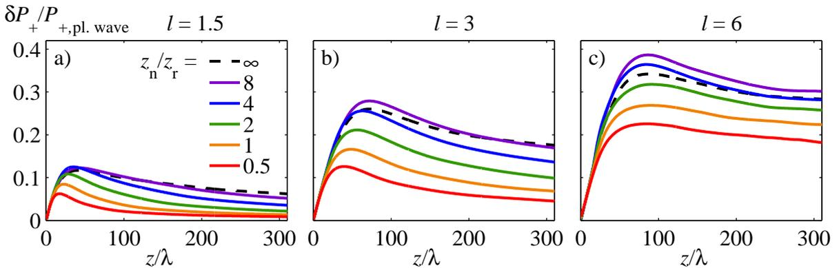
Figure 3.10: Standard deviation of peak positive pressure normalized to the plane wave amplitude as a function of propagation distance for various nonlinear lengths  $z_n$ : dashed line  $z_n/z_r = \infty$  – linear propagation, purple line  $z_n = 8z_r$ , blue line  $z_n = 4z_r$ , green line  $z_n = 2z_r$ , orange line  $z = z_r$  and red line  $z_n = 0.5z_r$ . From left to right – results for the phase screens with correlation length equal to  $l = 1.5$  (a),  $l = 3$  (b) and  $l = 6$  (c).
