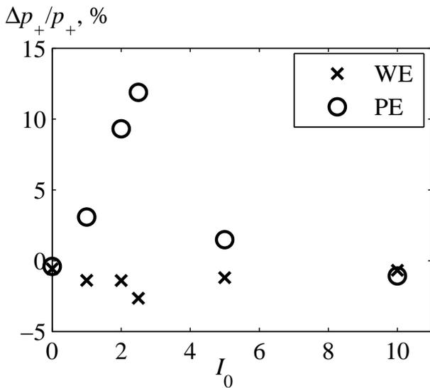
Figure 5.17: Relative difference between the peak positive pressure in the focal waveforms of the equivalent source and of the array  $[p_+(eqv.) - p_+(arr.)]/p_+(arr.)$  depending on the intensity  $I_0$ . Cross markers correspond to the axisymmetric Westervelt equation, circle markers – to the parabolic equation.
