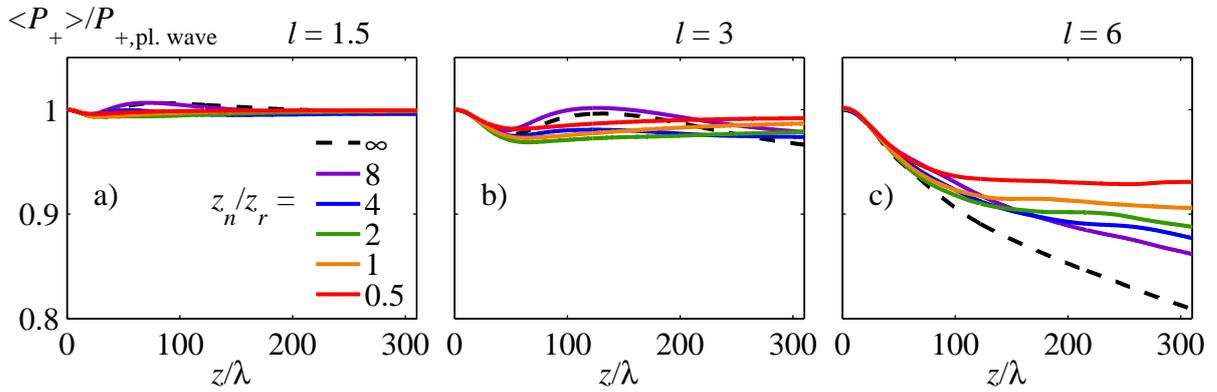
Figure 3.9: Mean peak positive pressure normalized to the plane wave amplitude as a function of propagation distance for various nonlinear lengths  $z_n$ : dashed line  $z_n/z_r = \infty$  – linear propagation, purple line  $z_n = 8z_r$ , blue line  $z_n = 4z_r$ , green line  $z_n = 2z_r$ , orange line  $z = z_r$  and red line  $z_n = 0.5z_r$ . From left to right – results for the phase screens with correlation length equal to  $l = 1.5$  (a),  $l = 3$  (b) and  $l = 6$  (c).
