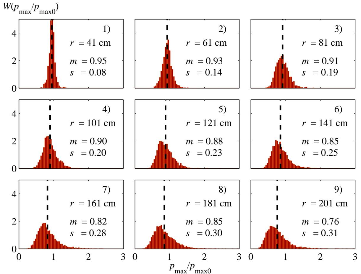
Figure 2.13: Histograms of the statistical distributions of the peak positive pressure, normalized to the corresponding values in a homogeneous medium,  $p_{\max}/p_{\max0}$ . Black dashed line shows the average value of each distribution. Values for the source-microphones distance  $r$ , the mean  $m$  and standard deviation  $s$  are given on the graphs. Class size is 0.04.
