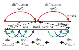
Figure 5.2: Diagram of the method of fractional steps with the operator splitting procedure over the one step  $\Delta z$ .
