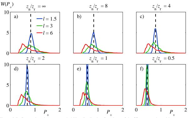
Figure 3.7: Comparison between probability distribution functions of the N-wave peak positive pressure obtained at the distance  $z = 2z_r$  for various nonlinear lengths  $z_n$ : linear (a),  $z_n = 8z_r$  (b),  $z_n = 4z_r$  (c),  $z_n = 2z_r$  (d),  $z_n = z_r$  (e) and  $z_n = 0.5z_r$  (f). Correlation lengths of the screens are: l = 6 (red curve), l = 3 (green curve), l = 1.5 (blue curve).
