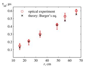
Figure 1.12: Comparison between the optically measured rise time (circles) and the rise time predicted by using the acoustic wave propagation (crosses, Eq. 1.1) at different distances from the spark source.
