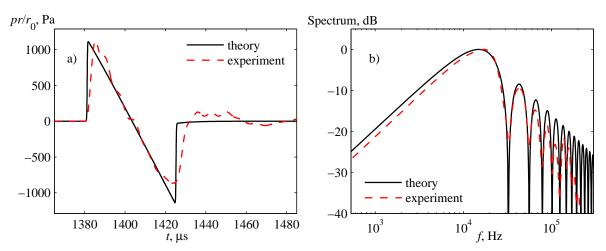
Figure 1.3: Measured (dashed) and calculated (solid) waveforms at the distance r = 49 cm from the source (a); corresponding normalized amplitude spectra (maximum at 0 dB) (b).
