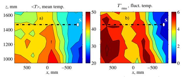
Figure 2.7: The parameters of the turbulent field in the vertical plane (x, y = -30 mm, z): the average temperature of  $\langle T \rangle$  (a), the rms fluctuation  $\Delta T_{\rm rms}$  (b). Source position is shown by with a white dot next to the letter S. Propagation path of the N-wave is marked by a thick dash-dot line.
