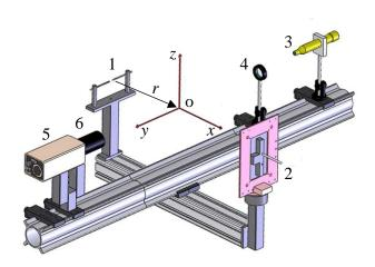
Figure 1.1: Experimental setup: 1-spark source, 2microphone in a baffle, 3-Nanolight flash lamp, 4focusing lens, 5-camera, 6-lens.
