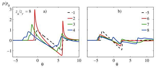
Figure 3.4: Initial and distorted N-waveforms modeled at points 1-4 and 5-8 along the horizontal dashed (a) and dash-dot (b) lines shown in Fig. 3.2b. The distances where waveforms were picked are the following: z = 0 (1 and 5),  $z = z_r$  (2 and 6),  $z = 2z_r$  (3 and 7),  $z = 4z_r$ , (4 and 8). Weak nonlinearity case is considered:  $z_n/z_r = 8$ .
