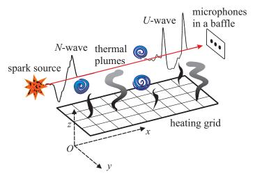
Figure 2.3: Schematic view of the experiment on the propagation of a spherical *N*-wave generated by a spark source in a thermal turbulence.
