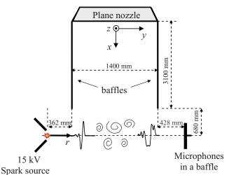
Figure 2.25: Schematic view of the experimental setup of the *N*-wave propagation experiment through kinematic turbulence.
