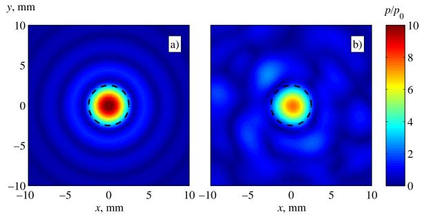
Figure 4.4: An illustration to definition of the focusing quality criterion for the first harmonic: the magnitude of the harmonic in the focal plane z = F without the phase layer in the beam path (a) and with it (b). The focal area is defined from the *undisturbed* focal distribution at the -6 dB level from its the maximum value.
