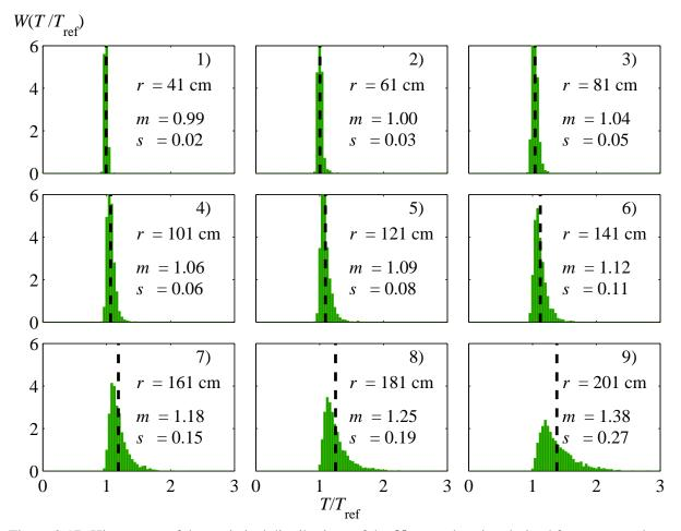
Figure 2.17: Histograms of the statistical distributions of the N-wave duration derived from temporal moments (Eq. 2.13) and normalized to the corresponding values in a homogeneous medium,  $T/T_{ref}$ . Black dashed line shows the average value of each distribution. Values for the source-microphones distance r, the mean m and standard deviation s are given on the graphs. Class size is 0.04.
