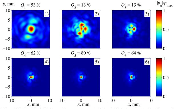
Figure 4.12: Spatial distributions of the pressure magnitude in the focal plane for the first 6 harmonics (number is given in the corner) in a case of the 90° phase layer (d = 3 mm) placed at  $z_p = 0.75F = 52.5$  mm distance from the source. The focusing quality  $Q_n$  is given at the top of each image.
