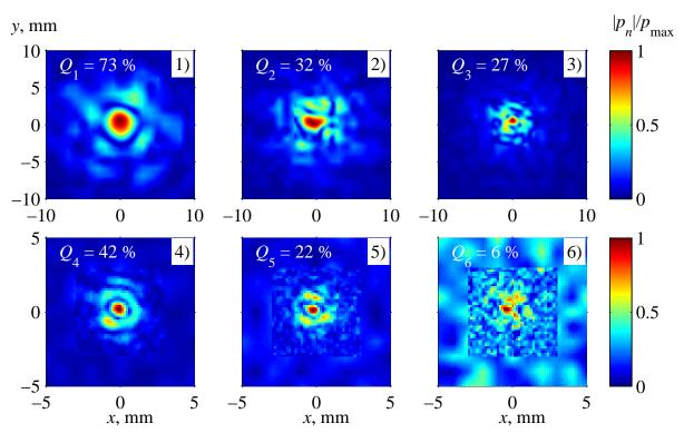
Figure 4.18: Pressure magnitudes of the first 6 harmonics in the focal plane (number in the corner), measured in a case of the 90° phase layer. The layer was placed at the distance from the source  $z_p = 0.71F = 51$  mm. The amplitudes are normalized on their peak values  $p_{\text{max}}$ , equal to 1260, 100, 26, 9.3, 3.6 and 1.4 kPa, respectively.
