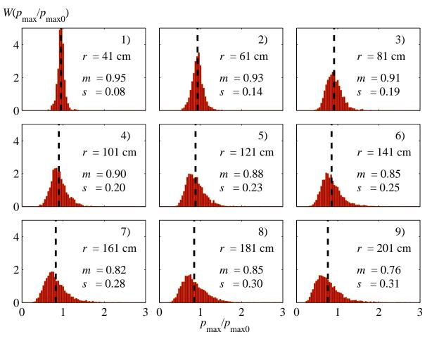
Figure 2.13: Histograms of the statistical distributions of the peak positive pressure, normalized to the corresponding values in a homogeneous medium,  $p_{\text{max}}/p_{\text{max}0}$ . Black dashed line shows the average value of each distribution. Values for the source-microphones distance r, the mean m and standard deviation s are given on the graphs. Class size is 0.04.
