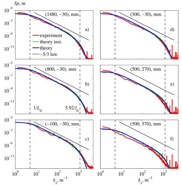
Figure 2.10: One-dimensional spectra of fluctuations of the refractive index obtained experimentally (red line) and by the von Karman model spectrum with the parameters of  $L_0 = 20$  cm,  $l_0 = 5$  mm (blue line). The green line shows a spectrum obtained by processing the artificial realization with the von Kármán spectrum using the same methodology (see Appenix. C), as in the processing of experimental spectra. Black line corresponds to the law  $k^{-5/3}$ .
