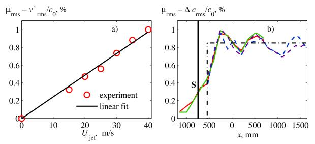
Figure 2.24: The rms fluctuations of the refraction index measured in the experiment with the jet (Fig. 2.23a,  $U_{jet}$  is flow velocity at the exit of the jet) and along the *N*-wave propagation path in the experiment with heating grid (Fig. 2.23b).
