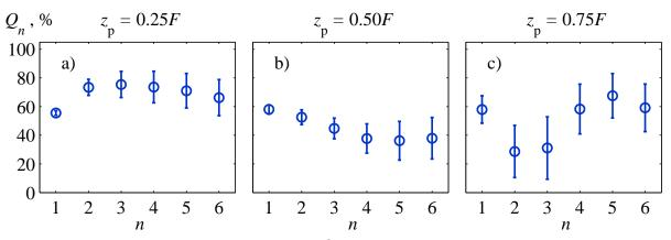
Figure 4.11: Mean values of the focusing quality  $Q_n$  for the first 6 harmonics in a case of the 90° phase layer placed at distances  $z_p = 0.25F$  (a),  $z_p = 0.50F$  (b), and  $z_p = 0.75F$  (c) from the source. Averaging was done using 10 realizations, error bars correspond to standard deviations.
