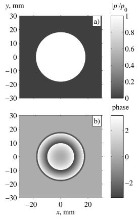
Figure 4.2: The pressure magnitude in the plane z = 0 in the case of circular focused piston.
