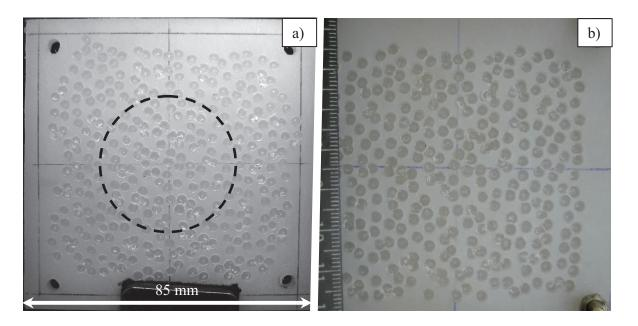
Figure 4.14: Images of the  $90^{\circ}$  – (a) and the  $180^{\circ}$  – (b) phase layers fabricated from low-density polyethylene. The dashed circle indicates the diameter of the source.
