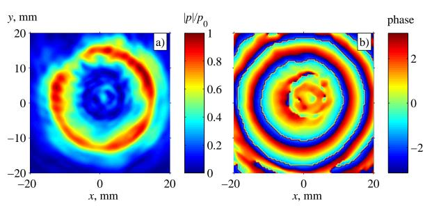
Figure 4.3: The amplitude (a) and phase (b) in the source plane z = 0 mm, obtained using the acoustic holography method.
