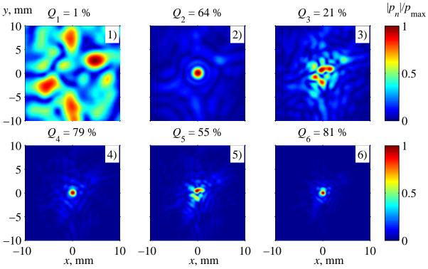
Figure 4.8: Spatial distributions of the pressure magnitude of the first 6 harmonics (number in the corner) in case of the 180° phase layer (d = 3 mm) placed at  $z_p = 0.5F = 35 \text{ mm}$  distance from the source. The focusing quality  $Q_n$  is given at the top of each image. The characteristic feature of the example is low focusing quality of the odd harmonics and high quality of even harmonics.
