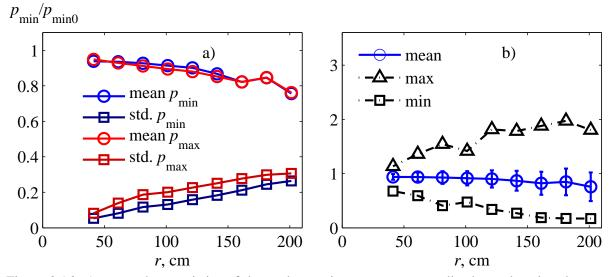
Figure 2.16: Average characteristics of the peak negative pressure, normalized to values in a homogeneous medium  $p_{\min}/p_{\min 0}$ . The graph shows the mean value (blue line, circle markers) and the standard deviation (blue line, square markers) (a), as well as maximum (triangle markers) and minimum (square markers) values observed in the sample (b). The comparison with normalized peak positive which data are shown by red line is also provided.
