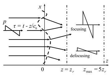
Figure 3.1: Propagation of initially plane N-wave through infinitely thin phase screen (dashed line) located at z = 0. Arrows illustrate focusing and defocusing effects behind the screen. The refraction length is denoted as  $z_r$ , maximum propagation distance in numerical simulations is  $z_{\text{max}} = 5z_r$ .
