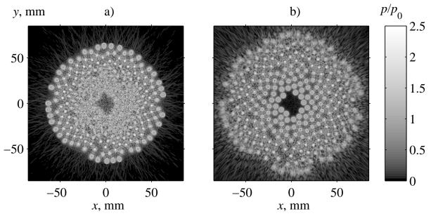
Figure 5.1: Spatial distributions of dimensionless pressure amplitude  $p/p_0$  calculated in a plane (x, y, z = 20 mm) near the edge of the radiator (a) and in a plane (x, y, z = 0 mm) – "virtual" source (b). Here,  $p_0 = \rho_0 c_0 u_0$ , where  $u_0$  is the amplitude of the vibration velocity at the surface of the array element.
