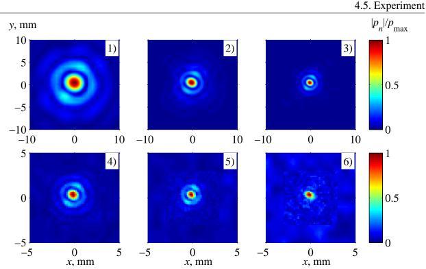
Figure 4.15: Pressure magnitudes of the first 6 harmonics in the focal plane (the number is in the corner), measured without the phase layer. The amplitudes are normalized on their peak values  $p_{\text{max}}$ , equal to 2000, 420, 150, 55, 28 and 14 kPa, respectively.
