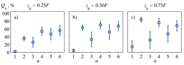
Figure 4.9: Mean values of the focusing quality  $Q_n$  for the first 6 harmonics in a case of the 180° phase layer placed at distances  $z_p = 0.25F$  (a),  $z_p = 0.50F$  (b), and  $z_p = 0.75F$  (c) from the source. Averaging was done using 10 realizations, error bars correspond to standard deviations.
