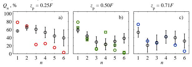
Figure 4.19: Comparison of the focusing quality criterion  $Q_n$  for the first six harmonics with the 90° phase layer placed at the distances  $z_p = 0.25F = 18 \text{ mm}$  (a),  $z_p = 0.50F = 36 \text{ mm}$  (b) and  $z_p = 0.71F = 51 \text{ mm}$  (c): experimental data (color markers) and simulations results (black markers). Different type of the color markers correspond to different realizations of the phase layer obtained by moving it parallel in its own plane.
