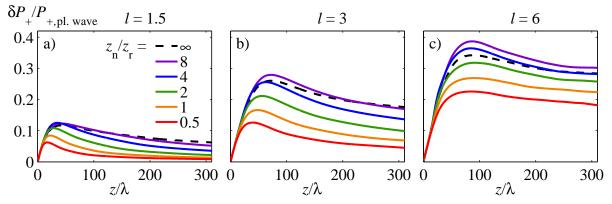
Figure 3.10: Standard deviation of peak positive pressure normalized to the plane wave amplitude as a function of propagation distance for various nonlinear lengths  $z_n$ : dashed line  $z_n/z_r = \infty$  – linear propagation, purple line  $z_n = 8z_r$ , blue line  $z_n = 4z_r$ , green line  $z_n = 2z_r$ , orange line  $z = z_r$  and red line  $z_n = 0.5z_r$ . From left to right – results for the phase screens with correlation length equal to l = 1.5 (a), l = 3 (b) and l = 6 (c).
