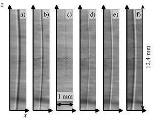
Figure 1.5: Positions of the camera observation plane along the y axis that correspond to the shadowgrams given in Fig. 1.6: 32 mm (a), 12 mm (b), 2 mm (c), -4 mm (d), -13 mm (e), and -24 mm (f). Shock wavefront is plotted schematically as a red solid curve.
