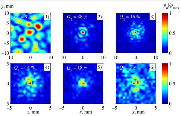
Figure 4.16: Pressure magnitudes of the first 6 harmonics measured in the focal plane (number in the corner). The 180° phase layer was placed at the distance from the source  $z_p = 0.5F = 36$  mm. The amplitudes are normalized on their peak values  $p_{\text{max}}$ , equal to 450, 76, 16, 3.0, 2.5 and 0.6 kPa, respectively.
