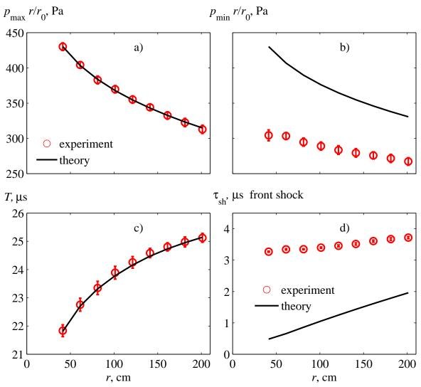
Figure 2.11: Main parameters of the N-wave, measured in a homogeneous air. The positive peak pressure (a), the negative peak pressure (b), half-duration (c), the front shock risetime (d). Black line shows the results of numerical simulation, red markers – the results of the experiment. Atmospheric conditions were the following:  $p_{\rm atm} = 97900$  Pa,  $T_{\rm atm} = 14.5$  °C, humidity 35%.
