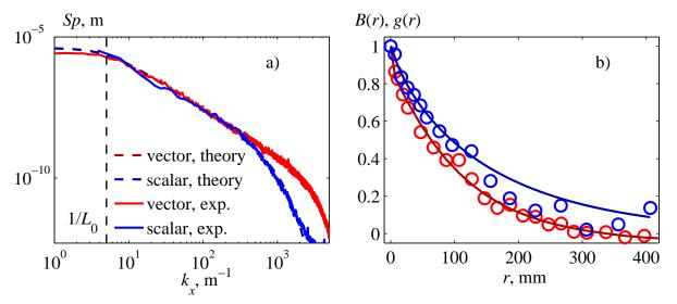
Figure 2.26: Comparison of one-dimensional spectra of vector (red lines) and scalar turbulence (blue lines) (a). Measured spectra are shown by solid lines, and theoretical by dashed lines. Spectrum of kinematic turbulence is normalized to have the same rms as the spectrum of thermal turbulence. Comparison of transversal correlation function of kinematic turbulence with correlation function of thermal turbulence (b).
