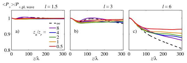
Figure 3.9: Mean peak positive pressure normalized to the plane wave amplitude as a function of propagation distance for various nonlinear lengths  $z_n$ : dashed line  $z_n/z_r = \infty$  – linear propagation, purple line  $z_n = 8z_r$ , blue line  $z_n = 4z_r$ , green line  $z_n = 2z_r$ , orange line  $z = z_r$  and red line  $z_n = 0.5z_r$ . From left to right – results for the phase screens with correlation length equal to l = 1.5 (a), l = 3 (b) and l = 6 (c).
