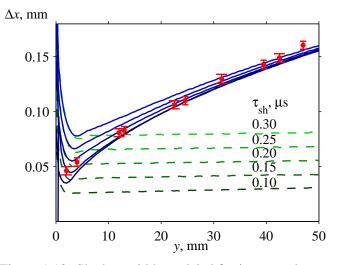
Figure 1.10: Shadow width modeled for images taken at different positions y of the camera focus. Dashed curves are obtained using the geometrical optics model and solid curves - using the parabolic equation. The change of the contrast in both sets of curves from dark to light corresponds to increasing shock rise time in the modeling. Points with vertical bars are shadow widths and corresponding standard deviations measured from experimental shadowgrams.
