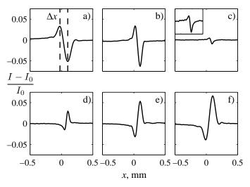
Figure 1.7: Normalized intensity distributions  $(I-I_0)/I_0$ along the *x*-axis obtained from shadowgrams given in Fig. 1.6.  $I_0$  is the background intensity. In the subplot (c) a zoom is plotted.
