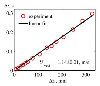
Figure 2.8: Determination of the average lifting speed of the turbulent structures  $U_{\text{vert}}$  using dependence of the time shifting interval between the two signals of the probes, at which the maximum correlation is reached, from the distance between them. Measurements were made at the point (175, -30, 1644) mm. The experiment – red circular markers, linear approximation  $\Delta z = U_{\text{vert}}\Delta t$  – black line.
