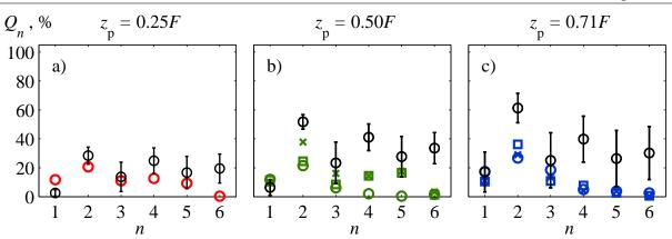
Figure 4.17: Comparison of the focusing quality criterion  $Q_n$  for the first six harmonics with the 180° phase layer placed at the distances  $z_p = 0.25F = 18 \text{ mm}$  (a),  $z_p = 0.50F = 36 \text{ mm}$  (b) and  $z_p = 0.71F = 51 \text{ mm}$  (c): experimental data (color markers) and simulations results (black markers). Different type of the color markers corresponds to different realizations of the phase layer obtained by moving it parallel in the (x, y) plane.
