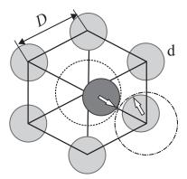
Figure 4.6: The method of random displacement of the circles to produce negligible overlap.
