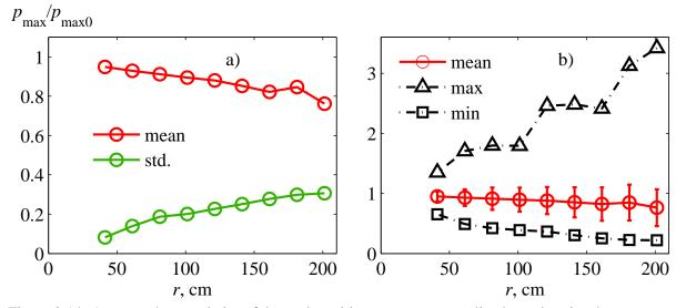
Figure 2.14: Average characteristics of the peak positive pressure, normalized to values in a homogeneous medium  $p_{\text{max}}/p_{\text{max}0}$ . The graph shows the mean value (red line) and the standard deviation (green line) (a), as well as maximum (triangle markers) and minimum (square markers) values observed in the sample (b).
