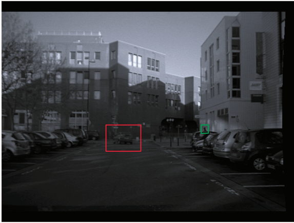
Fig. 6. Image extracted from a real test sequence. The vehicle within the red bounding box is driving forward and initiating a left bend. Within the green box lies the head of a partially occluded pedestrian walking from the right hand side of the field, toward the left-hand side.
