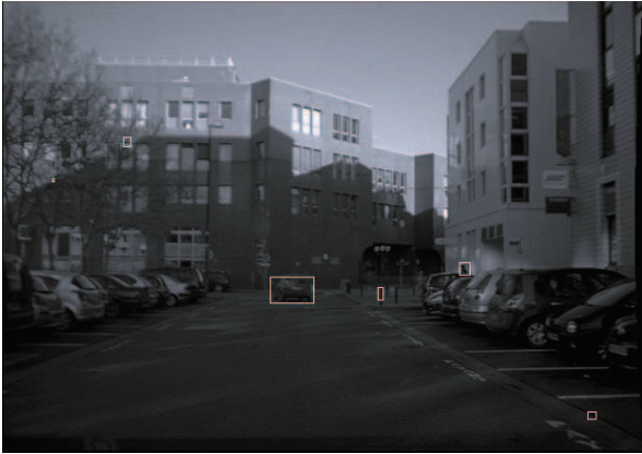
Fig. 9. Final Segmentation Realized. One can note the extraction of the road post, as well as two small false positives. Those false positives are due to false correlations. The targets, however are well defined.
