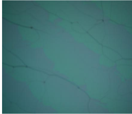
FIGURE 2- 6: GRANDJEAN STRUCTURE IN CHOLESTERIC WITH OILY STREAKS
