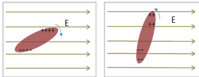
Figure 1- 12: RESPONSE TO ELECTRIC FIELD BY POSITIVE AND NEGATIVE ANISOTROPIC LIQUID CRYSTAL
