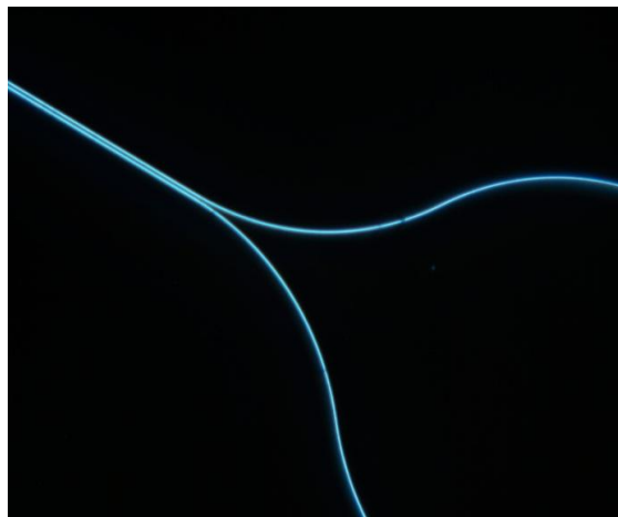
Figure 6- 10: Waveguide with two branches which separate the polarisations
