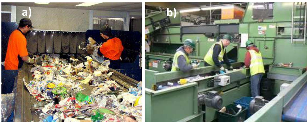
Figure 3. a) Pre-manual sorting to remove big contaminants. b) Manual plastic sorting.
