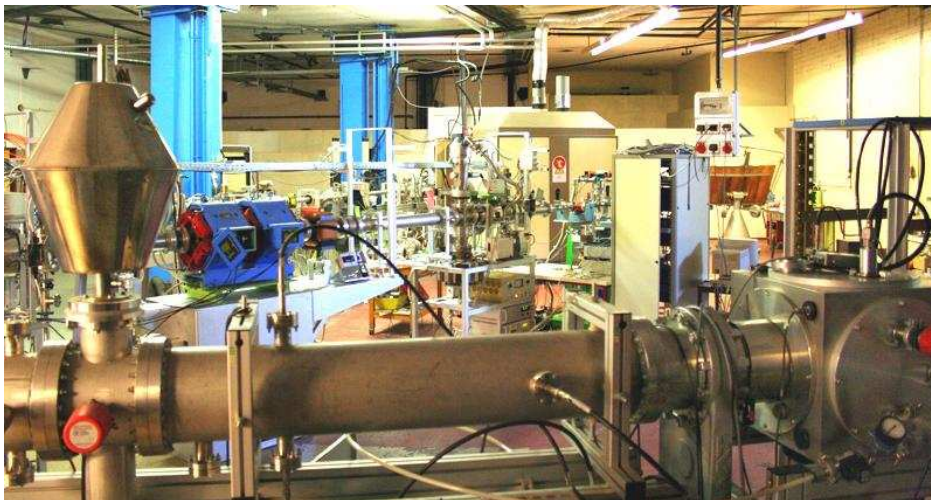
Fig. 3.1. Implanter EATON 200 kV used at InESS.
