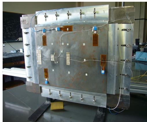
Figure 4.5: Energy source structure: A cantilever beam. Figure 4.6: Energy target structure: A four edge clamped plate.
