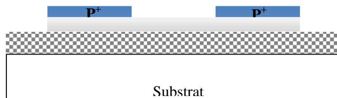
Figure 38. Isolation des transistors.
