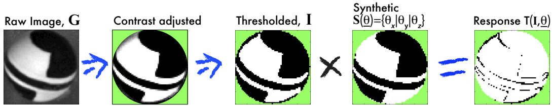
Figure 3.9: Texture extraction and comparison with a synthetic image. The resemblance between the image \underline{\mathbf{I}} and the synthetic projection \underline{\mathbf{S}} at angle \underline{\theta} is estimated using Eq. (3.13).
