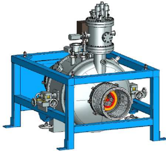
Figure 5.12: Drawing of the ground Calibration Light Source. In the lightbox on the top, a filament lamp provides the source spectrum, which is altered by passing through four filter wheels. The lightbox output enters the large integrating sphere, whose exit port can be seen at the front (orange). The aperture has a mask mimicking the JWST OTE pupil (red). (Credit: MSSL)
