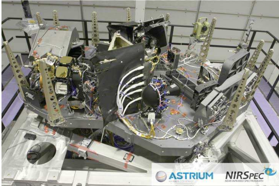
Figure 1.6: Fully assembled NIRSpec flight model 1 without the instrument cover (credit: EADS/Astrium).
