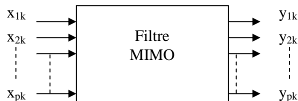
figure IV.5.b - Filtre MIMO (Multiple Input Multiple Output)
