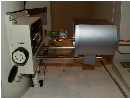
Fig. 2.9 – Sample introduction in the SEM setup
