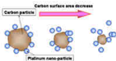
Figure 7. (Color online) Cathodic CO 2 -driven Pt coarsening mechanism.
