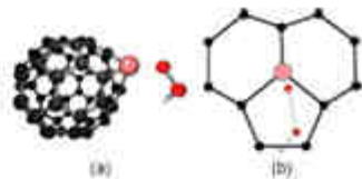
Fig. 7 OOH on CuPt. This molecule is on top of the Pt and will tend to block catalytic activity. It is also a rather bulky molecule and blocks the 5-membered ring. The colors and projection method are the same as in Fig. 3. Oxygen is shown in medium gray.
