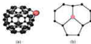
Fig. 2 C_{60}Pt , where (a) is a side view of the Pt which shows how the metallofullerene is 'puckered', and (b) is a projection of the front view and only includes the structure immediately around the gray platinum atom. The platinum is at the corner of two 6-membered rings and one 5-membered ring.
