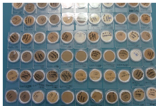
Filters after filtration
