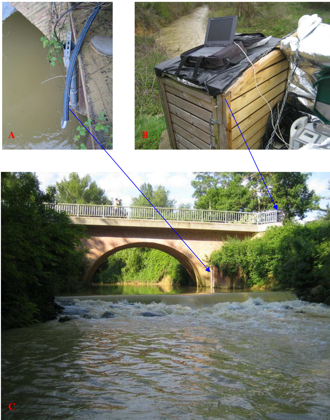
Figure 3-6: Schema of installing water quality monitoring system at Larra station: A) pump inlet and Sonde pipe, B) Automatic Water Sampler EcoTech, C) Sampling site at Larra bridge
