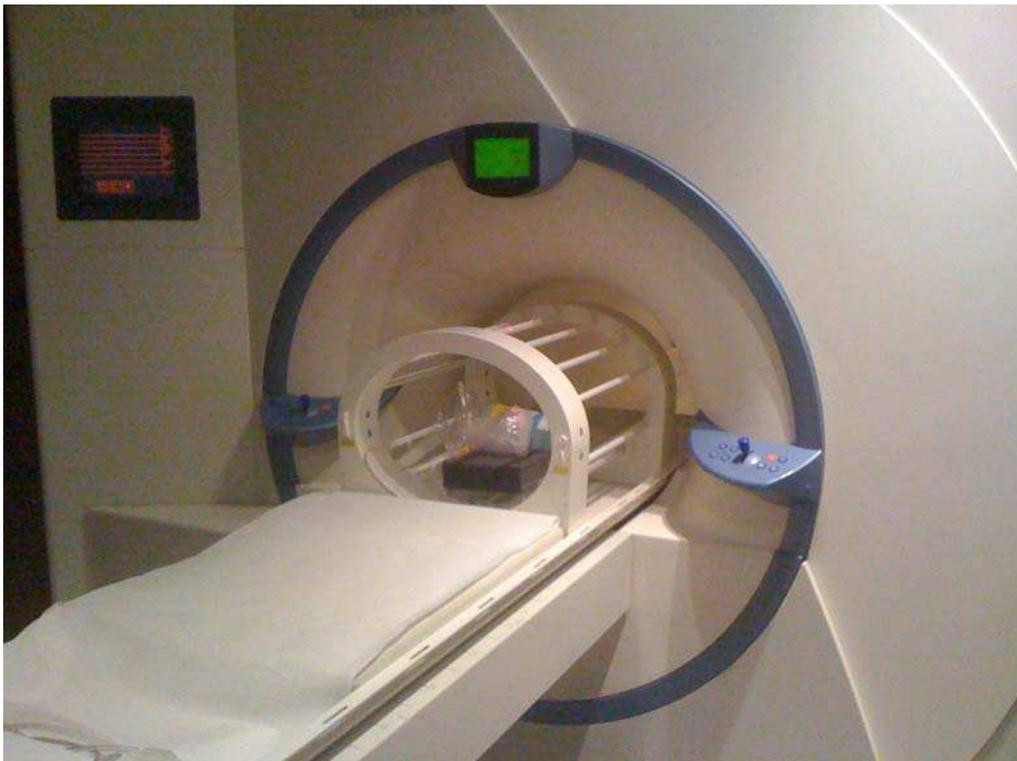
Fig. 2.10. Sonata scanner in John Paul 2<sup>nd</sup> Hospital with <sup>3</sup>He coil from RAPID Biomedical. In the center of the coil, a first phantom (see text) is placed for angle calibration experiment.
