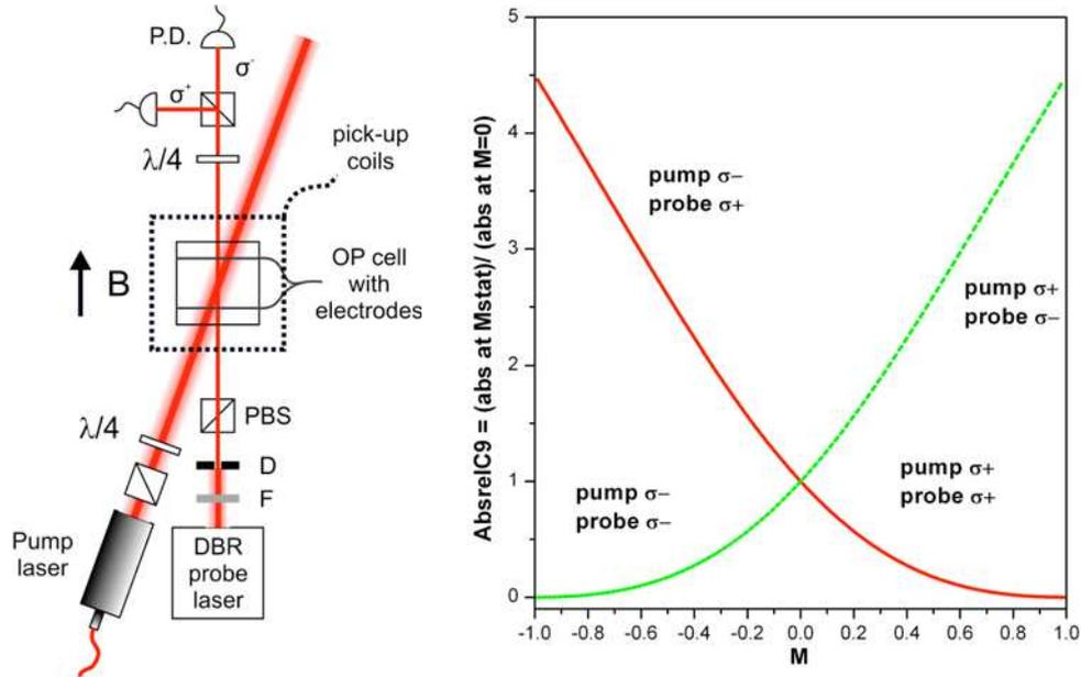
Fig. 2.8. Left: Schematic of the optical setup used for NMR calibration, see text (P.D.: Photodiode, PBS: Polarizing Beam Splitter, D: Diaphragm, F: Filter,  $\lambda/4$ : quarterwave plate). Right: relative  $\sigma^+$  and  $\sigma^-$  absorbances of a weak probe laser beam tuned on  $C_9$  line as a function of the nuclear polarization  $M$ .
