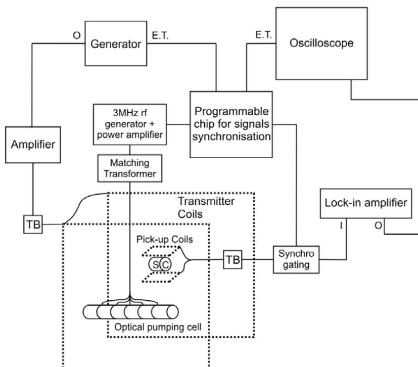
Fig. 2.7. Scheme of the NMR acquisition (see text). (TB: Tuning and matching circuit, I: Input, O: Output, S.C.: Storage Cell, E.T.: External Trigger). A microprocessor at the center of the NMR system is used to control the different elements.
