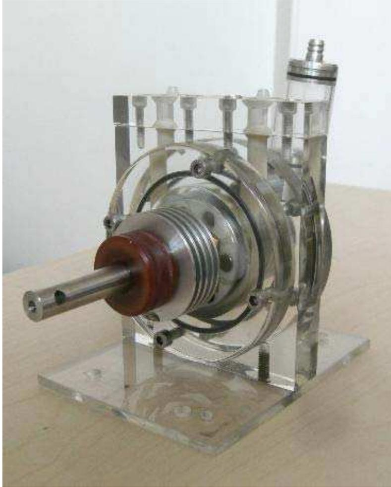
Fig. 2.6. Picture of the new peristaltic compressor design.
