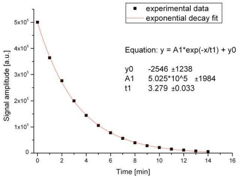
Fig. 2.4. Relaxation of magnetization inside a 12 mL polypropylene/polyethylene syringe in our 0.088T permanent magnet. Plastic syringe was used to transport polarized  $^3\text{He}$  from the storage cell to the scanner and to inflate lungs of the tracheotomised rat. Time before application was reduced as much as possible and kept below 20 s, which is equivalent to a total magnetization loss lower than 10 %.
