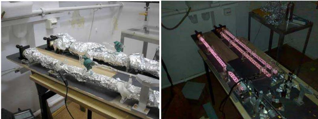
Fig. 4.12. Cleaning process of the OP cells. Left: A heating tape ( $100^{\circ}\text{C}$ ) was wired around each cell while a vacuum was produced by a TMP. The aluminium foil visible on the picture keeps the heat close to the glass. Right: Plasma discharge with 20 mbar of  $^4\text{He}$ . The shape of the plasma is made of rings close to each electrode.
