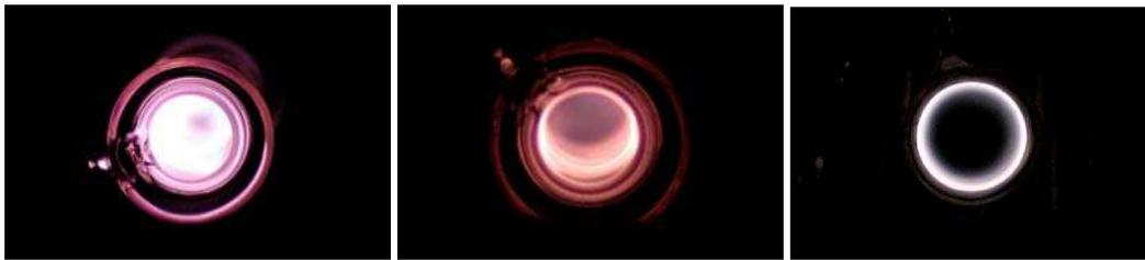
Fig. 4.3. Pictures of the plasma inside sealed cells (diameter 14 mm) at 1.33 mbar (left), 32 mbar (center) and open cell (diameter 31 mm) at 18 mbar (right) after conscientious cleaning process consisting of rinsing several times the cell with high plasma discharges in  $^4\text{He}$ .
