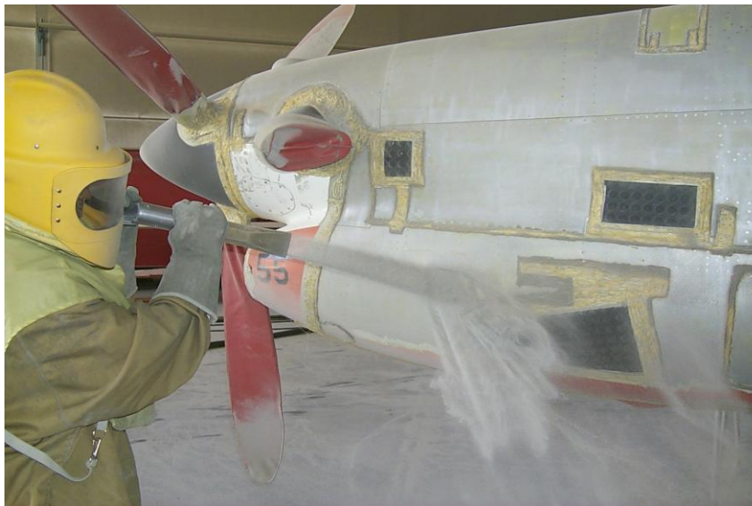
Figure 4. Fuselage stripping of T-25 aircraft at PAMA-LS.
