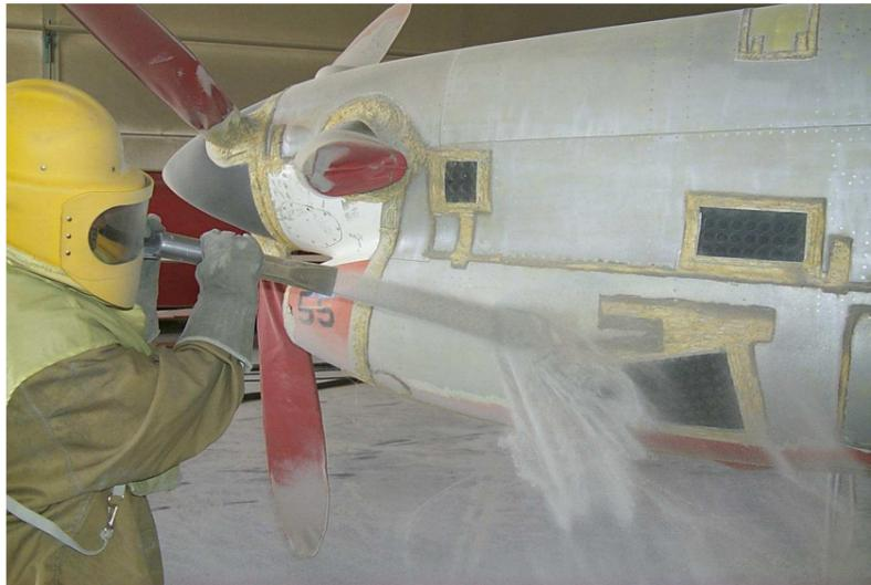
**Figure 4.** Fuselage stripping of T-25 aircraft at PAMA-LS.
