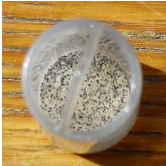
Figure 5.12: Photograph of LMO sample when attempt to be reduce in Ar + 10% H 2 with 60 ml/min flow rate in a quartz crucible. Black spots in a white matrix can be seen.
