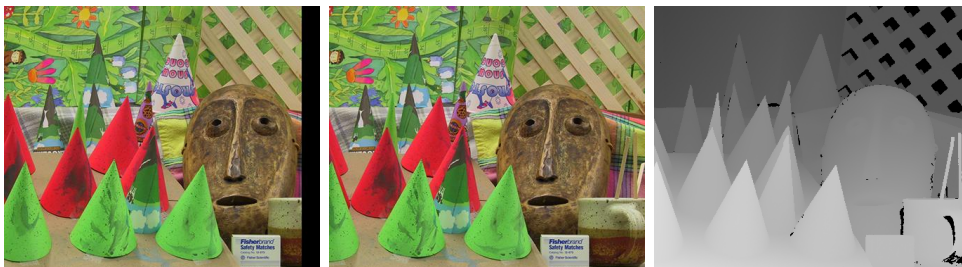
Figure 2.4: Disparity of rectified images. The third image displays the disparity measure of the second image with the first one.
