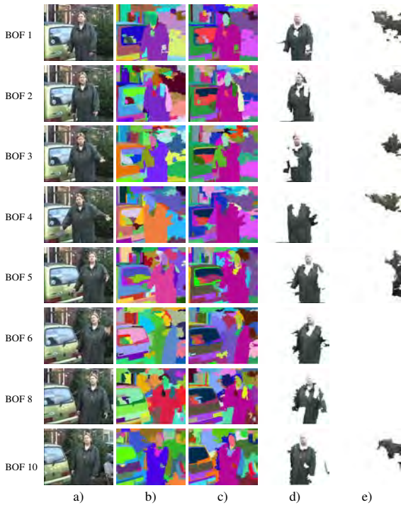
Fig. 6. Video semantic segmentation. (a) Frames in various BOF. (b) Spatiotemporal segmentation. (c) Semantic segmentation and inter-BOF matching. (d) Concept "person". (e) "foliage".
