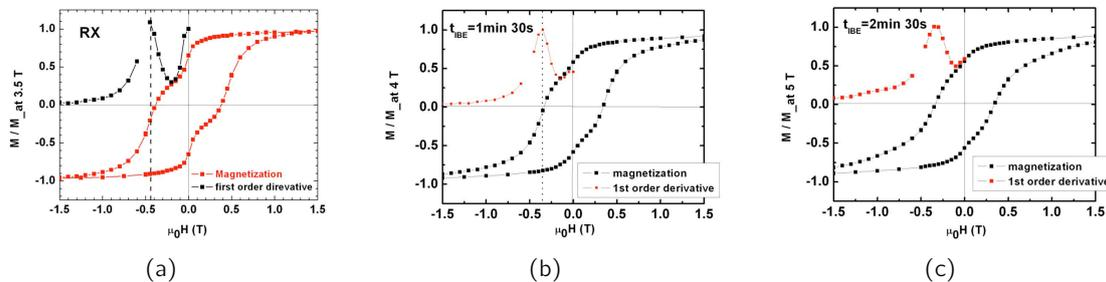
**Fig. 3.14:** Magnetic properties of patterned NdFeB layers: (a) Two-phase characteristic of the hysteresis loop after patterning of the NdFeB layer; (b) Partial removal of the soft phase on top of the magnetic layer after an ion beam etching step for 1'30" and annealing at 610°C; (c) Complete removal of the soft phase on top of the magnetic layer after an ion beam etching step for 2'30" and annealing at 610°C.
