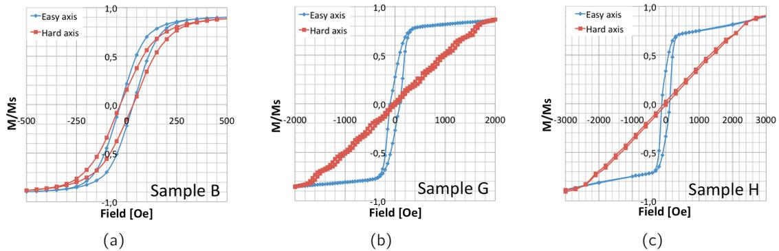
**Fig. 3.24:** Evolution of shape anisotropy depending on stripe width (before annealing): (a) weak shape anisotropy for sample B ( $w = 4\mu\text{m}$ ); (b) clear presence of magnetic easy- and hard axis for sample G ( $w = 0.5\mu\text{m}$ ); (c) the highest shape anisotropy is observed for sample H ( $w = 0.25\mu\text{m}$ ).
