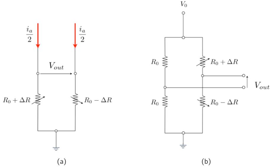
**Fig. 2.11:** Two different configurations for signal readout: (a) constant current supply; (b) constant voltage supply.
