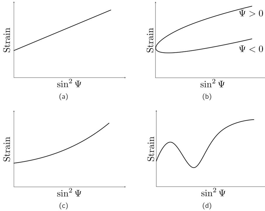
**Fig. 4.12:** Dependencies of strain on  $\sin^2 \Psi$ : (a) linear dependence for stress perpendicular to the plane; (b) splitting of the curve for the case of shear stresses; (c) presence of a stress gradient perpendicular to the surface; (d) large stress variations; equation 4.4 is not applicable in this case [101].
