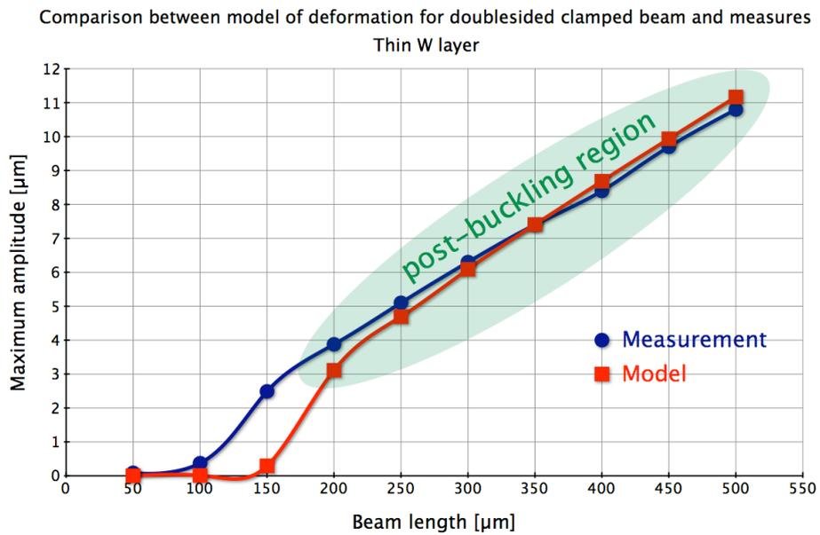
**Fig. 4.25:** Fitting of the measurements to the model shown by the example of a thin W layer. The fit was applied exclusively in the post-buckling region.
