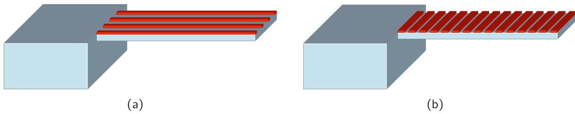
**Fig. 4.26:** Two different layer patterns: (a) lengthwise split; (b) lateral split. The drawing shows the case where the stressed layer is situated on top of the substrate. The integration of the stressed layer into the substrate was studied in the same way.
