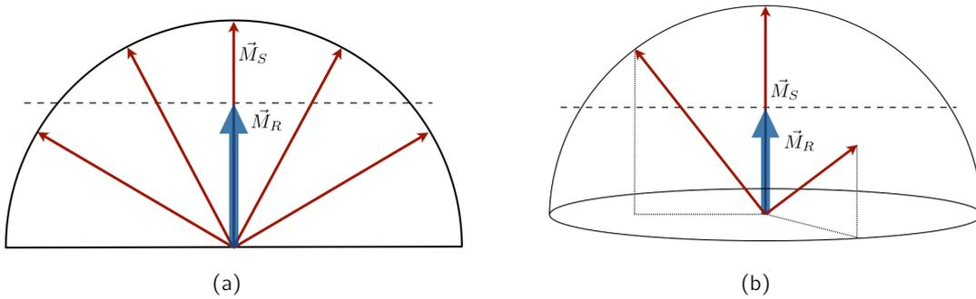
**Fig. 3.6:** Influence of magnetocrystalline anisotropy on remanence: (a) Remanence is reduced by a factor  $2/\pi$  in case of in-plane magnetization of amorphous magnetic material; (b) Remanence is reduced by a factor 0.5 for amorphous magnetic material without effects of shape anisotropy.
