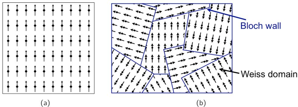
**Fig. 3.4:** Ferromagnetism: (a) In ferromagnetic materials, dipole moments are aligned and stabilized by the exchange interaction; (b) Separation of magnetic domains ("Weiss domains") in a ferromagnet by transition regions ("Bloch walls").
