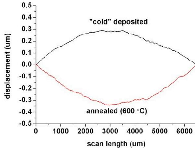
**Fig. 4.16:** Stress measurements for a  $1\mu\text{m}$  thick NdFeB layer before and after annealing. Downward bending indicates compressive residual stress, upward bending indicates tensile residual stress.
