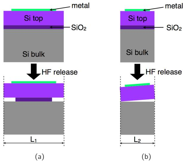
**Fig. 2.29:** Influence of the conducting path's line width on its mechanical stability: (a) sufficient line width  $L_1$  to assure stability of the conductor path after HF release; (b) loss of electrical contacts for narrow line width  $L_2$  due to complete removal of the sacrificial SiO<sub>2</sub> layer.
