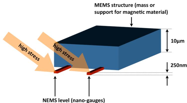
**Fig. 2.1:** M&NEMS concept: a relatively thick (10 μm) MEMS structure is connected to a piezoresistive strain-gauge with nanometric section. A displacement of the MEMS structure deforms the nano-gauges and induces high mechanical stresses.
