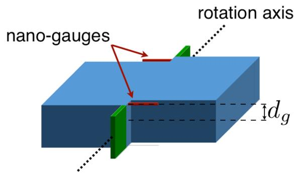
**Fig. 2.33:** Example for a torsion beam hinge
