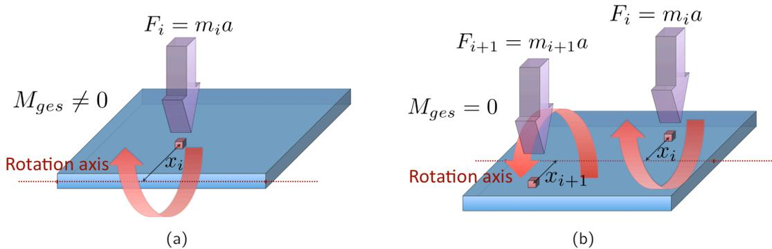
**Fig. 2.26:** Impact of acceleration on the sensor's Silicon mass: (a) resulting moment for unbalanced structures; (b) the moment vanishes for balanced structures.
