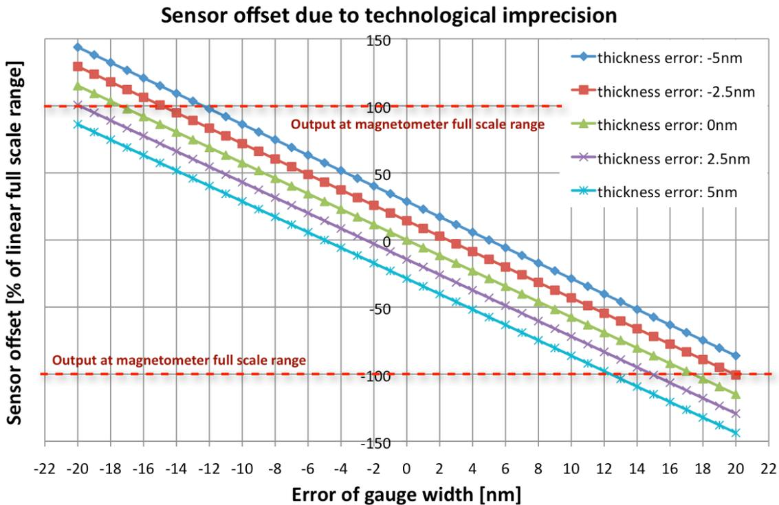
**Fig. 2.40:** Maximum possible sensor offsets for different deviations from nominal gauge width and nominal gauge thickness, calculated for a polarization current of  $100\mu\text{A}$ , a silicon resistivity of  $2.3 \times 10^{-5}\Omega\text{m}$  and nominal gauge dimensions of  $0.25 \times 0.25 \times 5\mu\text{m}^3$ . Offset values can even reach the level of the output signal at full scale which is reached for a gauge stress of  $100\text{MPa}$ .
