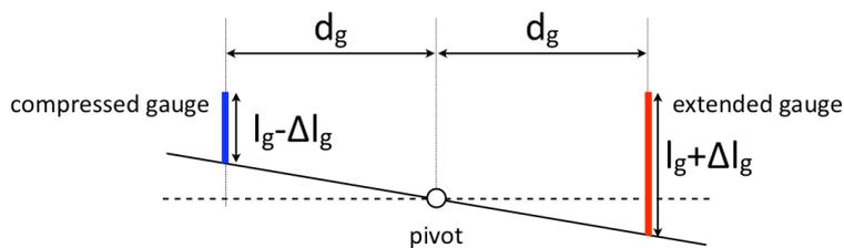
**Fig. 2.41:** Geometrical configuration of nano-gauges
