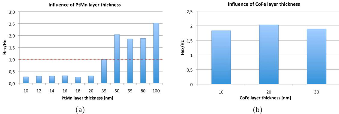
**Fig. 3.28:** Influence of layer thickness variation on  $H_{ex}/H_c$  ratio in case of full-sheet deposition of AF/F stacks: (a) different PtMn layer thicknesses for a fixed CoFe layer thickness of 20nm; (b) different CoFe layer thicknesses at a fixed PtMn layer thickness of 50nm.
