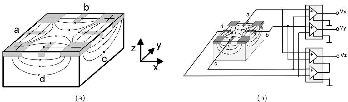
**Fig. 1.11:** Principle of a 3D Hall according to Schott and Popovic [11]: (a) The 3D sensor is a low doped Silicon block with 8 ohmic contacts at its surface. Current is injected in the four corners and sensing is achieved by the contacts a,b,c and d; (b) Simultaneous sensing of the three magnetic field components.
