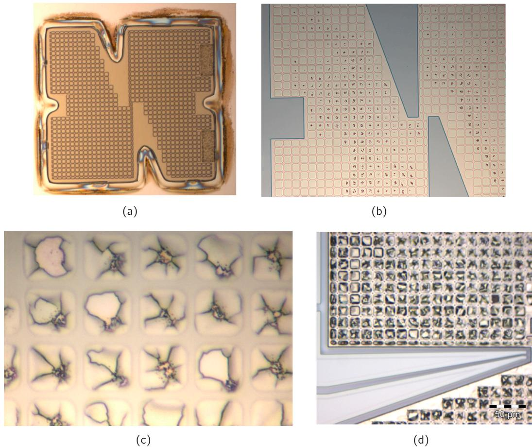
**Fig. 4.7:** Problems with integration of NdFeB in the magnetometer demonstrator: (a) No visible defects after patterning of the NdFeB layer; (b) brittle  $W_2N$  capping layer; (c) after deposition and stripping of an AlSi layer for electrical contacts; (d) after HF vapor release.
