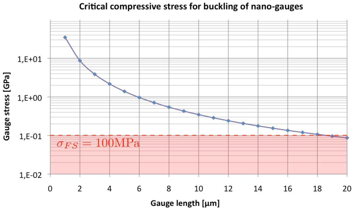
**Fig. 2.17:** Critical stress where Euler buckling of nano-gauges appears for different gauge lengths.
