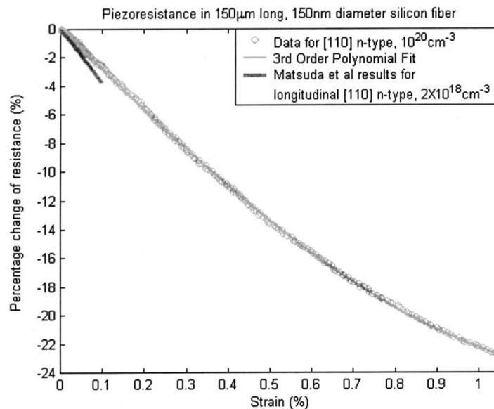
**Fig. 2.9:** Relative change in resistance of a silicon nanowire depending on strain, as measured by Chen [37]. Measurement data is compared to formerly obtained results by Matsuda [38]. Nanowires in the [110] orientation with a doping rate of  $10^{20}\text{cm}^{-3}$  were used. The piezoresistive effect is linear in a large range.
