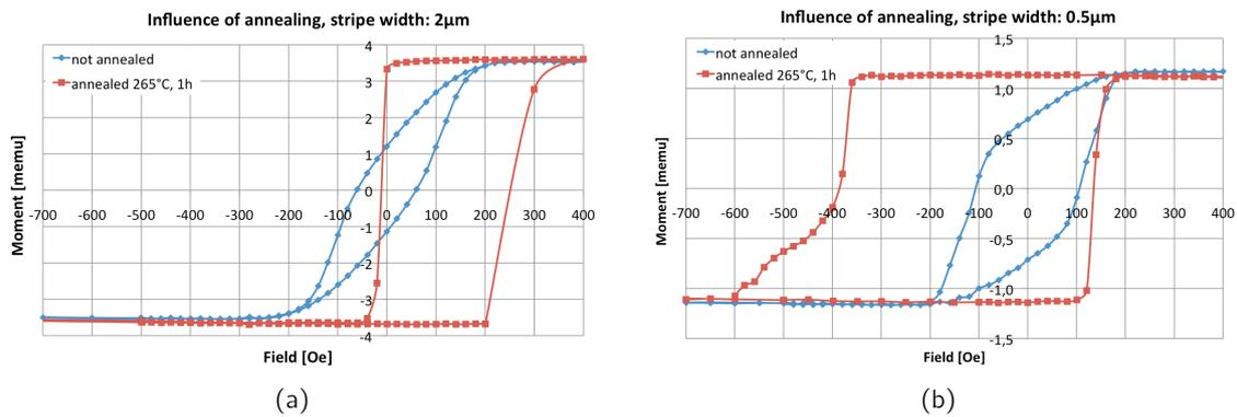
**Fig. 3.31:** Influence of annealing (265°C for 1h) on stripe-patterned AF/F stacks ([PtMn 50nm/CoFe 20nm] $\times$ 5/PtMn 50nm/Ta 50nm): (a) stripe width  $w = 2\mu\text{m}$ ; (b) stripe width  $w = 0.5\mu\text{m}$ . The coercive field increases after annealing and is larger for narrow stripes.
