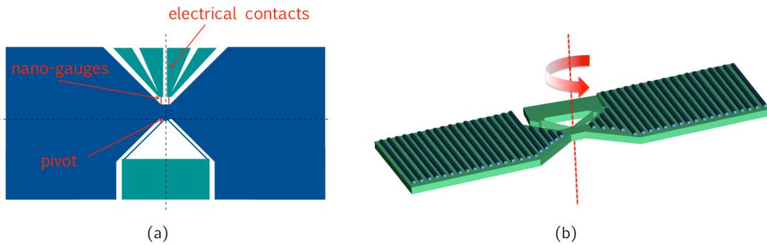
**Fig. 2.46:** Magnetometer design for detection of in-plane-field components: (a) schematic top view; (b) schematic 3D view, representing the case of deposited CoFe/PtMn multilayers on top of the structure (cf. section 2.2.2).
