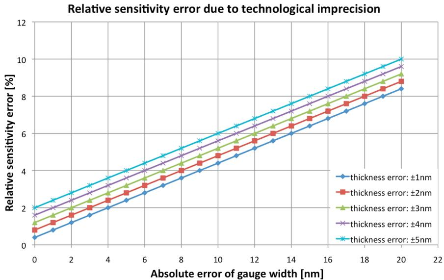
**Fig. 2.42:** Maximum possible variation in sensitivity depending on errors of gauge width and gauge thickness. A polarization current of  $100\mu\text{A}$ , a silicon resistivity of  $2.3 \times 10^{-5} \Omega\text{m}$  and nominal gauge dimensions of  $0.25 \times 0.25 \times 5\mu\text{m}^3$  were assumed for numerical evaluation.
