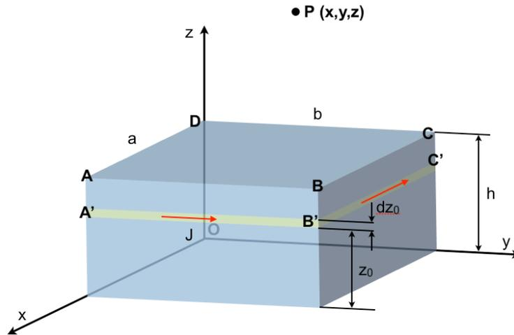
**Fig. A.1:** Modeling of a permanent magnet with a current loop model
