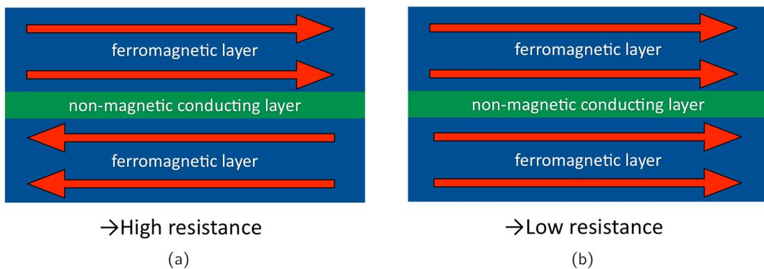
**Fig. 1.9:** Principle of Giant Magnetoresistivity: (a) adjacent ferromagnetic layers are separated by thin non-magnetic, electrically conducting layers and exhibit opposite magnetization directions in their initial state; (b) in presence of an external magnetic field, magnetizations in the ferromagnetic layers align into the same direction, which leads to a reduction of electrical resistance.
