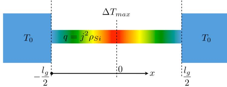
**Fig. 2.20:** 1D model of current-induced joule heating in a nano-gauge. The gauge is fixed to two infinitely large heat reservoirs, so that there is no temperature difference between the gauge's end and its clamping.
