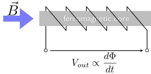
**Fig. 1.7:** Principle of a search-coil magnetometer
