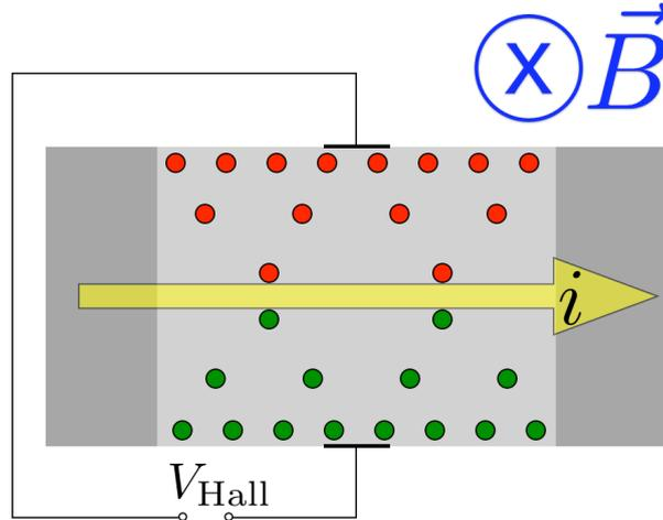
**Fig. 1.10:** Principle of the Hall effect: Charge carriers cumulate at both opposite sides of the Hall device in presence of a perpendicular magnetic field, so that a Hall voltage  $V_{\text{Hall}}$  is generated.
