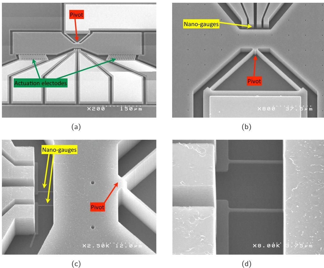
**Fig. 4.3:** Technology results for magnetometer structures designed for detection of in-plane field components: (a) The complete structure with integrated electrical contacts and actuation electrodes; (b) Bending beams build the pivot, the nano-gauges are placed on the opposite side; (c) 250nm thin nano-gauges compared to the  $10\ \mu\text{m}$  thick Silicon structure; (d) Close view of the nano-gauges.
