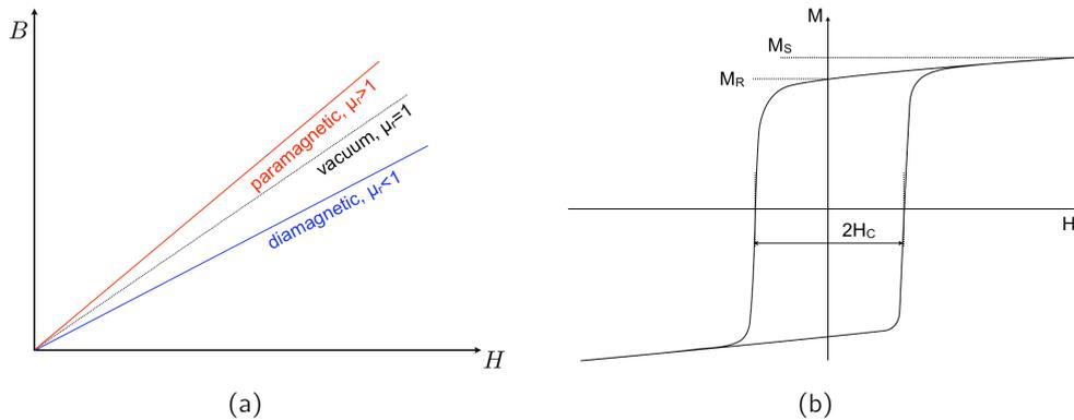
**Fig. 3.2:** Properties of magnetic materials: (a) Classification of materials by means of their magnetic permeability; (b) Typical  $M(H)$  hysteresis loop of a ferromagnetic material.  $H_C$  is the coercive field,  $M_R$  the remanent magnetization and  $M_S$  the saturation magnetization.
