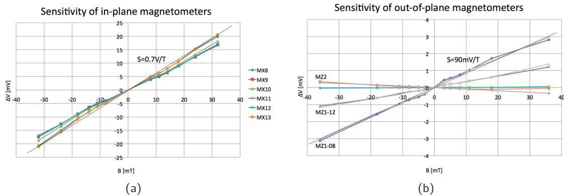
**Fig. 5.4:** First characterization results with the application of a magnetic field using permanent magnets and a gauge polarization current of  $50\mu A$ : (a) Measured sensitivity of in-plane-magnetometers. The measured sensitivity matches well the sensitivity predicted by design; (b) Measured sensitivity of out-of-plane magnetometers. The actual sensitivity is below the predicted value.
