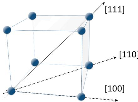
**Fig. 2.8:** Nomenclature for directions in crystalline Silicon
