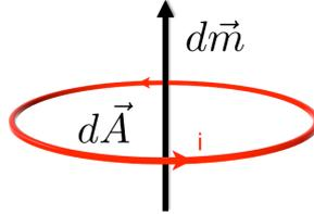
**Fig. 3.1:** Closed current loop for modeling of a magnetic dipole moment
