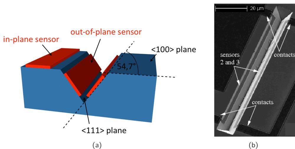
**Fig. 1.6:** Z-sensitive AMR sensor: (a) Principle of an out-of-plane AMR sensor: Trenches etched by anisotropic KOH etching into the  $\langle 100 \rangle$  plane of a Silicon substrate fix the out-of-plane sensors at an angle of  $54.7^\circ$  with respect to the substrate. So, the sensor is sensitive to the magnetic field component vertical to the  $\langle 100 \rangle$  Silicon plane; (b) SEM photograph of the technological realization of da Silva *et al.* [8].
