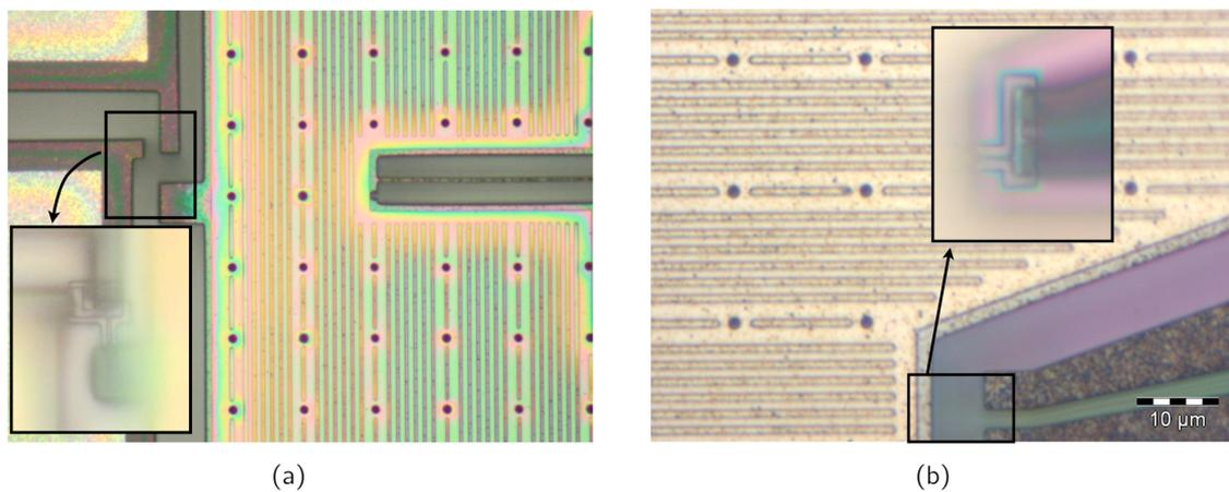
**Fig. 4.5:** Validation of critical process steps for magnetometers using integrated AF/F multilayers: (a) outer left border of a z-magnetometer using a combination of torsion- and bending beams. The small picture shows a focus on the nano-gauge. (b) Z-magnetometer using torsion beams for suspension.
