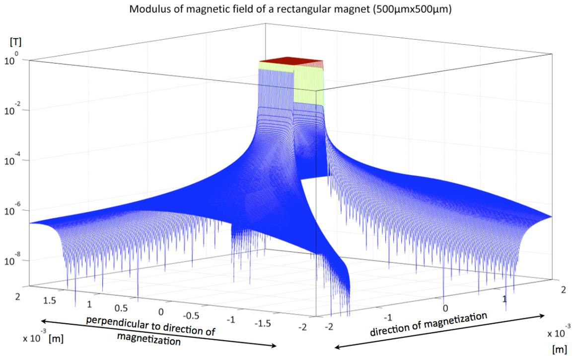
**Fig. 2.23:** Calculated magnetic field of a permanent magnet with a magnetization of 0.7T and a size of  $500 \times 500 \times 1\mu\text{m}^3$ . Greatest field magnitudes are situated along the direction of magnetization.
