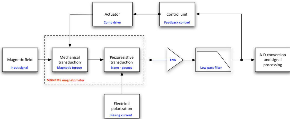
**Fig. 2.5:** Model of the transduction chain for the considered sensor. An optional control circuit may be conceived for closed loop detection and is schematically presented as a simple feedback loop with a control unit, a low noise amplifier (LNA) and capacitive comb drives or electrodes as actuation units.
