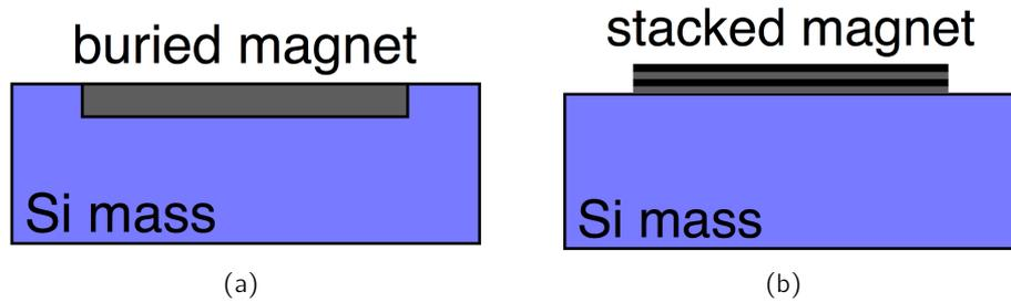
**Fig. 2.6:** Scheme of the two methods used to integrate magnetic material: (a) burying of hard magnetic material into a silicon mass; (b) stacked thin layers of ferromagnetic and antiferromagnetic material onto a silicon mass.
