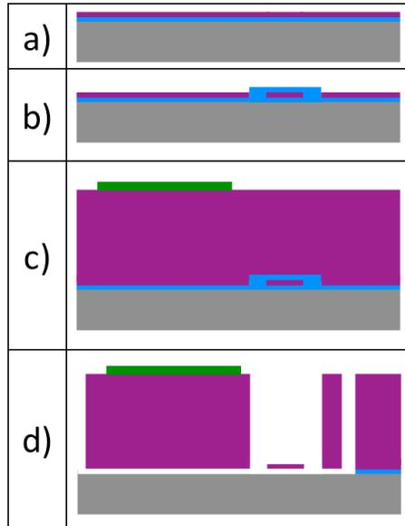
**Fig. 2.2:** Simplified process flow of the M&NEMS magnetometer: a) Start of the process on a SOI substrate; b) etching of nano-gauges within the monocrystalline top silicon layer and protection with  $\text{SiO}_2$ ; c) epitaxy of a thick monocrystalline silicon layer and deposition of magnetic material, which will be presented in chapter 3; d) DRIE etching of the MEMS structures and subsequent release by vapor hydrofluoric acid etching.
