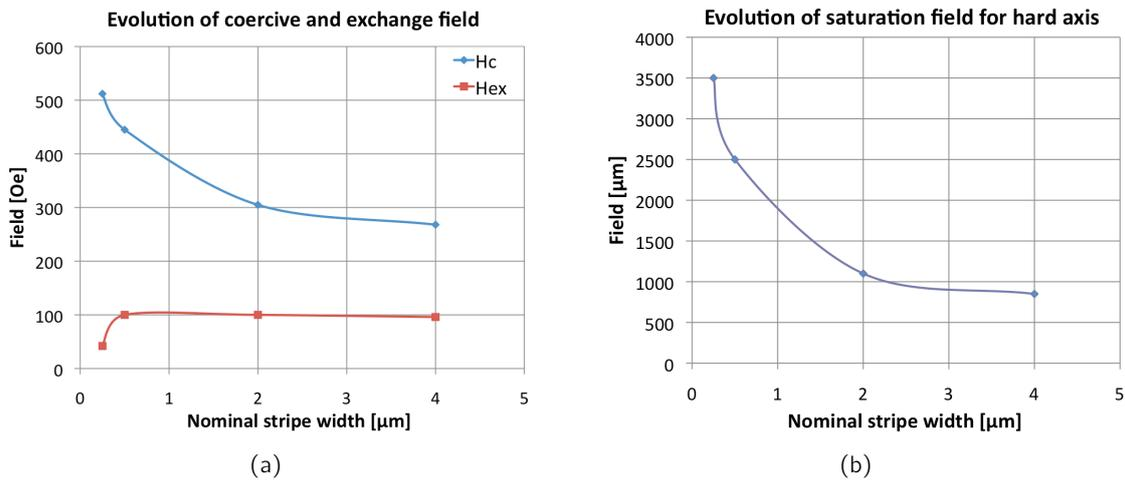
**Fig. 3.26:** Evolution of  $H_c$ ,  $H_{ex}$  and  $H_{sat,h}$  with stripe width: (a)  $H_{ex}/H_c$  ratio decreases for narrower stripes; (b) the field required to saturate the hard axis increases for narrower stripes.
