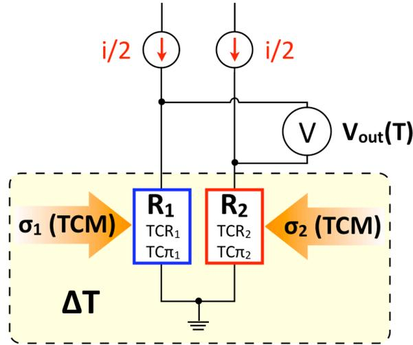
Fig. 2.45: Readout configuration considered for investigation of thermal effects
