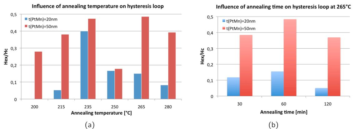
**Fig. 3.32:** Influence of annealing conditions for two different stacks. Stack 1) Ta 5nm/[PtMn 20nm/CoFe 10nm] $_{10}$ /PtMn 20nm/Ta 5nm. Stack 2) Ta 5nm/[PtMn 50nm/CoFe 20nm] $_5$ /PtMn 50nm/Ta 5nm: (a) variation of annealing temperature; (b) variation of annealing time.
