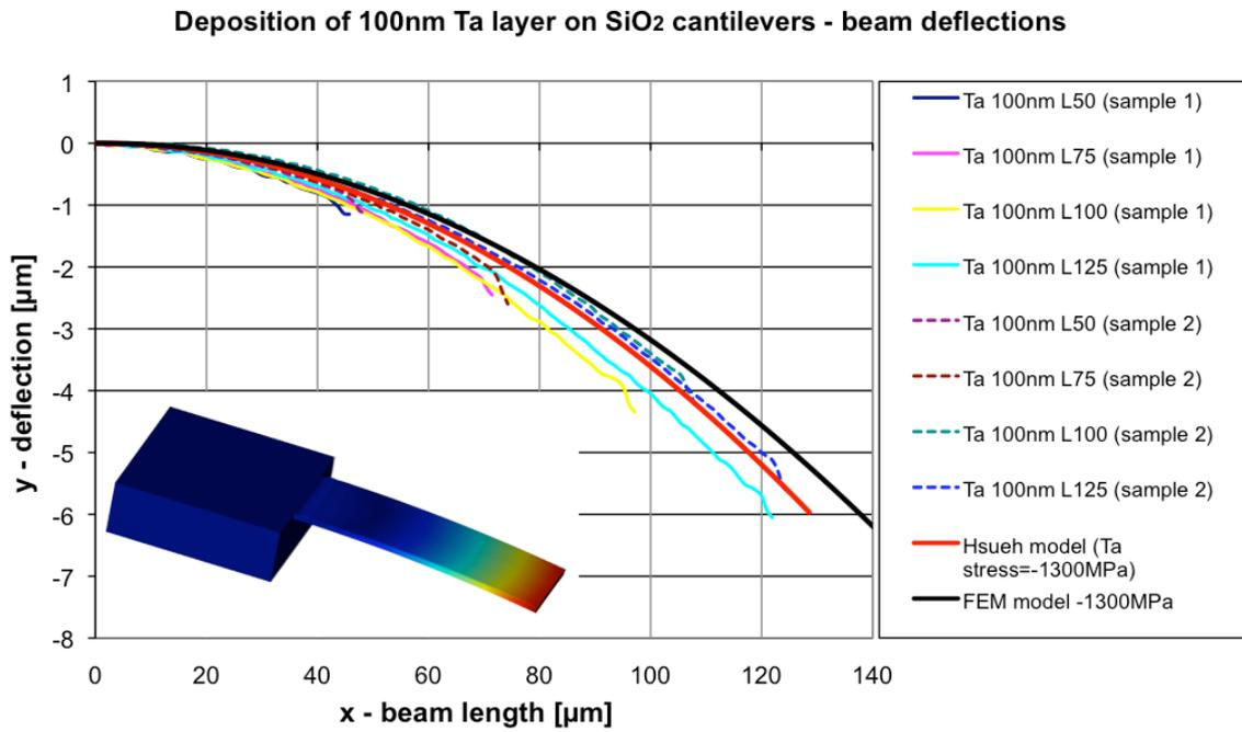
**Fig. 4.19:** Evaluation of stress in a 100nm thin Ta layer, based on the bending of cantilevers. Measurements were taken from 2 different samples which are represented by continuous and dashed lines. They show good conformity. The stress value extracted from the model is -1.3GPa, which is confirmed by FEM simulation of this cantilever.
