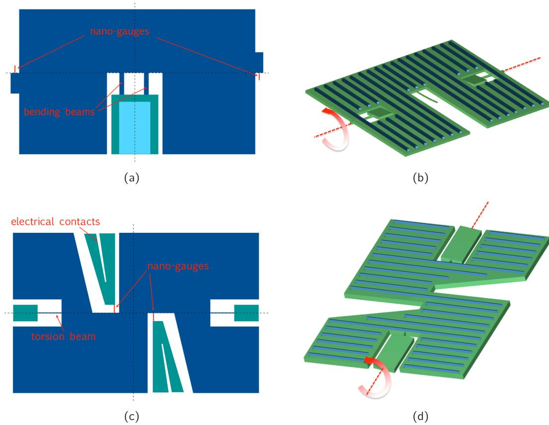
**Fig. 2.47:** Schematic view of the two types of Z magnetometers, where exclusively the case of a deposited stack of coupled antiferromagnetic and ferromagnetic layers is presented. (a) schematic top view of magnetometers using bending beams; (b) schematic 3D view of a magnetometer combining bending and torsion beams; (c) top view of a magnetometer using torsion beams; (d) schematic 3D view of the same structure.
