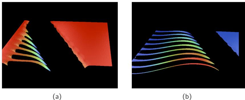
**Fig. 4.21:** Deformation of cantilevers due to high compressive stress in a 330nm thick AF/F stack on 2 $\mu\text{m}$  thick SiO<sub>2</sub>: (a) short cantilevers after deposition of AF/F stack; (b) long cantilevers after deposition of AF/F stack. From a qualitative point of view, the deformation indicates high residual stress in the layer; finally, inhomogeneous cantilever deformations did not lead to a quantitative evaluation of stress.
