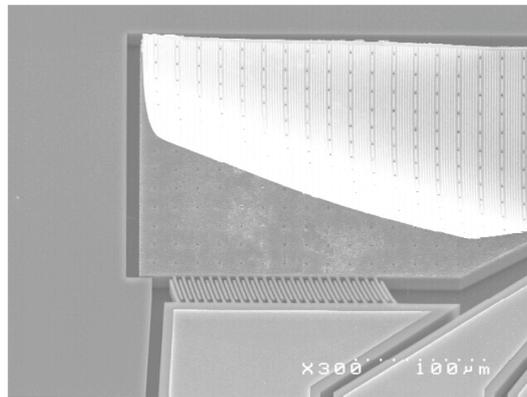
**Fig. 4.8:** Example for peel-off for a stack of AF/F multilayers after a HF etching step to release the MEMS structure.
