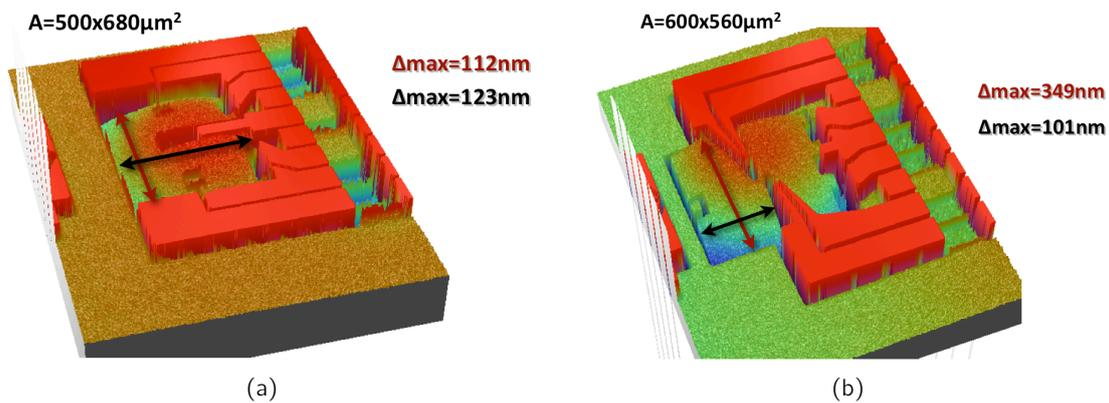
**Fig. 4.29:** Downward bending of z-magnetometer structures without integrated magnetic material: (a) z-magnetometer with a size of  $500 \times 680 \mu\text{m}^2$ , using a combination of torsion- and bending beam hinges; (b) z-magnetometer with a size of  $600 \times 560 \mu\text{m}^2$ , using torsion beams as hinge.
