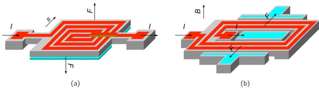
**Fig. 1.14:** 3 axis magnetometer as presented by Kyyräinen *et al.* [18], using capacitive sensing: (a) structure for measurement of the in-plane field component; (b) structure for measurement of the out-of-plane field component.
