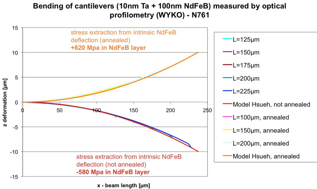
**Fig. 4.18:** Fit of the model to measurements
