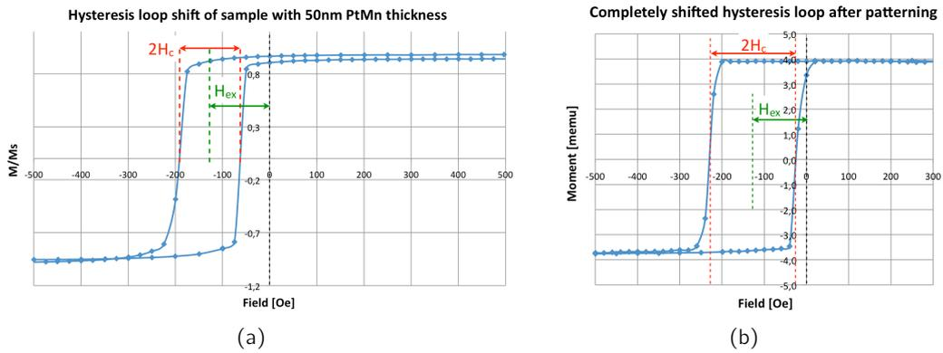
**Fig. 3.29:**  $H_{ex}/H_C > 1$  for a PtMn thickness of 50nm: (a) Completely shifted hysteresis loop ( $H_{ex}/H_C \approx 2$ ) of a sample using a [PtMn 50nm/CoFe 20nm] $\times$ 5/PtMn 50nm stack (full sheet deposition); (b) completely shifted hysteresis loop for a patterned [PtMn 50nm/CoFe 20nm] $\times$ 5/PtMn 50nm multilayer stack for a stripe width of 2 $\mu$ m.
