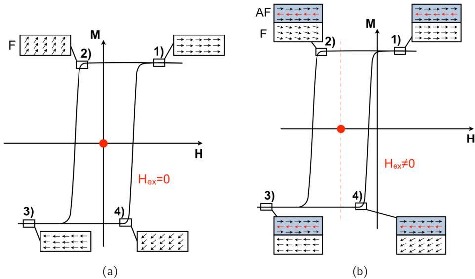
**Fig. 3.16:** Shift of hysteresis loop in ferromagnets and AF/F systems: (a) hysteresis loop of a simple ferromagnet; (b) shifted hysteresis loop of an exchange bias coupled AF/F system.
