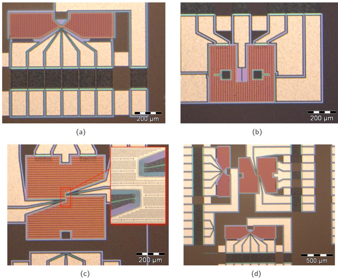
**Fig. 4.6:** Technological realization of magnetometers with integrated magnetic material (coupled antiferromagnetic and ferromagnetic multilayers): (a) Magnetometer for detection of the field components in the plane of the chip; (b) Magnetometer for out-of-plane field detection using a combination of bending- and torsion beams; (c) Magnetometer for out-of-plane field detection using torsion beams; (d) Fully integrated 3 axis magnetometer.
