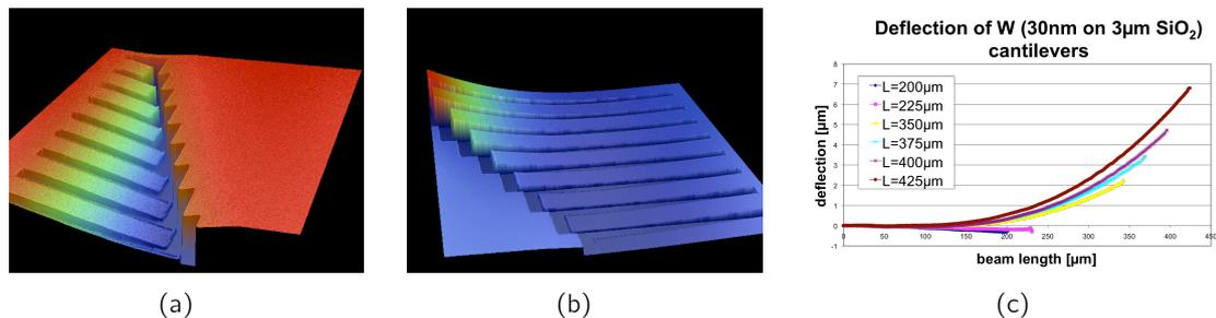
**Fig. 4.23:** Deflection of cantilevers with W layer: (a) short cantilevers are slightly bent downwards; (b) long cantilevers are bent upwards; (c) the measured deformation curves of cantilevers with different lengths are not superposed.
