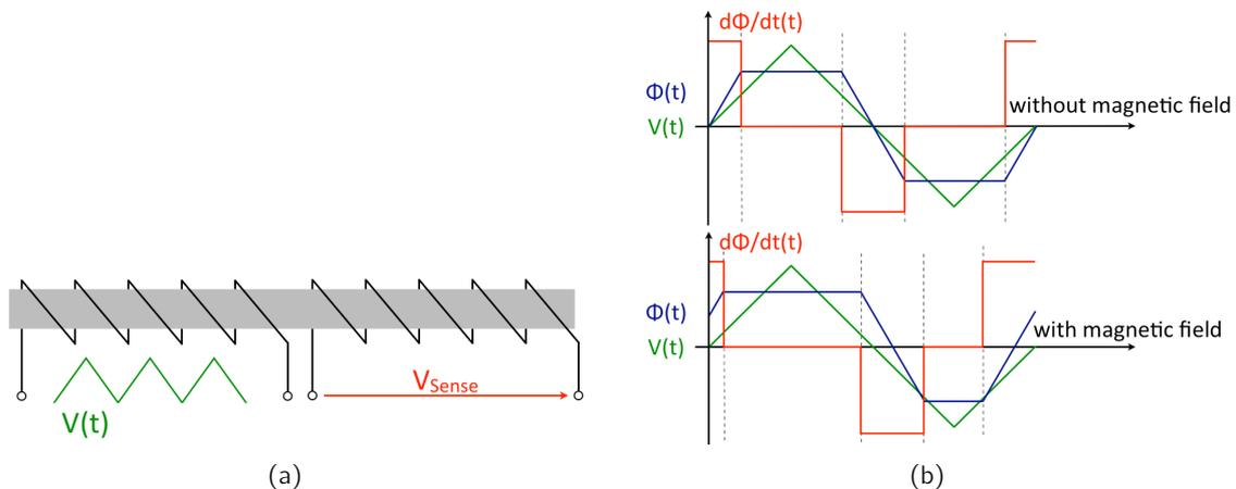
**Fig. 1.3:** Principle of a fluxgate magnetometer: (a) A ferromagnetic core is alternatively driven in- and out of saturation by a primary drive coil. Changes in flux density are then sensed by the secondary coil; (b) Scheme of the induction signal with and without external magnetic field.
