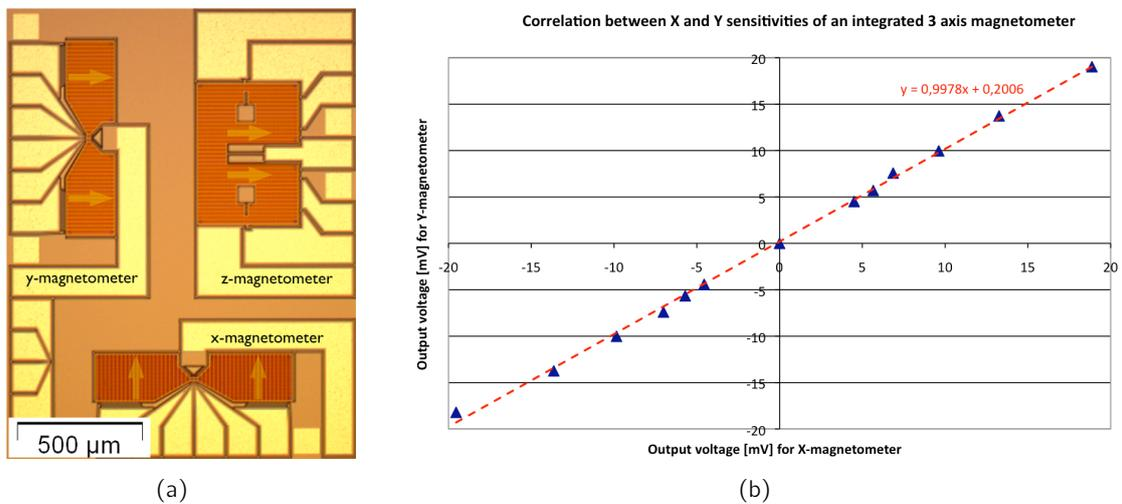
**Fig. 5.7:** Validation of the 3D magnetometer concept: (a) Ideal alignment of two magnetization directions in the integrated 3D magnetometer; (b) Measured correlation of 99.7% between x- and y sensitivity axes.
