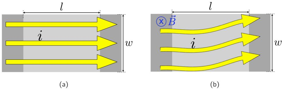
**Fig. 1.8:** Principle of a magnetoresistor: (b) Device without an external magnetic field: the resistance is minimum; (b) Device with an external magnetic field, where the current direction is deviated and resistance increases.
