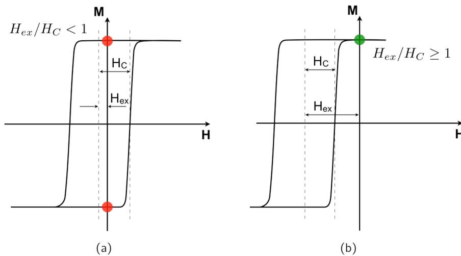
**Fig. 3.19:** Resistance to magnetic shocks: (a) two different possible remanent states after exposure to a high perturbation magnetic field; (b) one stable remanent state; insensitivity to magnetic shocks.
