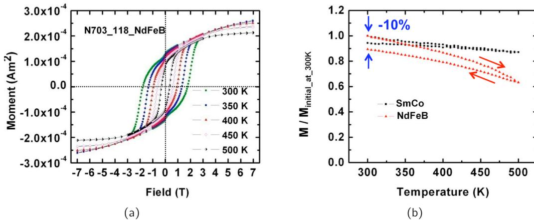
**Fig. 3.12:** Potential loss in remanence after exposure to high processing temperatures: (a) Dependency of the hysteresis loop on temperature (cold-deposited NdFeB films with in-plane magnetization); (b) Hysteresis in remanent magnetization after a heating-cooling cycle. For NdFeB, the potential magnetization loss is about 10%.
