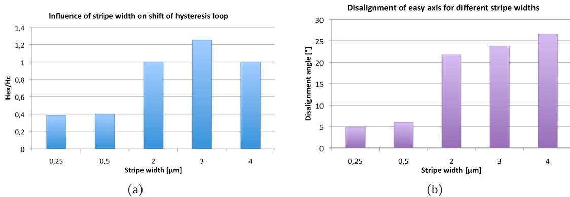
**Fig. 3.30:** Measured characteristics of patterned [PtMn 50nm/CoFe 20nm] $\times$ 5/PtMn 50nm stacks: (a) a completely shifted hysteresis loop is achieved with a stripe width of 3 $\mu$ m; (b) the disalignment angle  $\beta$  increases with growing stripe width.
