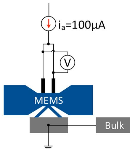
**Fig. 5.3:** Scheme of the used measurement configuration
