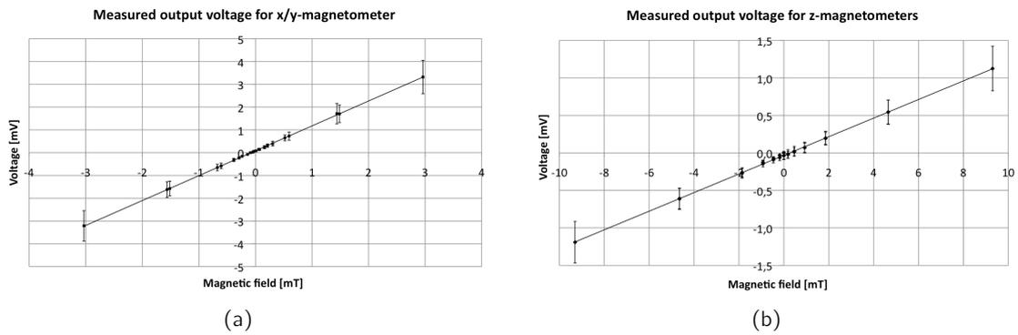
**Fig. 5.6:** Results for sensitivity measurements using coils. The error bars represent the technological dispersion over the wafer. (a) x/y-magnetometer with a distance of  $2.5\mu\text{m}$  between gauges and the fulcrum; (b) z-magnetometer (type MZ1) with a bending beam length of  $150\mu\text{m}$ .
