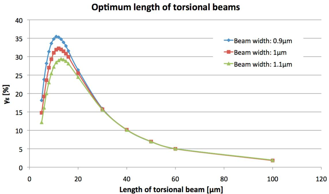
**Fig. 2.35:** Optimum lengths for 10  $\mu\text{m}$  thick torsional beams with variable width, as obtained from FEM analysis using COMSOL. Relative stress in the gauges is expressed in terms of  $\gamma_g$ , which is defined in eqn. 2.61.
