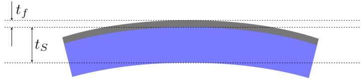
**Fig. 4.9:** Layer configuration considered for application of the Stoney formula
