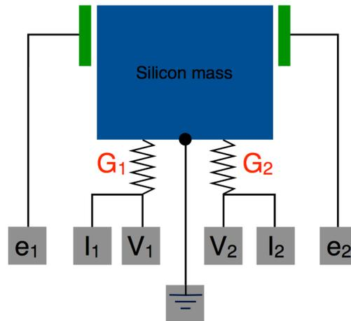
**Fig. 2.28:** Electrical connections needed for electrostatic actuation of the Silicon mass ( $e_1$  and  $e_2$ ), current biasing ( $I_1$  and  $I_2$ ) of the nano-gauges ( $G_1$  and  $G_2$ ), voltage measurement ( $V_1$  and  $V_2$ ) and connection of the mass.
