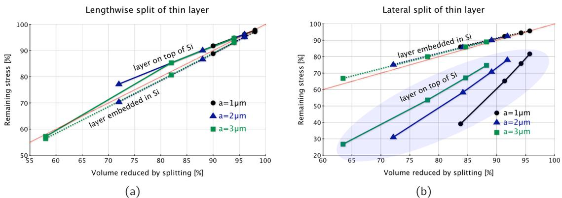
**Fig. 4.27:** Influence of patterned layers on residual stress: (a) normalized residual stress for a striped layer, orientated lengthwise to the beam; (b) normalized residual stress for a striped layer, oriented lateral to the beam. The dotted red line indicates the residual stress which would remain in case of a simple reduction of the layer’s volume without patterning.
