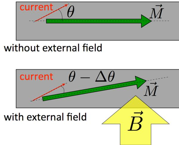
**Fig. 1.4:** Principle of an AMR device: An external magnetic field tilts the magnetization, so that the electrical resistance is modified with a changing angle  $\theta$  between current and magnetization direction.
