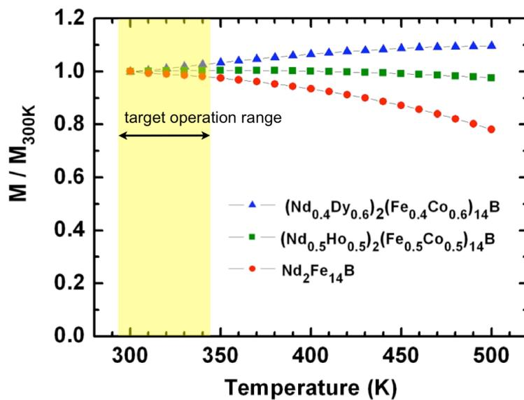
**Fig. 3.13:** Effect of substitution of Nd content for Dy and Ho on the temperature dependency of remanence. A stable remanence in the targeted temperature range of  $-10^\circ\text{C} - 50^\circ\text{C}$  is obtained by substitution of Nd content for Ho.
