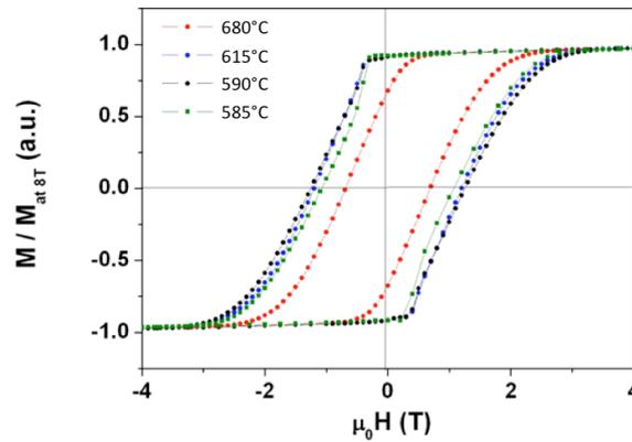
**Fig. 3.11:** Initial magnetic properties measured for different annealing temperatures between 585°C and 680°C on 5µm thick NdFeB layers with out-of-plane magnetization, carried out by the Néel Institute.
