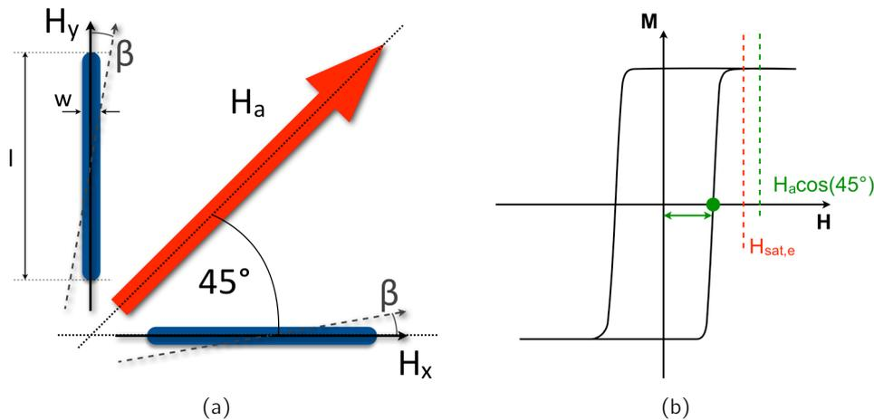
**Fig. 3.22:** Process for integration of two magnetic easy axes: (a) Configuration for integration of two perpendicular magnetization directions; (b) For saturation of the easy axis, the applied field during annealing must be sufficiently high, so that  $H_a \cos 45^\circ \geq H_{sat,e}$ .
