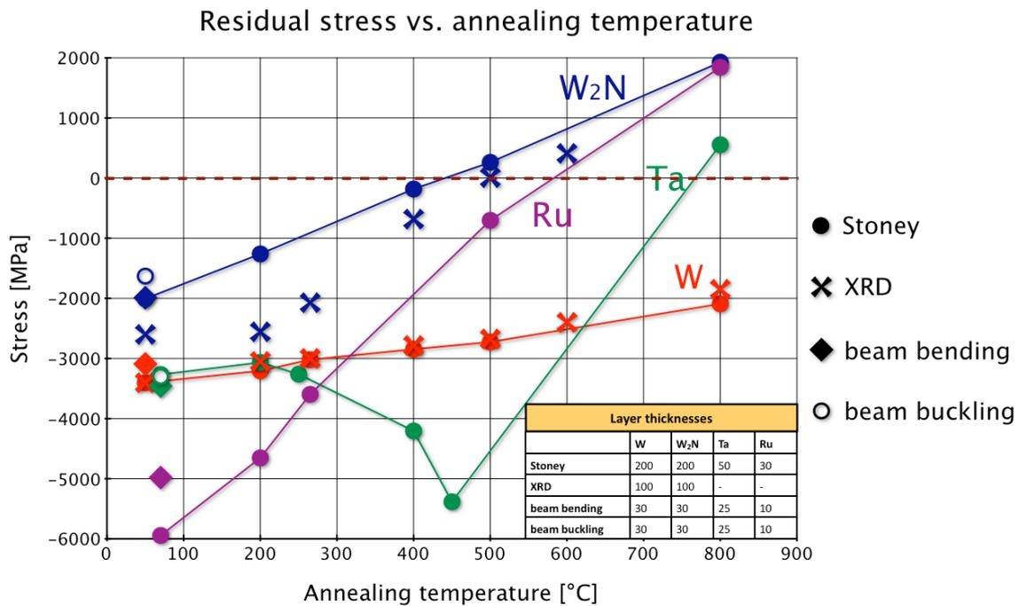
**Fig. 4.22:** Evolution of residual stresses for different potential sub- and capping layers with different annealing temperatures. Individual measurement points were obtained from all four characterization methods.
