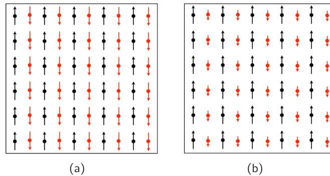
**Fig. 3.5:** Antiferromagnetic and ferrimagnetic materials: (a) Lattice configuration of an antiferromagnetic material; (b) Lattice configuration of a ferrimagnetic material.
