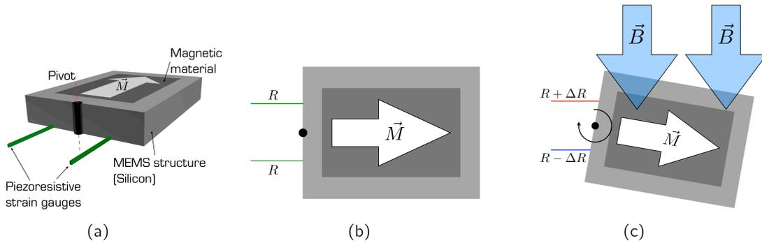
**Fig. 2.3:** Principle of a M&NEMS magnetic field sensor: (a) A silicon brick contains the magnetic material and is connected to two piezoresistive nano-gauges; (b) both strain gauges show same resistance when there is no surrounding magnetic field; (c) in presence of a magnetic field, the MEMS structure rotates around a pivot and deforms piezoresistive nano-gauges.
