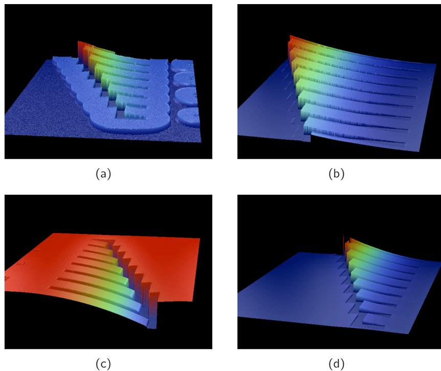
**Fig. 4.17:** Stress measurements of thin films with bent cantilevers: (a) Initial Ta layer on shorter cantilevers; (b) Initial Ta layer on longer cantilevers; (c) Downward-bent cantilevers with a 100nm thin NdFeB layer in their as-deposited state; (d) Upward-bent cantilevers with a 100nm thin NdFeB layer after annealing at  $600^\circ\text{C}$ . Note that deflections are not scaled.
