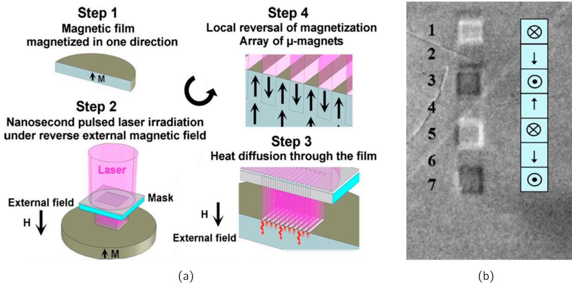
**Fig. 3.10:** Integration of multiple magnetization directions in a thin film of hard magnetic material using TMP (the images are taken from [59]): (a) Scheme of technological process; (b) Array with multiple integrated magnetization directions.
