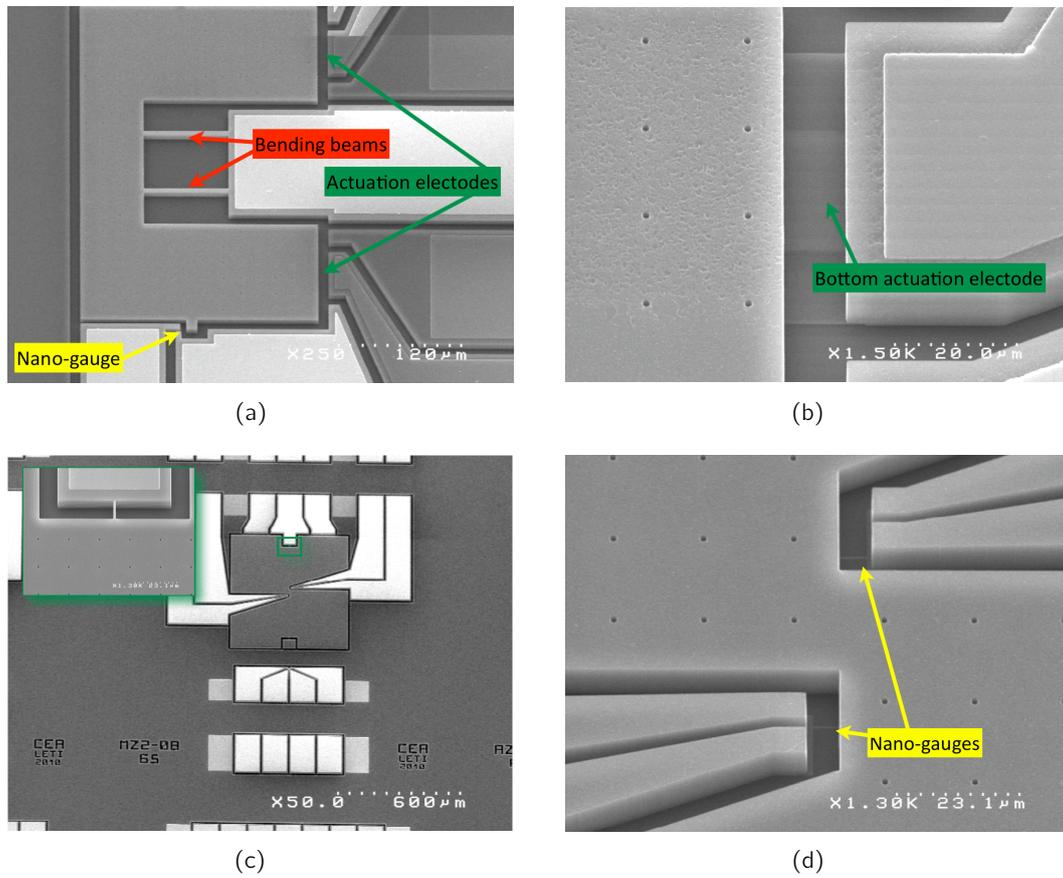
**Fig. 4.4:** Technological results for Z magnetometer structures: (a) Magnetometer structure using bending beams for rotation; (b) Actuation electrodes are situated under the silicon structure; (c) Magnetometer structure using torsion beams; (d) Position of the nano-gauges for a magnetometer using torsion beams.
