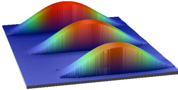
**Fig. 4.24:** Buckling for beams of different lengths (350 $\mu\text{m}$ , 400 $\mu\text{m}$  and 450 $\mu\text{m}$ ) as measured for 3 $\mu\text{m}$  thick  $\text{SiO}_2$  substrates with a 30 $\mu\text{m}$  thin Tungsten layer.
