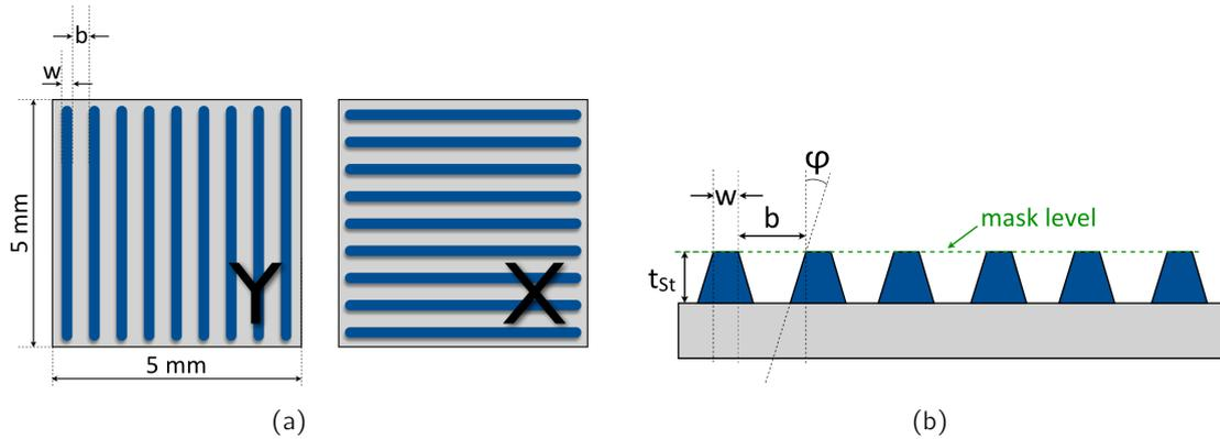
**Fig. 3.21:** Design of test samples for evaluation of the magnetic shape anisotropy: (a) scheme of arrays including perpendicularly orientated stripes for evaluation of magnetic shape anisotropy; (b) the limit for distance  $b$  between stripes is technologically determined, depending on the thickness of the deposited magnetic material.
