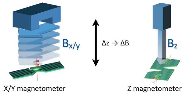
**Fig. 5.2:** Method for a first quantitative characterization of the magnetometers: U-shaped magnets were used for in-plane magnetometers, bar magnets for out-of-plane magnetometers. The magnets were vertically displaced above the sensors, which led to a change in magnetic field.
