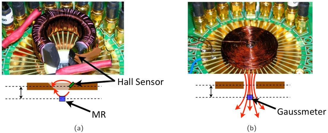
**Fig. 5.5:** Coils mounted on measurement cards for enhanced measurement precision: (a) toroidal coil for generation of in-plane field components; (b) planar spiral coil for generation of out-of-plane field components.
