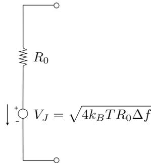
**Fig. 2.12:** Modeling Johnson noise in a piezoresistive gauge
