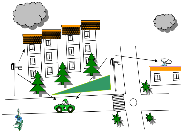
Figure 1.5: Example of Pico cell deployment serving static and moving users
