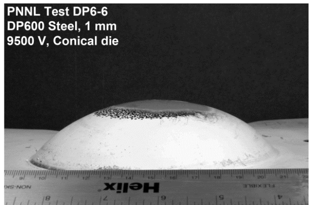
Figure 47 - Images comparing free forming and conical die forming for DP600 at 9500V.
