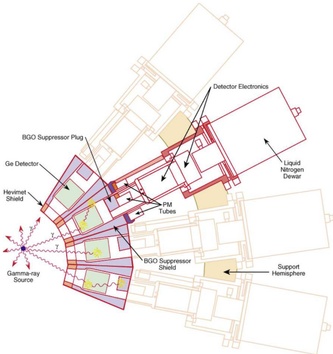
Figure 4.5: Schematic view of a Gammasphere module. The Ge crystal (Ge) (in green) is surrounded by a BGO shield (in purple) around and at the back ( back plug to catch scattered \gamma rays escaping from the rear of the Ge crystal). An absorber foil is set at the front of the module (not represented). A hevimet shield (orange) can be placed in front of the BGO, but has been removed in our experiment. The Ge crystal is kept cold with liquid nitrogen.
