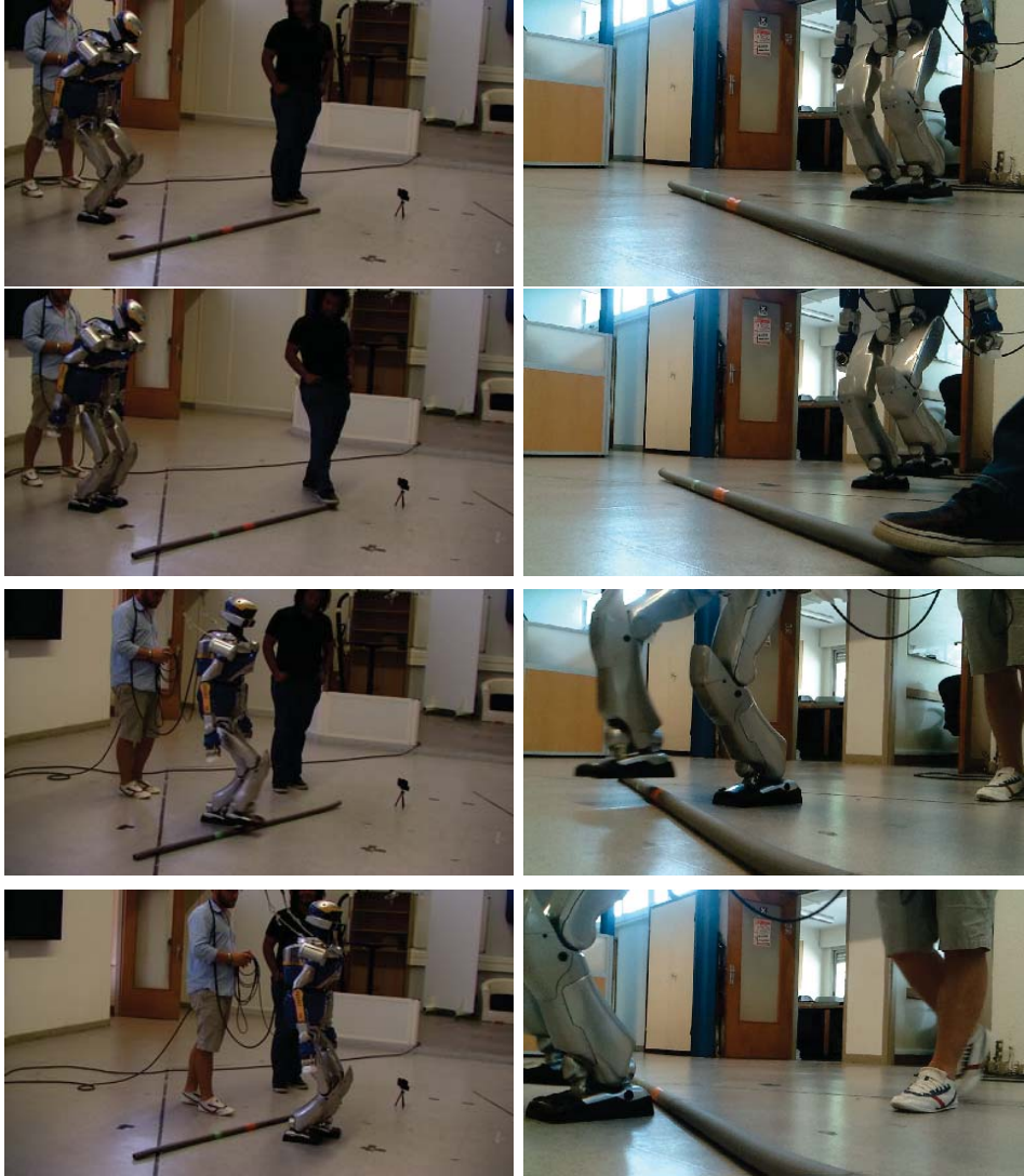
Figure 5.7: Stepping over a bar on HRP-2
