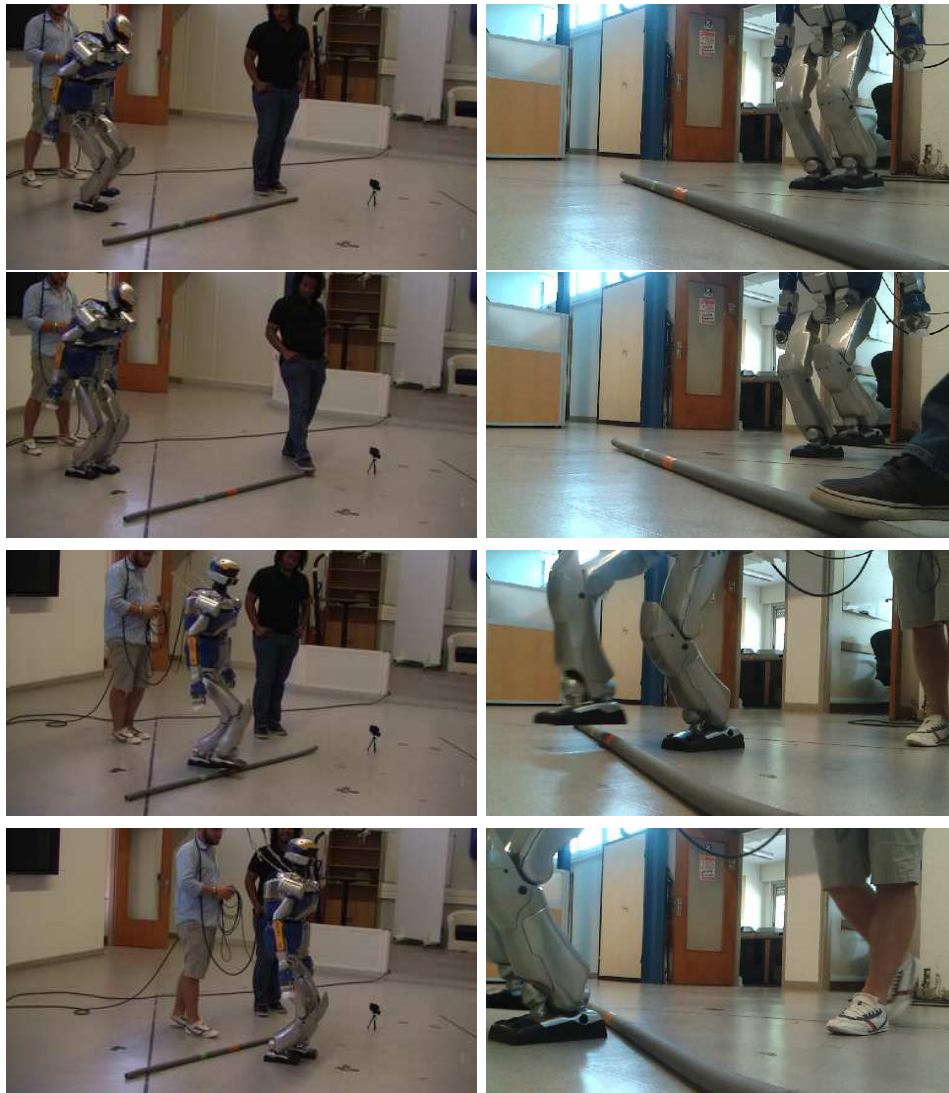
Figure 5.7: Stepping over a bar on HRP-2
