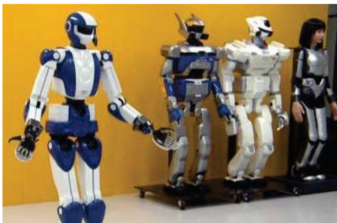
Figure 1.5: Some of the HRP family, from left to right: HRP-4, HRP-2, HRP-3P and HRP-4c
