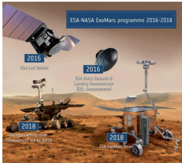
Figure 1: Elements of the ESA ExoMars programme 2016-2018. On the left TGO and the EDM, to be launched in 2016, and on the right the rover equipped with a drill (in black in front of the rover), to be launched in 2018. The NASA Rover part of the project was deleted in February 2012. Credit ESA.
