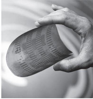
**Figure I-1** | Left: Roll-to-roll production of flexible organic photovoltaic modules. (After OE-A brochure, 3<sup>rd</sup> Edition, 2009) Right: Fully processed 150nm wafer foil containing all-polymer transistors and integrated circuits. (After ref.,<sup>[2]</sup> P332)
