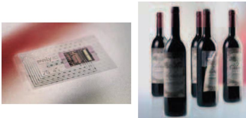
**Figure I-4** | Left: Printed RFID tags. (After OE-A brochure, 3<sup>rd</sup> Edition, 2009) Right: RFID tags for brand protection. (After OE-A brochure, 2<sup>nd</sup> Edition, 2007)
