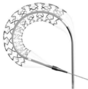
FIGURE 2.20: Coronary stents are very rigid on their radial axis to handle the pressure of the artery wall, but very flexible in the perpendicular direction to conform to the curvature of the artery.
