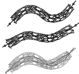
FIGURE 2.6: Schematic illustration of the limitations of the linear, marker-ball based registration realized with an image processing software for explanatory purpose (not necessarily geometrically exact). The two top images are two images of a same stent. Bottom is the marker-ball based registration. Although the two marker-balls are accurately registered, the stent, that underwent a non-linear deformation is not accurately registered. The guide-wire that supports the marker-balls is also undergoing a non-linear deformation. We use it as additional landmark in our nonlinear registration.
