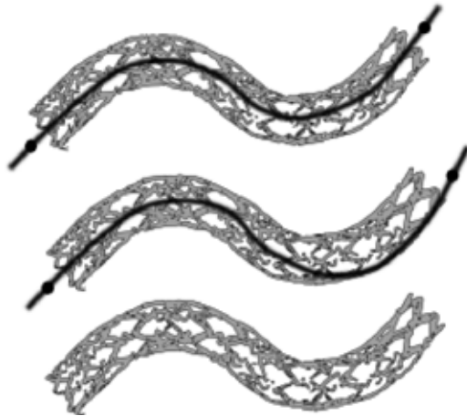
FIGURE 3.2: Scheme illustrating the difficulties in stent visualization introduced by the presence of the guide-wire. Top: the guide-wire hides the structure of the stent struts; Middle: the guide-wire hides partially the border of the stent; Bottom: ideal case for stent visualization where the guide-wire is not displayed (images are adapted from a Cypher stent photo [tim05]).
