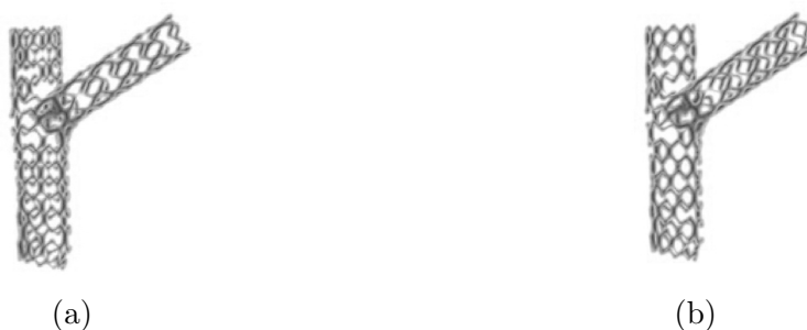
FIGURE 2.37: Illustration of the variability of the appearance due to strut superimpositions patterns. (a) and (b) depict the same stent under two viewpoints differing from few degrees.
