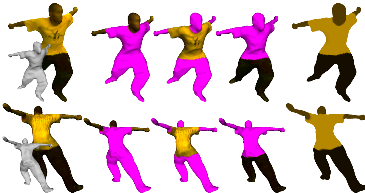
Figure 8: Segmentation result on a colored mesh obtained by multiview stereo algorithm. Front view (top row) and back view (bottom row). Original input colored mesh and the associated 3D shape (left). Result of the segmentation into three regions obtained by our algorithm (middle). Recovered mean values displayed for each region (right).
