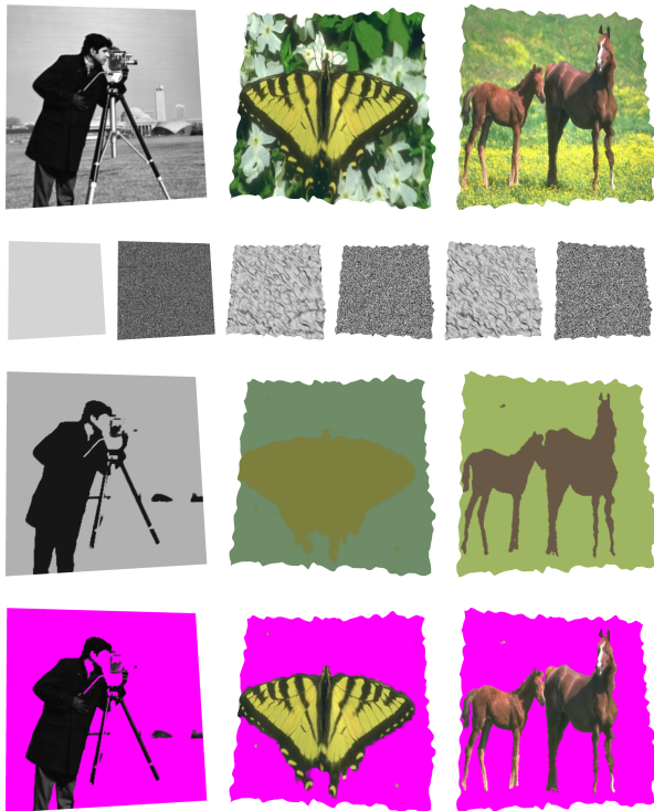
Figure 4: Segmentation results on meshes in the two-region segmentation on three different examples. From top to bottom: Input textured mesh; Mesh shape where the segmentation is performed and the initial random value of one component of \mathbf{U} ; Recovered mean values of each region; Segmented object.
