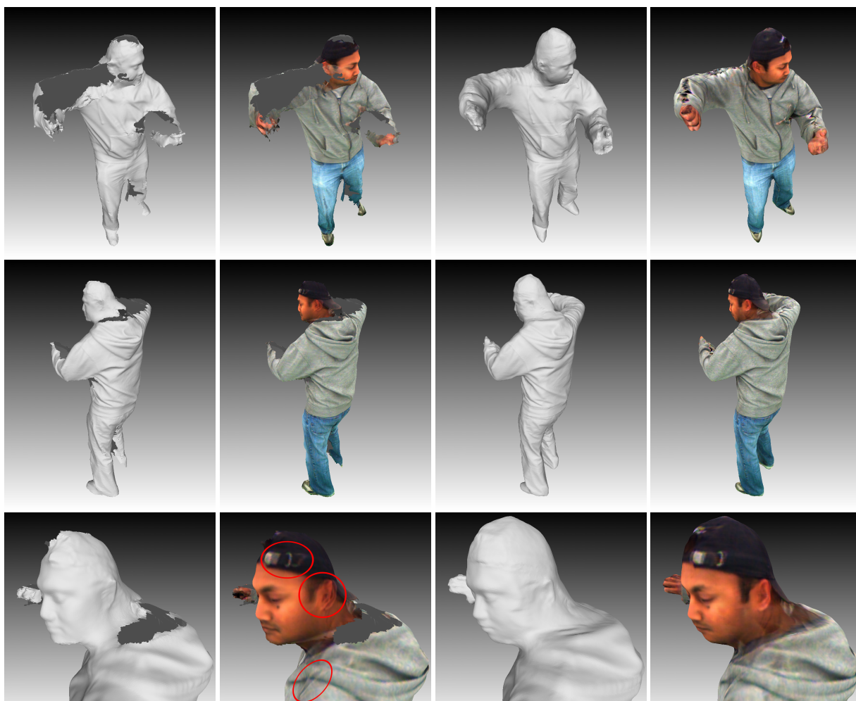
Figure 14: Results and comparison with [43]. From left to right: final shape of [43]; corresponding mean texture from visible cameras; result with the proposed approach; corresponding mean texture from visible cameras.
