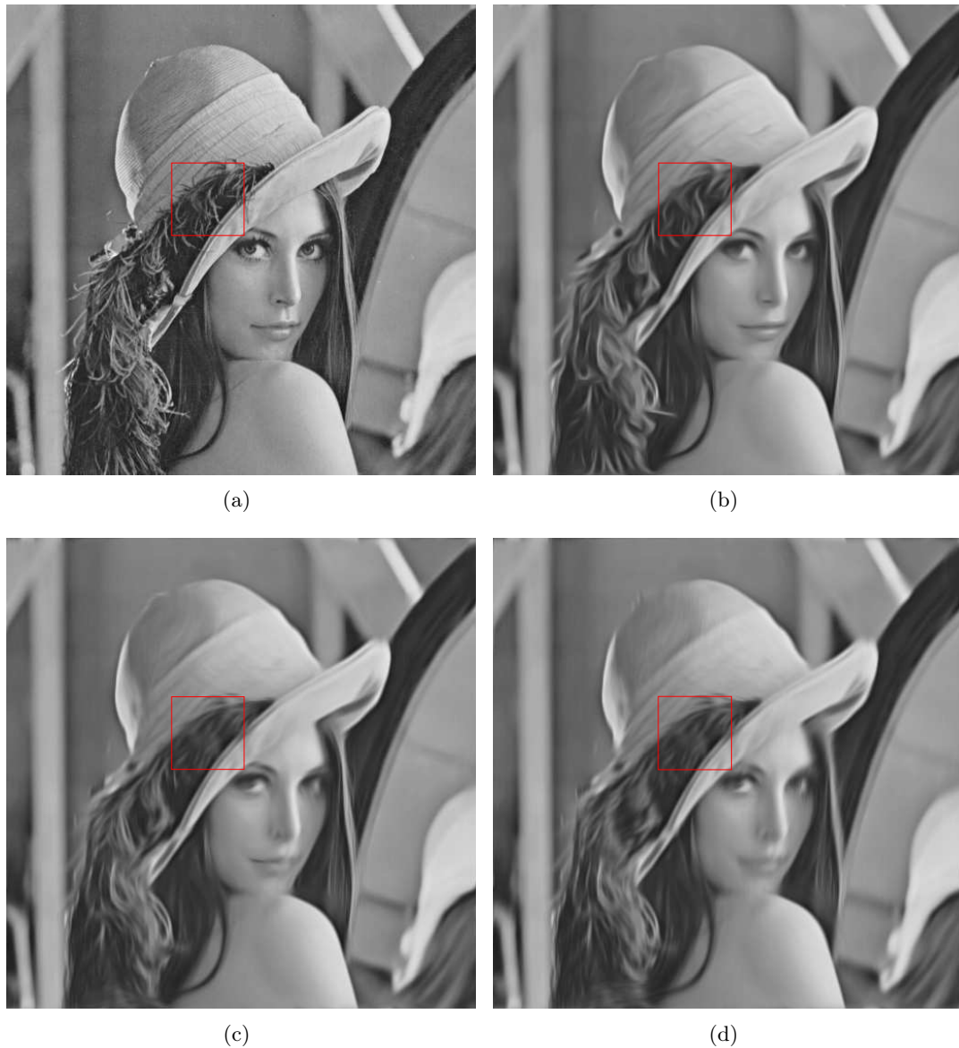
Figure 4.23: Image of Lena ( 512^2 pixels) at various feature sizes: (a) original data, (b), (c) and (d): filtered data with increasing feature size of 20, 50, and 100 respectively. Note how our algorithm smooths out details of the feathers on hat as the feature size increases while the preserving the edges greater than the specified feature size.
