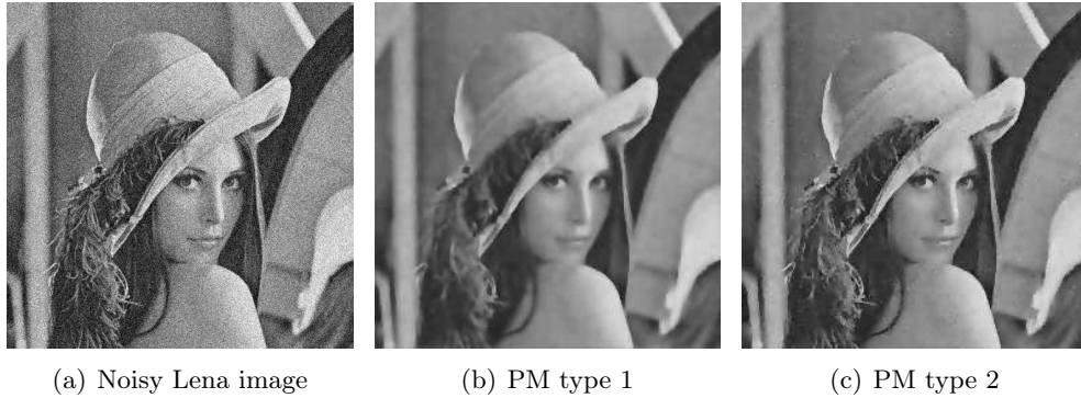
Figure 3.18: Smoothing with Perona-Malik diffusion: (a) A noisy Lena image. (b) The image of Lena smoothed by type 1 of Perona-Malik diffusion. (c) The image of Lena smoothed by type 2 of Perona-Malik diffusion. Both (b) and (c) were smoothed with 9 diffusion steps and K = 0.1 . Edges are well preserved but one can notice noise around edges.
