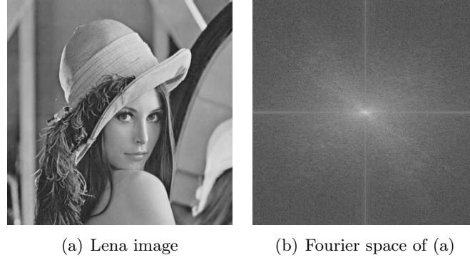
Figure 3.13: (b) displays the frequency data of the Lena image(a) after converting it with FFT.
