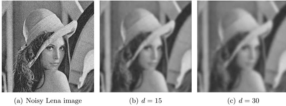
Figure 3.15: A noisy image of Lena (a) smoothed by linear heat diffusion at diffusion steps: (b) 15 and (c) 30. Diffusion is spread uniformly in all direction. The intensity values are spread over all the image as more diffusion steps is applied.
