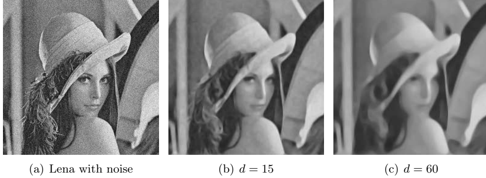
Figure 3.17: A noisy image of Lena(a) smoothed by geometric heat diffusion at diffusion steps: (b) 15 and (c) 60. Notice the edges are well preserved even as the number of diffusion steps increases. This can be seen in (c). The interior regions are blurred but the edges are preserved.
