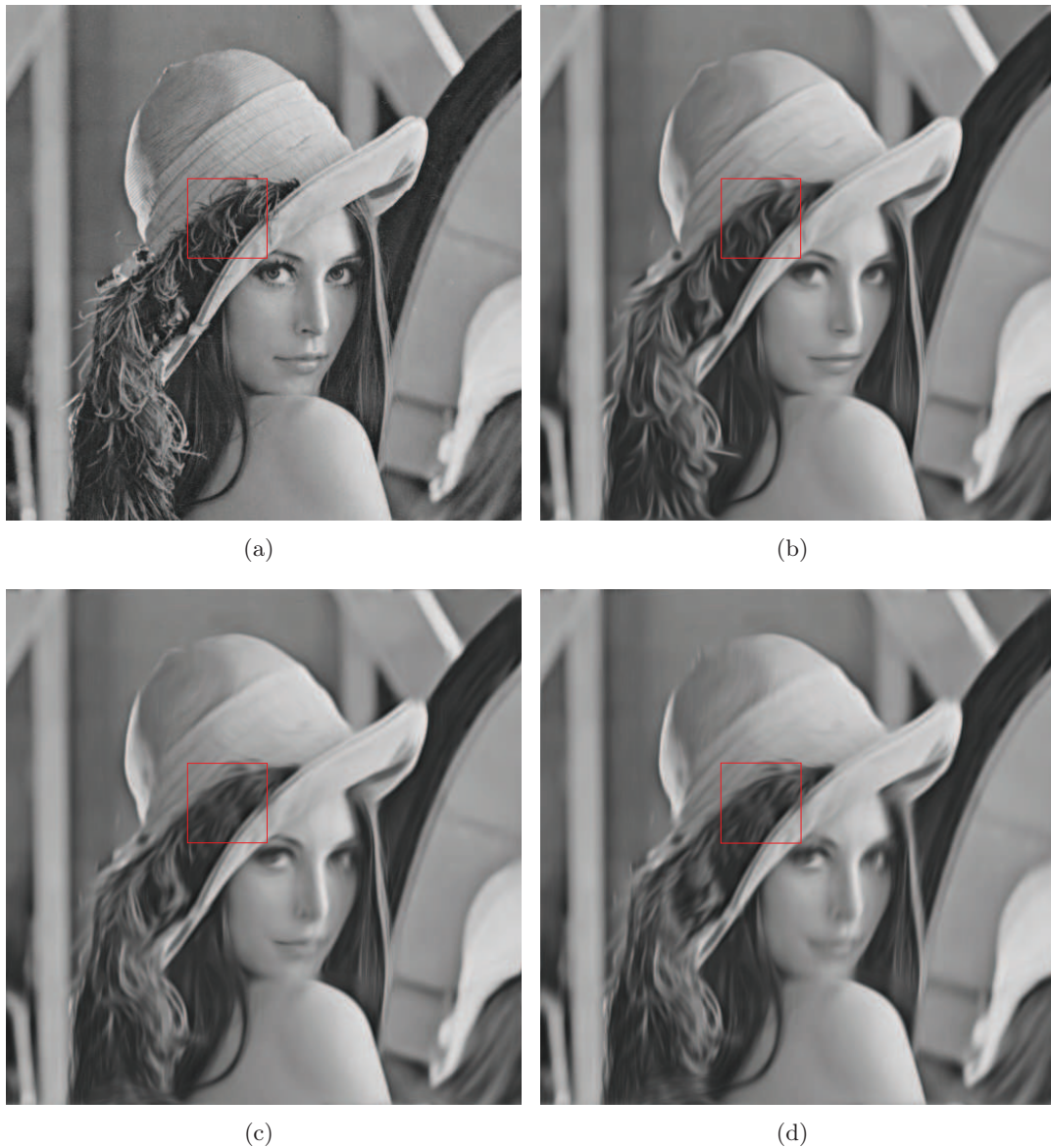
Figure 4.23: Image of Lena ( 512^2 pixels) at various feature sizes: (a) original data, (b), (c) and (d): filtered data with increasing feature size of 20, 50, and 100 respectively. Note how our algorithm smooths out details of the feathers on hat as the feature size increases while preserving the edges greater than the specified feature size.
