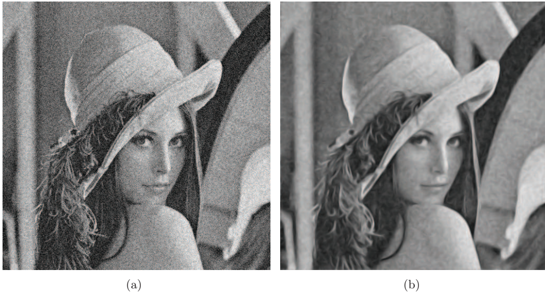
Figure 4.17: Image of Lena (512 2 pixels): (a) random noise is added to the image and (b) the image after smoothing by our algorithm at feature size s = 5 and 40 diffusion steps (processing time = 0.26 sec). Note how our algorithm reduces the noise while preserving the sharp and detail features such as the junctions, curve of the hat and the feathers on the hat.
