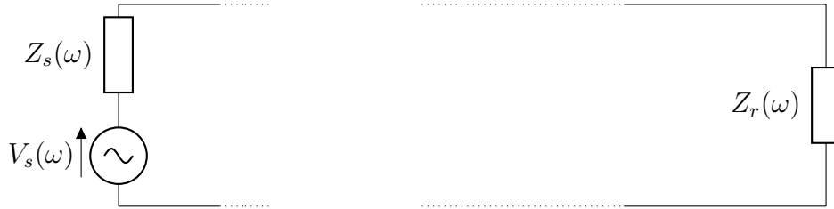
Figure 1.10: One generator source model
