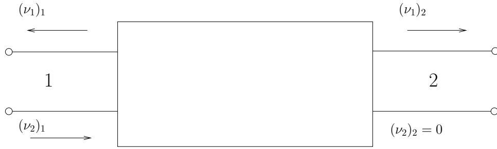
Figure 1.8: Reflectometry on a two-port network
