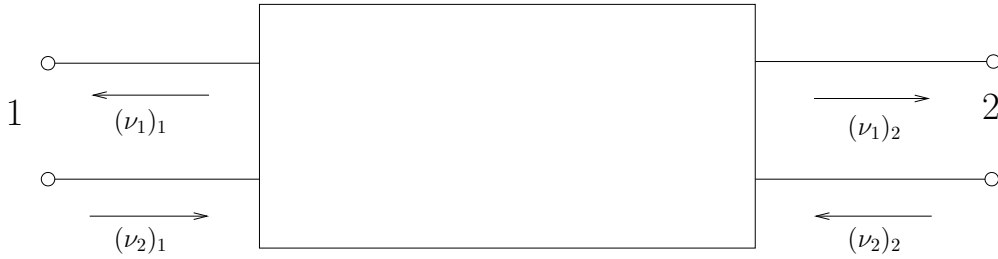
Figure 1.5: 2-Port Network with power waves
