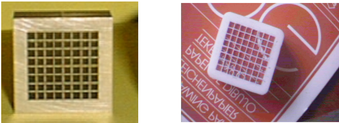
Figure 1: Matrix pictures: stainless steel matrix (left) and Teflon matrix (right) obtained with the epoxy mould displayed in Fig.2 (left).
