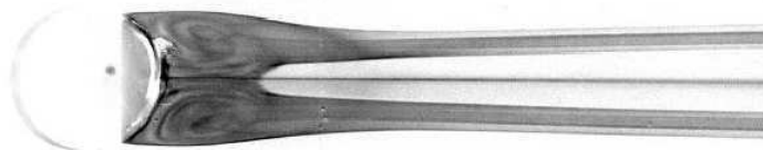
Figure 1.6: Streaklines showing a bifid wake. The plane of symmetry is imposed by the holding; Re = 250 . Przada et al. (2008).
