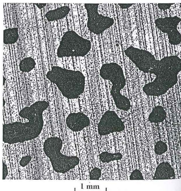
Fig. 2. Black and white photograph of a thick section using coaxial episcopy before sublimation (Km 105).
