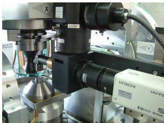
Figure 2.7 Interferometric microscope above the glass disc
