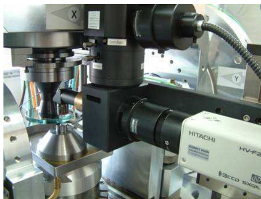
Figure 2.7 Interferometric microscope above the glass disc
