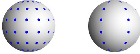
Figure 5.10: Sampling on equiangular grids, for exact reconstruction of band-limited functions at order  $L = 4$ . (left) the equiangular grid of  $K = (2L - 1)^2$  samples as in citetdriscoll-healy:94, and (right) the equiangular grid of  $K = 2L^2 - 3L + 2$  samples, as in McEwen and Wiaux [2011].
