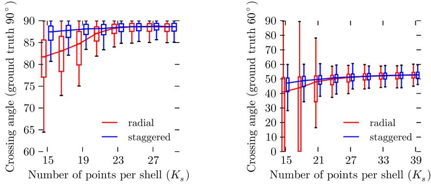
Figure 8.8: Crossing angle for a reconstructed fiber crossing. The  $q$ -space signal was reconstruction in the mSPF basis, with Laplace regularization as presented in Chapter 6, fixed regularization weight  $\lambda = 0.5$ . The ODF was further estimated using the SPFI method in Cheng et al. [2010a]. The boxplot represents min and max values, as well as the first and third quartiles.
