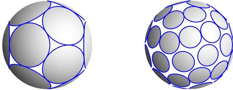
Figure 5.1: Spherical caps packing, (left) for  $K = 12$  the Fejes-Tóth bound is achieved: the centers of the spherical caps are the vertices of an inscribed icosahedron; (right) for  $K = 40$ , suboptimal configuration provided by the electrostatic energy minimization, as in Jones et al. [1999a].
