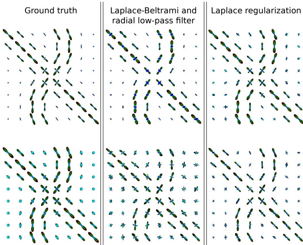
Figure 6.5: Reconstruction of a diffusion propagator field, from 120 measurements on 3 shells (max  $b$ -value was  $3000\text{s} \cdot \text{mm}^{-2}$ ). We compare the diffusion EAP profile (top row)  $P(r_0 \mathbf{u})$ , for  $r_0 = 15\mu\text{m}$ , and the diffusion ODF  $\psi(\mathbf{u})$  (bottom row). Fiber crossing are better resolved with Laplace regularization, and isotropic regions are smoother.
