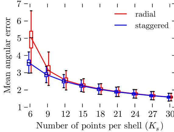
Figure 8.7: Average angular error between the principal direction of the estimated tensor and the axis of the cylinder. Signal simulation and reconstruction was repeated with 2000 different orientations, and 100 repetitions with random, Rician noise for each orientation. We plot here the median, first and third quartiles, and extremal values of the angular error (in degrees).
