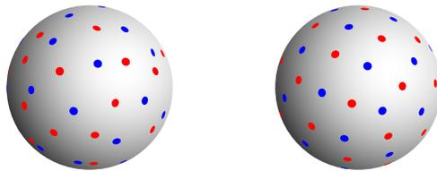
Figure 8.6: (left) incrementally constructed point set on  $S = 2$  shells,  $K_s = 17$  points per shell, and (right) optimal configuration for the same parameters. For such a small sample size, the incremental construction gives poorly uniform configurations.
