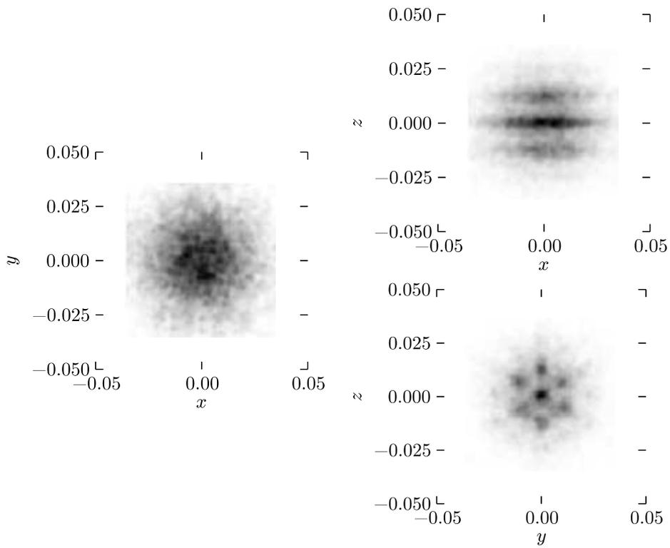
Figure 3.6: Displacement of 10000 water molecules over the diffusion time  $t = 60$  ms. (left) unrestricted medium, and (right) within the population of fibers presented on Fig. 3.5. The fibers axis is parallel to the  $x$ -axis.
