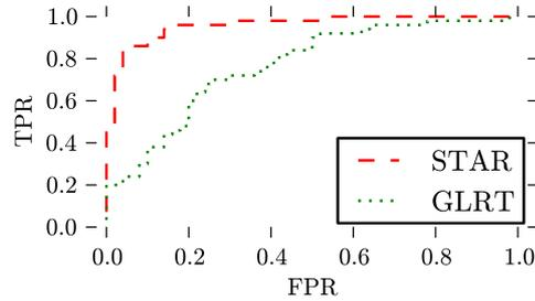
Figure 7.4: TPR versus FPR in motion detection. This experiment was done on 100 datasets without motion, and 100 acquisitions for which a rigid motion (rotation by an angle of  $2^\circ$ ) occurred after 20 diffusion weighted images were acquired.
