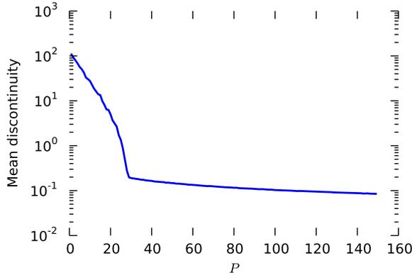
Figure 6.3: Discontinuity, measured about the origin, of a synthetic Gaussian diffusion signal, reconstructed from  $K$  measurements on 3  $q$ -shells, plus  $P$  virtual measurements at  $\mathbf{q} = \mathbf{0}$ . The discontinuity remains very high, even for a large number of additional, virtual measurements ( $P = 150$ ).
