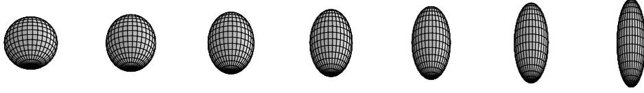
Figure 3.10: Diffusion tensors, represented as ellipsoids, for FA ranging from 0.0 to 0.6. The Mean Diffusivity is constant across the tensors.
