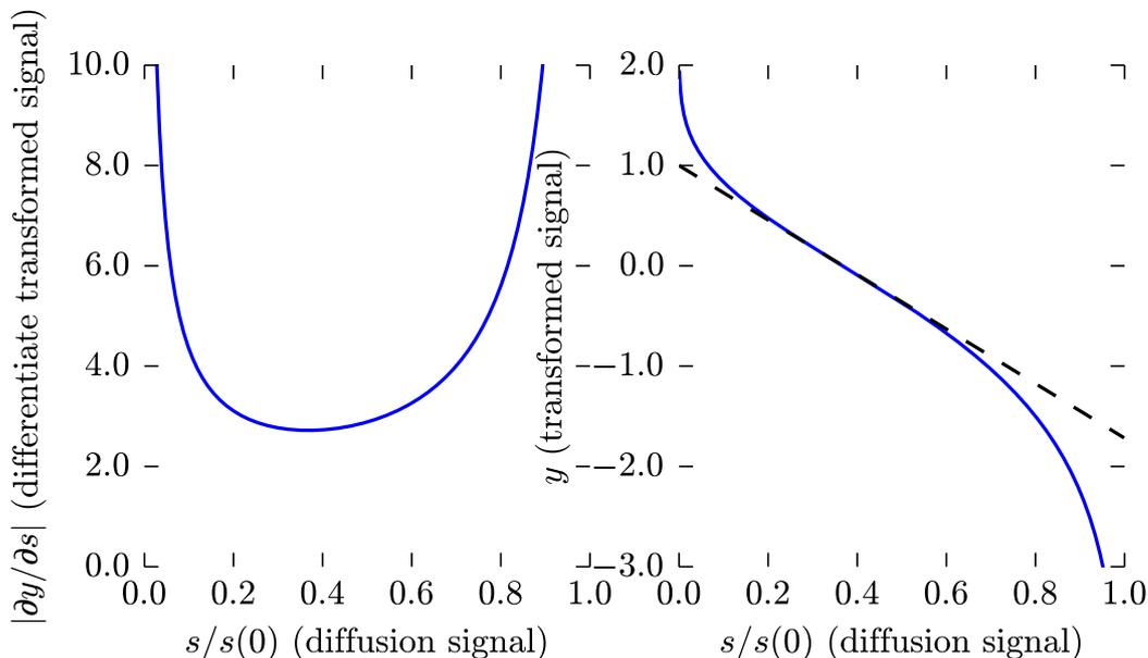
Figure 7.1: (left) Non linear transform on the diffusion signal; (right) derivative with respect to the signal. The distortion is maximum for  $s/s(\mathbf{0}) \rightarrow 0.0$  and  $s/s(\mathbf{0}) \rightarrow 1.0$ , and minimum for  $s/s(\mathbf{0}) \approx 1/e$ .
