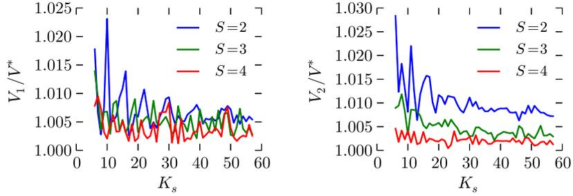
Figure 8.4: (left) normalized average energy per shell  $V_1$ . (right) normalized average energy of the sampling directions as a whole,  $V_2/V^*$ . The normalized energy are very close to 1 in all cases.
