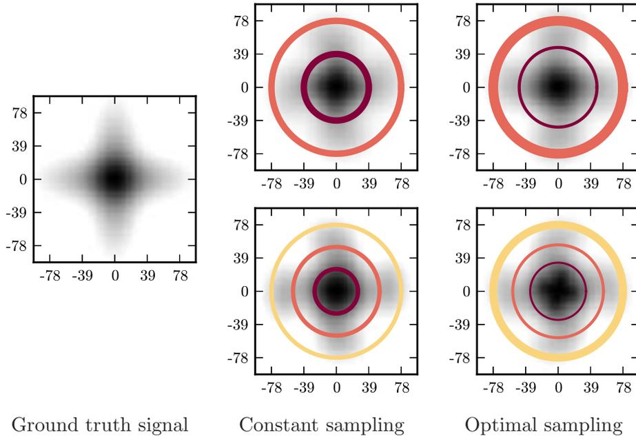
Figure 9.6: 2 shell (top) and 3 shell (bottom) sampling in action, for the reconstruction of a synthetic diffusion signal corresponding to a mixture of Gaussian, simulating fiber crossing. The circles represent the sampling shells, and the line widths are proportional to the number of points per shell.
