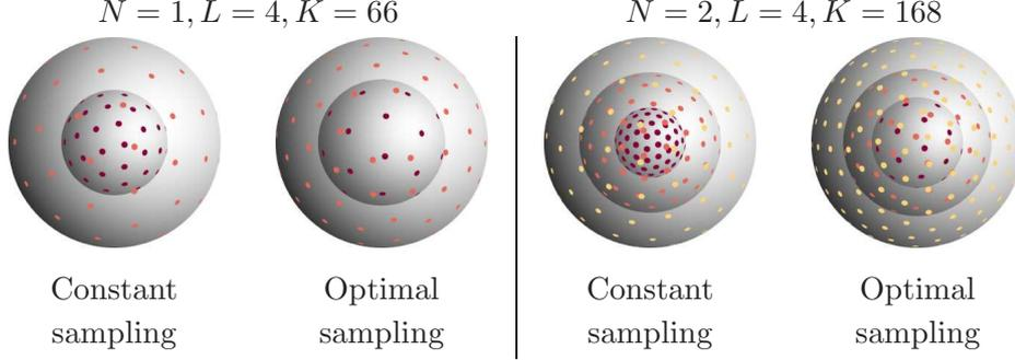
Figure 9.4: 2-shell (left) and 3-shell (right) acquisition protocols: regular multiple  $q$ -shell with constant number of points per shell, and optimal arrangement with minimal condition number for reconstruction in SPF basis.
