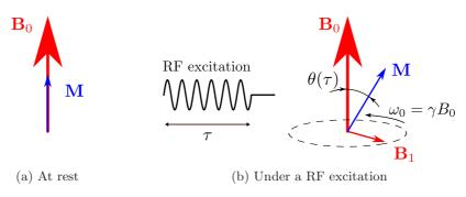
Figure 4.2: Net magnetization in presence of a strong magnetic field.
