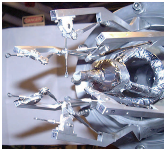
Figure 6.1: Picture of the target system of the eg2 run. The cryogenic target is in the back, enveloped in aluminum foils. The solid targets are held by mechanical arms allowing to change targets remotely, in the picture the top arm is in the beam line.
